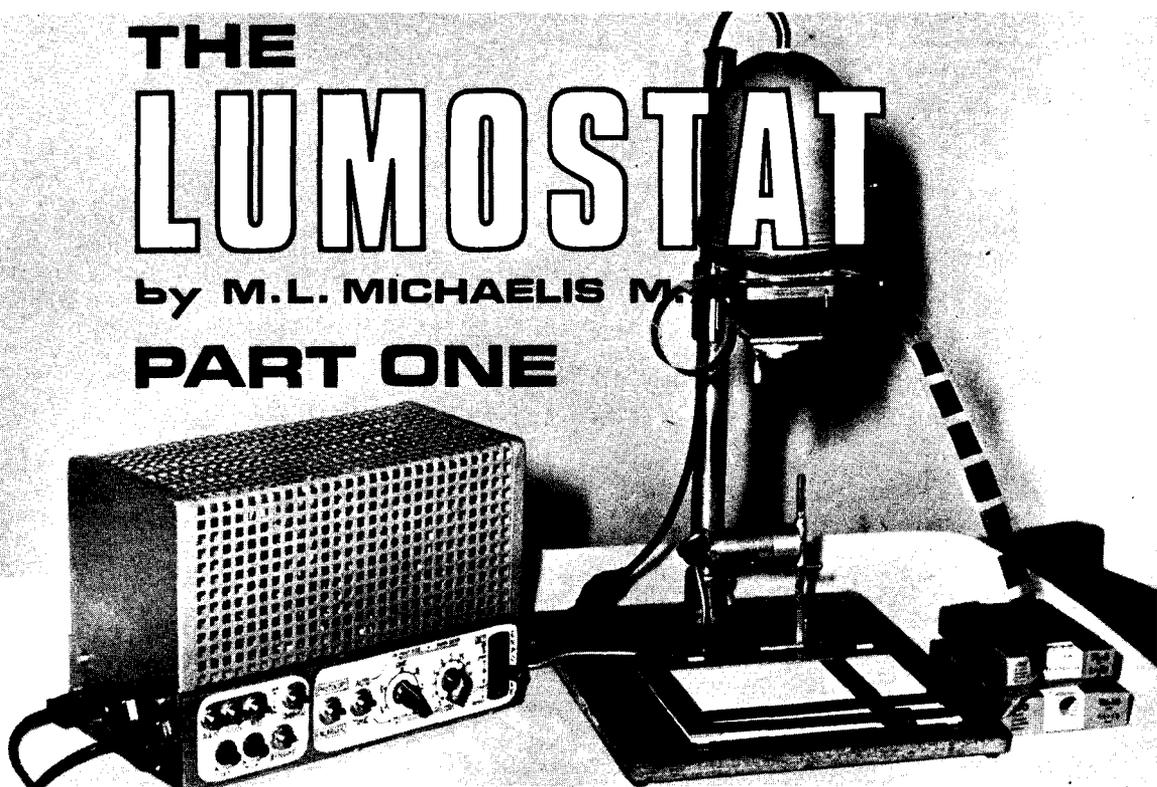
An automatic exposure control unit for the photographic darkroom. Suitable for both black/white and colour enlargements and prints, as well as for a wide variety of other imaging processes commonly encountered.
