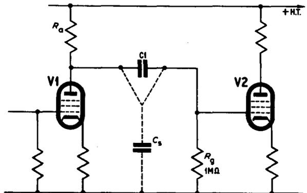
Fig. 1. Coupling components between two audio amplifier stages
