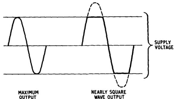
Fig. 6. The effect of boosting any frequency above specified maximum voltage causes distortion
