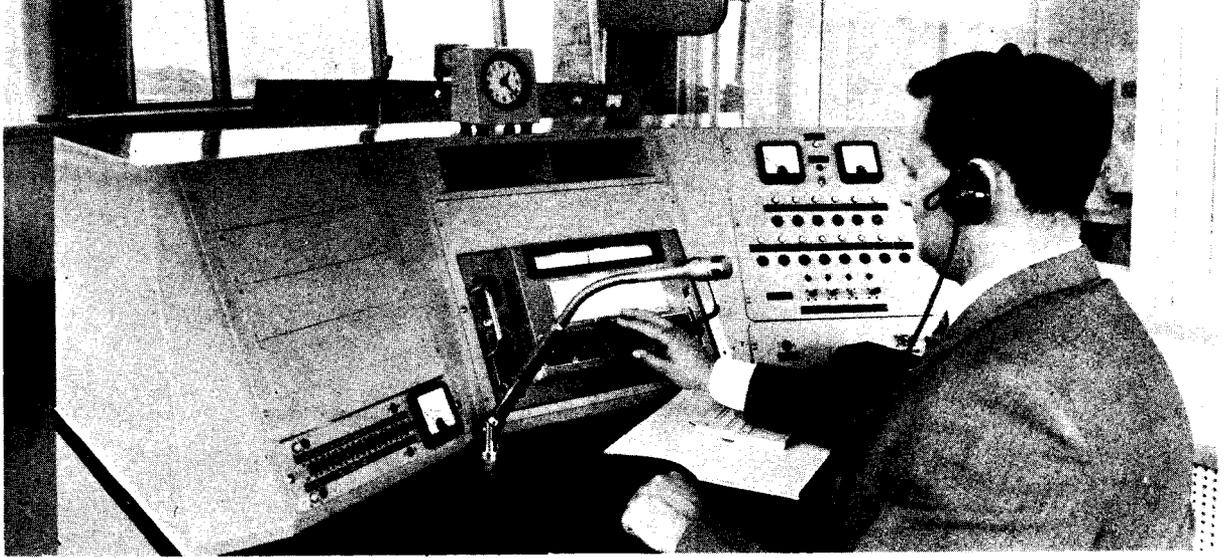
Fig. 7. Radio Officer's Remote Control Console at Anglesey Radio Station
