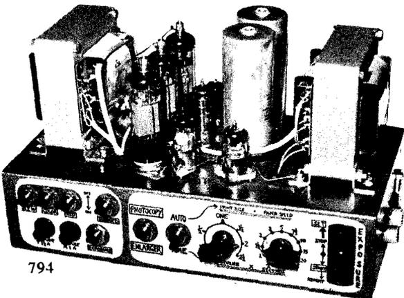
that this reduces the output ripple to negligible proportions even with the effective smoothing resistance of only 330 ohms presented by V1 to V3 at full load. The actual output ripple was measured to be 25mV with the lamp off and 50mV with the lamp on (full load). This does not change greatly if C2a,b are replaced by an ordinary 8 $\mu$ F capacitor, proving the point that most of the effective output capacitance results by electronic multiplication of C5.
