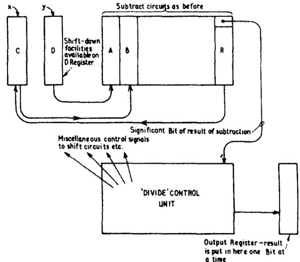
Fig. 6.2. The special registers C and D are required to hold both operands during the division process
