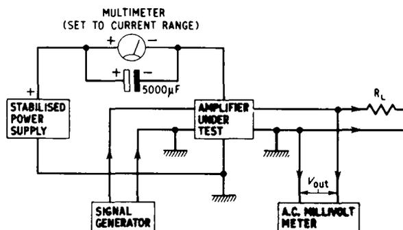
Fig. 2. Current drain measurement for maximum r.m.s. output
