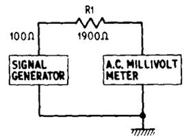
Fig. 4. Simulating the correct source resistance for the amplifier to measure the amplifier input voltage
