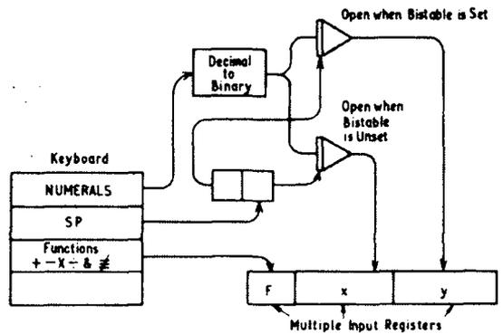
Fig. 6.5. Basic numerical input arrangement
