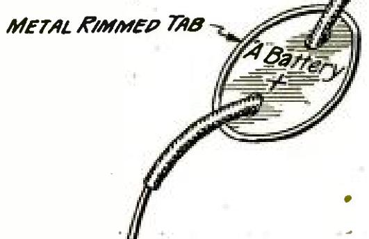
A MARKER FOR BATTERY WIRES
