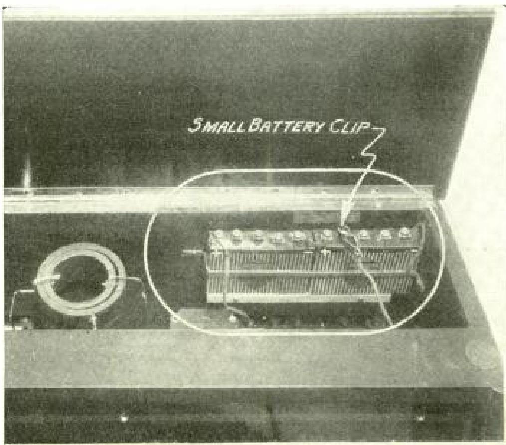
THE "C" BATTERIES INSTALLED IN THE CABINET
