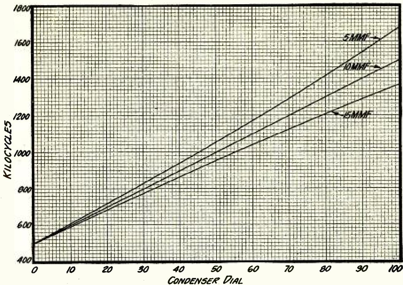
THE RESULT OF VARYING THE DISTRIBUTED CAPACITY OF THE COIL
