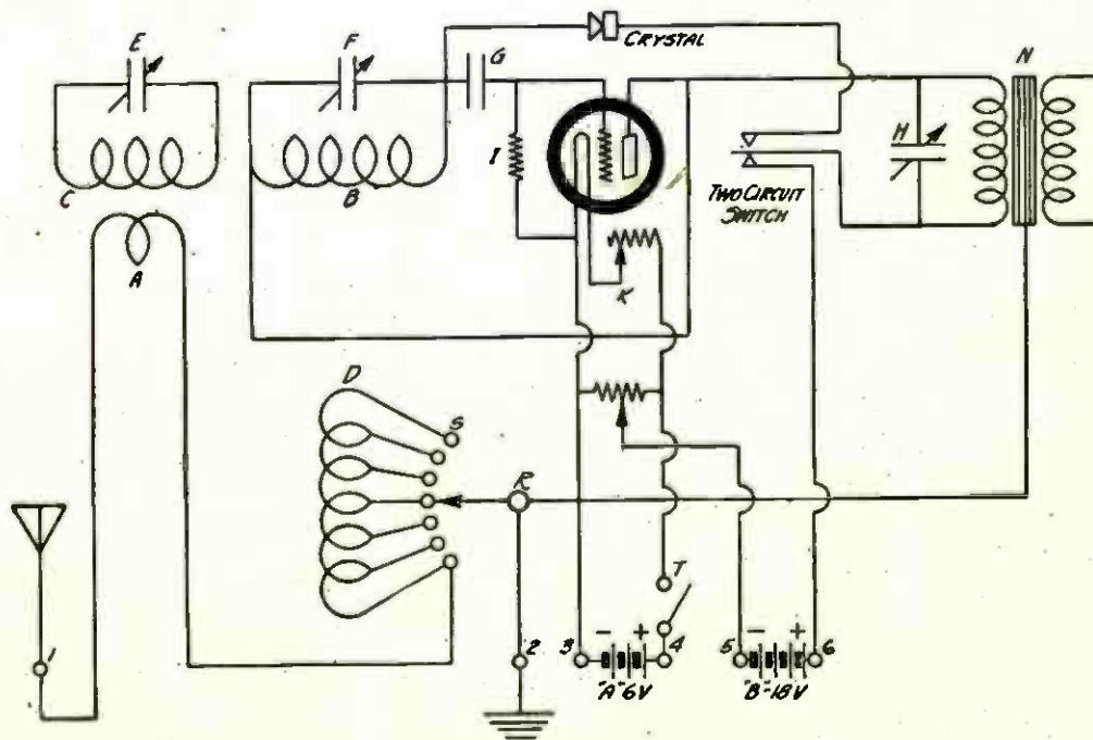
THE FOUR-CIRCUIT RECEIVER WITH A CRYSTAL DETECTOR
