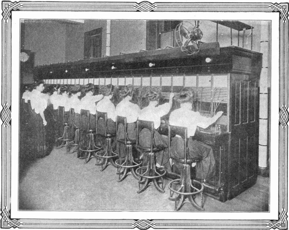
TYPE OF SWITCHBOARD TO WHICH SUBSCRIBERS' LINES ARE CONNECTED
