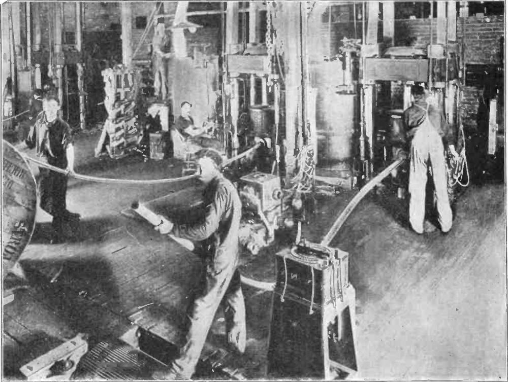
FIG. 4. FINISHED CABLE COMING OUT OF THE LEAD PASSES. THE LEAD JACKET IS SMOOTH AND CYLINDRICAL, WITHOUT A SEAM
