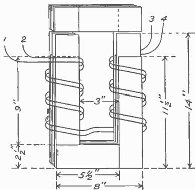
Connect No. 2 and 4 together for series connection and for parallel No. 1 & 2, And also 3 and 4.
