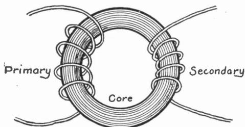
FIG. 91. SIMPLE TRANSFORMER WITH RING CORE
