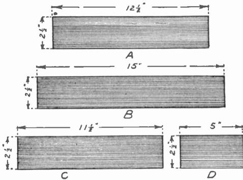
FIG. 95. STRIPS FORMING CORE
