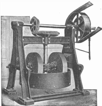
CRUSHING MACHINE FOR GRINDING UP THE CRYSTALS
