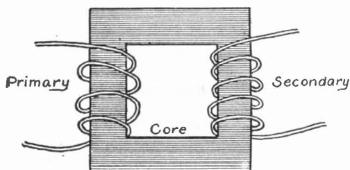
FIG. 92. SIMPLE TRANSFORMER WITH RECTANGULAR CORE
