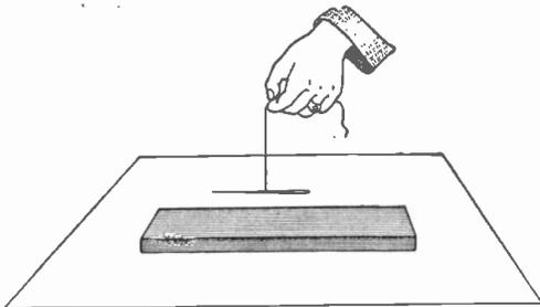
FIG. 108. DETERMINING THE DIRECTION OF MAGNETIC FIELD
