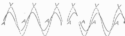
FIG. 93. ILLUSTRATING LEAD AND LAG IN PHASE
