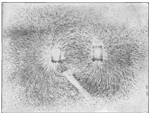
FIG. 111. PIECE OF IRON IN MAGNETIC FIELD
