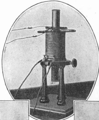
Fig. 1. Iron core with two coils
