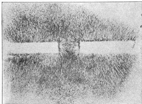
FIG. 113. ACTION BETWEEN LIKE POLES rather large diameter. Place in the bottom of this vessel a permanent bar magnet and
