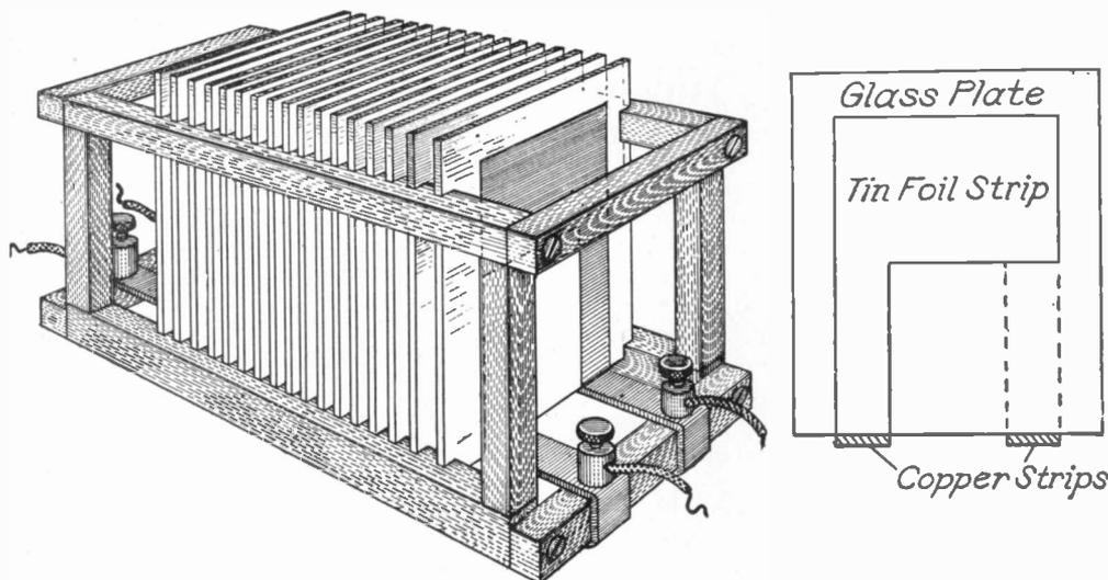
FIG. 2—CONDENSER FOR HIGH FREQUENCY APPARATUS
