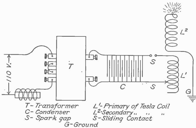
FIG. 3. CONNECTIONS OF TESLA OUTFIT
