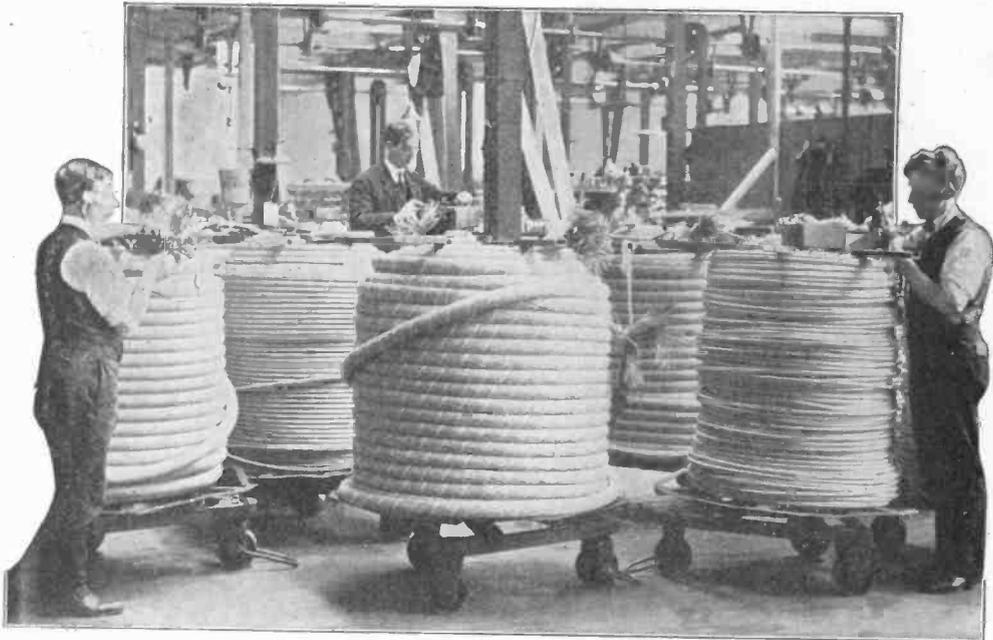
FIG. 2. TESTING CABLE CORES
