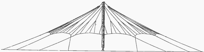
FIG. 3. ARRANGEMENT OF THE SIX FOLD UMBRELLA ANTENNA
