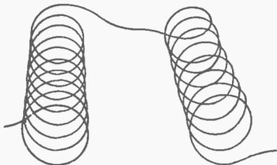
FIG. 134. THE WINDINGS MUST BE IN A CONTINUOUS DIRECTION
