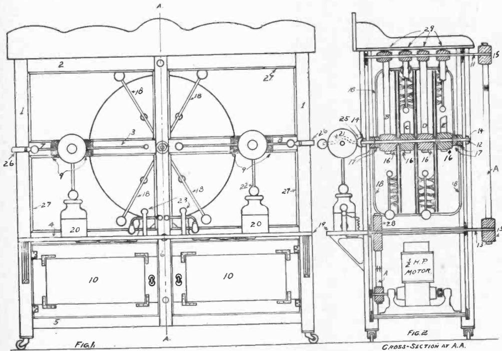
well seasoned hardwood. They should have an inch hole drilled exactly through the center and be fitted with a brass bushing which should fit the shaft very closely. The two center pulleys should be faced on each end, leaving a boss  $1\frac{1}{2}$  inch in diameter projecting 3-16 inch. The end pulleys have a similar boss on one end only. Great care must be taken to have the face true with the bore; otherwise the plates will not run true.
