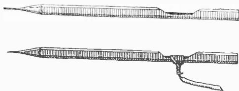
FIG. 1. LEAD PENCILS MAY BE USED FOR A MINIATURE ARC LAMP
