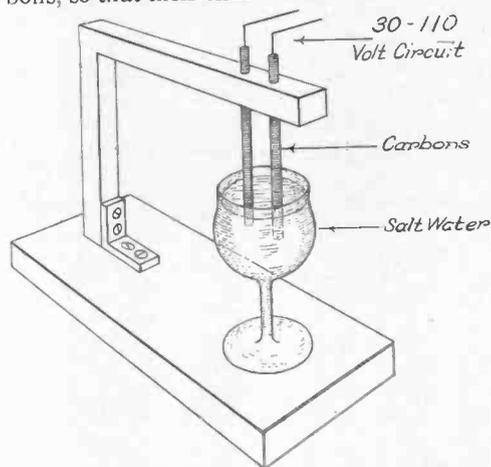
nect the carbons through a switch to the two sides of a 110-volt circuit and turn on the current. The more salt there is in the water the quicker it will boil. Be careful that the two carbons do not touch.
