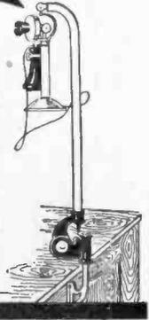
The *Radio* is simple in construction—strong, and has fewer parts than any other holder on the market. And any one can install it in five minutes. No disturbing of telephone cords or wiring necessary. Its suspension joint is ball-bearing, insuring ease of motion. All parts are malleable and non-breakable. Beautifully finished in fine enamel and oxidized copper.
