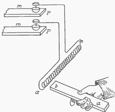
FIG. 135. A HOLLOW SOLENOID ACTS AS A MAGNET
