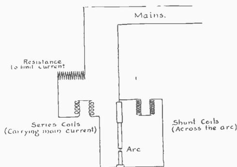
FIG. 4. CONNECTIONS OF AN ARC LAMP
