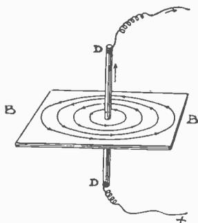
FIG. 41. ILLUSTRATING THE DIRECTION OF MAGNETIC FLUX
