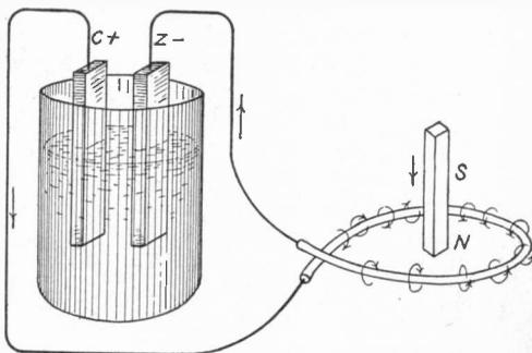
FIG. 131. MAGNETIZATION OF A BAR OF IRON BY CURRENT-CARRYING COIL
