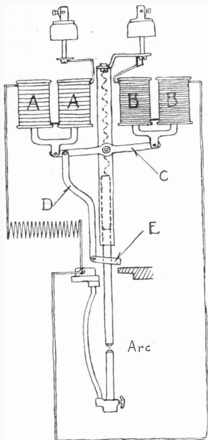
FIG. 3. THE VARIOUS ELEMENTS OF AN ARC LAMP
