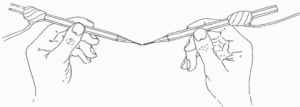
FIG. 2. HOLDING THEM BY THE WOOD, BRING THE TWO POINTS CAREFULLY INTO CONTACT
