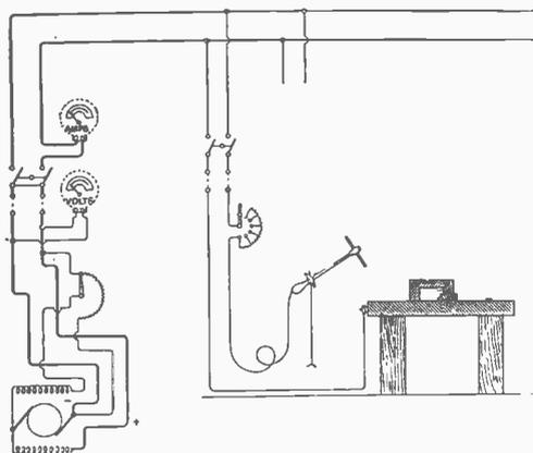
FIG. 2. ELECTRIC ARC WELDING EQUIPMENT
