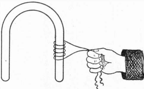
FIG. 132. STRENGTH OF MAGNETISM DEPENDS ON AMPERE-TURNS
