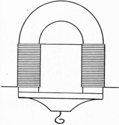
FIG. 136. HORSE-SHOE TYPE OF ELECTRO-MAGNET
