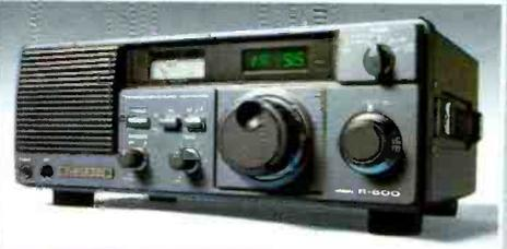
**R-600** General coverage receiver • 150 kHz - 30 MHz • digital display • 2 IF filters • PLL UP conversion • noise blanker • RF attenuator • front speaker • 100-240 VAC (Optional 13.8 VDC).
