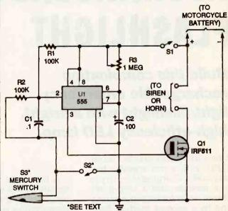
Fig. 4. Feel safer with this alarm circuit. When you're away, S3 makes sure no one touches your bike; when you're on it, S2 doubles as a panic switch.
