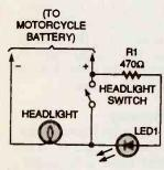
Fig. 1. With this simple circuit, you'll never again forget to turn your headlight on.
