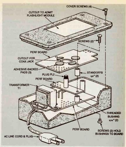
FIG 4—TRANSFORMER MODULE ASSEMBLY. A cutout in the cover admits the flashlight module. The upper board supports the flashlight when jack J1 is plugged into plug PL2 on the middle board. Transformer T1 is on the bottom board.
