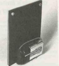
FIG. 7—THE 9-VOLT BATTERY and battery clip act as a stand.
