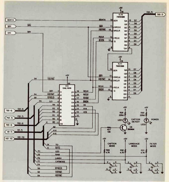
FIG. 5—THE DIGITAL DATA STREAM from the comparator is sent to a pair of serial-toparallel shift registers, IC10 and IC11. PAL IC9 asserts the RCLK signal that causes IC10 and IC11 to latch the data in the shift registers.
