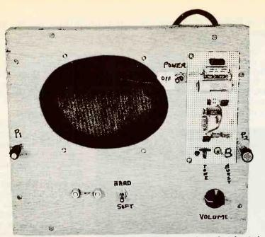
FIG. 3—THE AUTHOR MOUNTED THE COMPONENTS on a piece of perforated construction board and used point-to-point wiring. Everything was then installed in a home-made wood cabinet.
