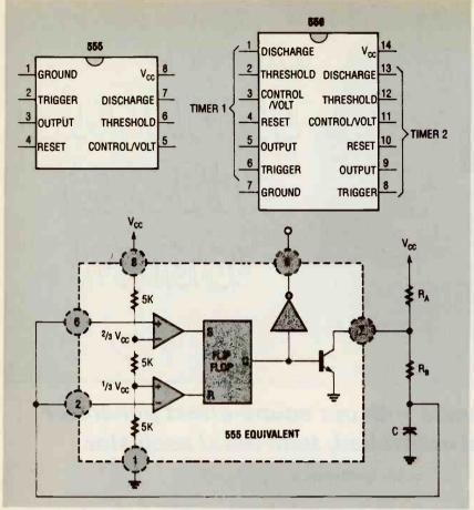
FIG. 1—PINOUTS OF THE 555 AND THE 556, and the equivalent circuit of the 555 timer.
