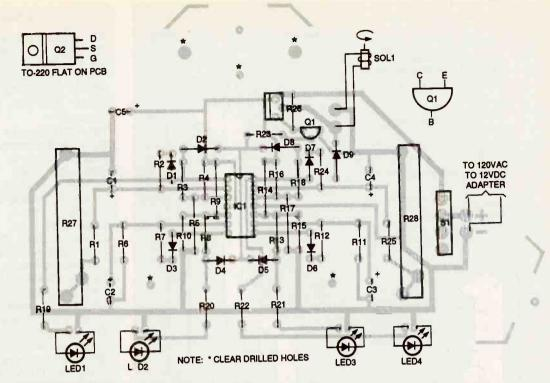
FIG. 4—PARTS PLACEMENT DIAGRAM for Bonker drive circuit. Bend the leads of MOSFET Q2 so it lies flat on circuit board.
