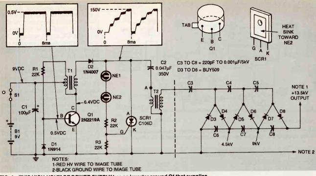
FIG. 4— THIS HIGH-VOLTAGE POWER SUPPLY has an inverter around Q1 that supplies 150-volt pulses to the converter of SCR1 and C2. The output of T2 is a 4.5 kilovolt pulse that is multiplied by the voltage-tripler network (right) to produce 13.5 kilovolts.
