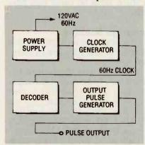
FIG. 1—MINUTE MARKER BLOCK DI-AGRAM. A 60-hertz square wave is generated from a 60-hertz signal, which is then used to decode desired time intervals. output, which is fed to the input IC1, a CD4040 12-stage binary counter.
