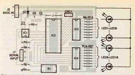
FIG. 3—PARTS-PLACEMENT DIAGRAM. Install sockets for IC1 and IC2, but don't insert the ICs into the sockets until tests are complete.
