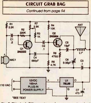
Fig. 7. This simple FM transmitter makes a great monitor circuit that can keep you out of harm's way.
