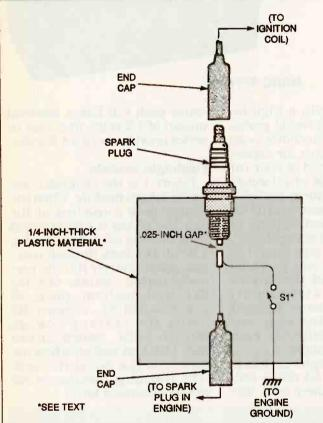
Fig. 3. Performing a tune-up on a newer bike is made a lot easier with this helpful circuit. Because of the high voltages present, make sure SI has an insulated handle and that the fixture is grounded.
