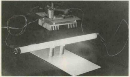
FIG. 5—THE FLUORESSCENT LAMP lights above the insulated metal plate.
