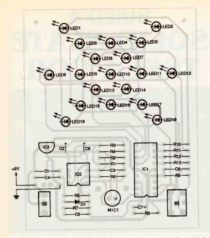
FIG. 5—PARTS-PLACEMENT DIAGRAM. Be sure to mount the LEDs flush with the board so that all cathodes face to the left.
