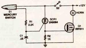
Fig. 3. Protect your bike with this simple alarm circuit.
