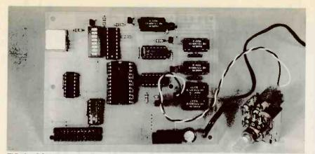
FIG. 6—COMPLETED RECEIVER board can be mounted in its own case or inside the device you want to control remotely.
