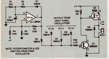
FIG. 2—A SIMPLIFIED SCHEMATIC to explain how the Bonker's solenoid drive circuit works.
