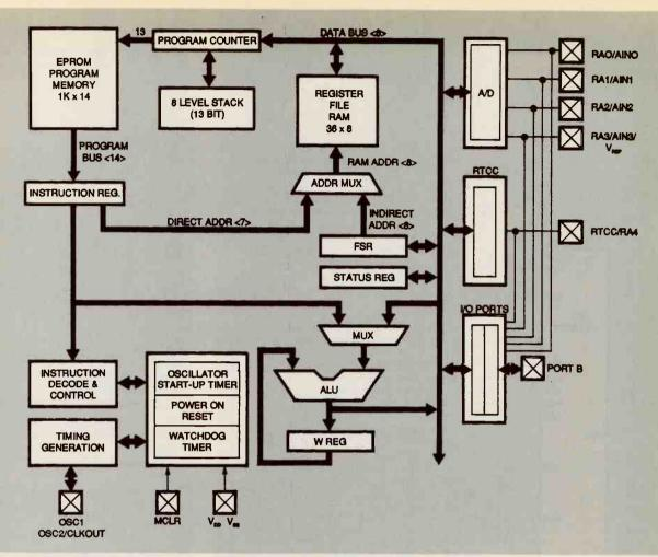
FIG. 2—PIC16C71 BLOCK DIAGRAM. The chip includes fully static CMOS circuitry, flexible I/O pin programming, timed interrupts, and a built-in eight-bit A/D converter.
