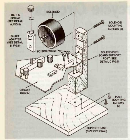
FIG. 6—ASSEMBLY DIAGRAM: The support base can be round or rectangular provided it is thick enouugh and has an area larger than about 30 square inches so it will be stable.
