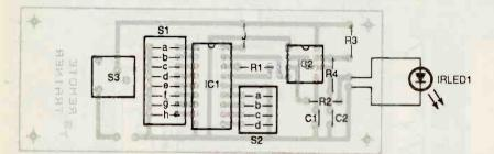
FIG. 4—TRANSMITTER PARTS-PLACEMENT. The small board makes a nice handheid unit.
