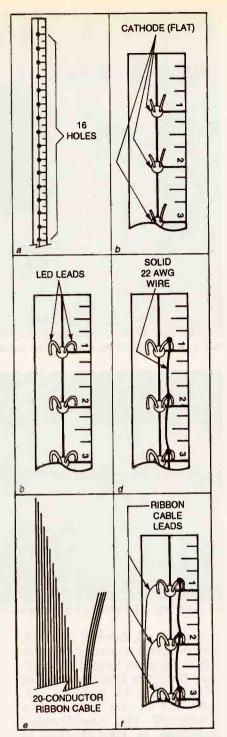
FIG. 6— HOW TO MAKE THE WAND. Drill 16 holes for the LEDs down the center of a wooden yardstick starting at the 1-inch mark (see text).
