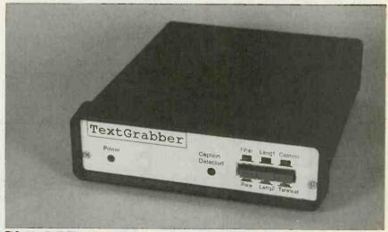
FIG. 10-THE TEXTGRABBER can be built in a compact cabinet.
