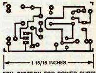
FOIL PATTERN FOR POWER SUPPLY circuit board.
