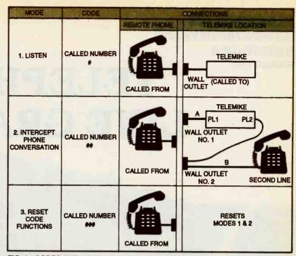
FIG. 1-CODES AND OPERATING MODE for the Telemike telephone line monitor.
