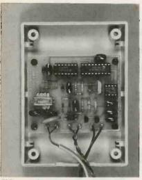
FIG. 4—MOUNT THE BOARD in the enclosure and cut two slots in the seam of the plastic case for the power cord and the phone cord.
