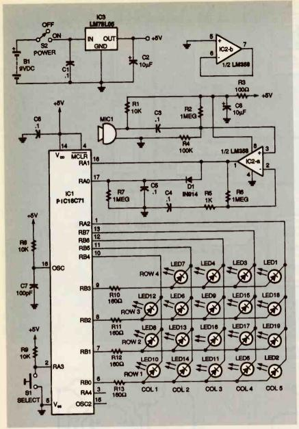
FIG. 1—MICRO-LIGHTS SCHEMATIC. At the heart of the circuit is Microchip Technology's PIC16C71 8-bit, CMOS microcontroller with built-in EPROM.
