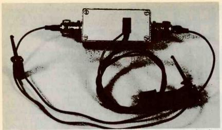
FIG. 3—COMPLETED FREQUENCY DOUBLER. The power leads are fitted with microclips and attached to two extra pins on the jumper block.
