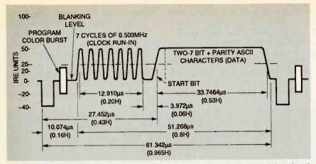
FIG. 1—CLOSED CAPTION DATA FORMAT. Captions are added to the television signal as serial bit streams that occur on line 21 of the odd field during the vertical blanking Interval (VBI).
