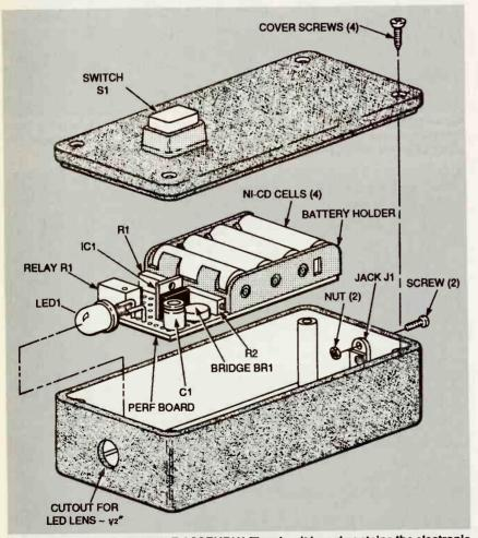
FIG. 3—FLASHLIGHT MODULE ASSEMBLY. The circuit board contains the electronic components and battery holder. The LED lens projects through a hole in the case. Jack J1 is at the other end of case, and switch S1 is on the cover.
