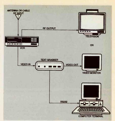
FIG. 9—TYPICAL TEXTGRABBER SETUP. The program being transcribed can be viewed either on a television connected to the VCR's RF pass-through, or on a video monitor connected to the TextGrabber's baseband video pass-through.
