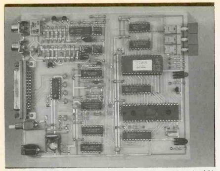
FIG. 8—FINISHED PC BOARD. This is an early prototype, so some of the parts might not be the same as those that you will be installing.
