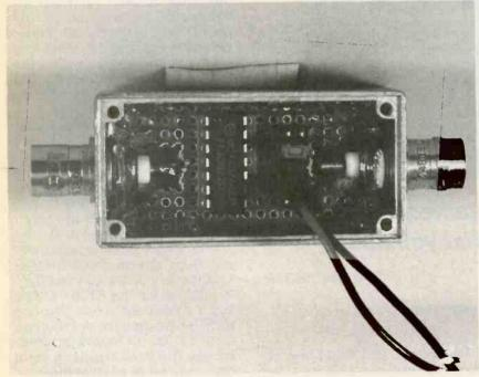
A JUMPER BLOCK was substituted for a triple-throw switch to conserve space.
