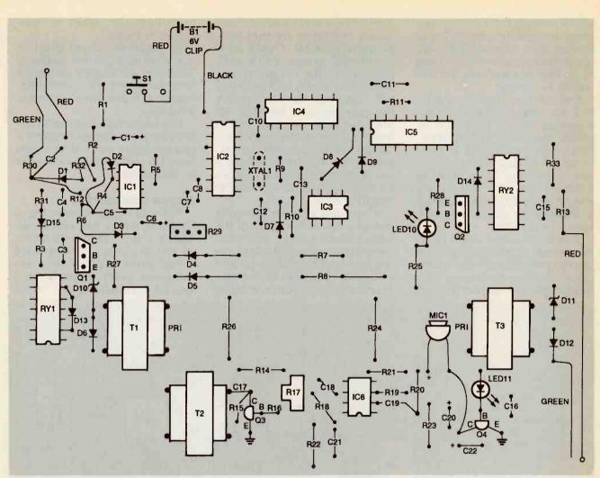
FIG. 3—PARTS PLACEMENT DIAGRAM. The entire circuit fits on a  $5\% \times 4$ -inch perforated circuit board. The components are interconnected by point-to-point wiring and power and ground bus wires. Switch S1 can be mounted off the board.
