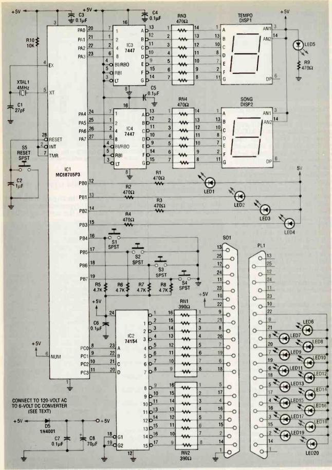
FIG. 2—SCHEMATIC FOR MICROCONTROLLER and indicator panel.
