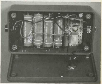
FLASHLIGHT MODULE with cover removed showing the four Ni-Cd cells, LED, and circuit components.
