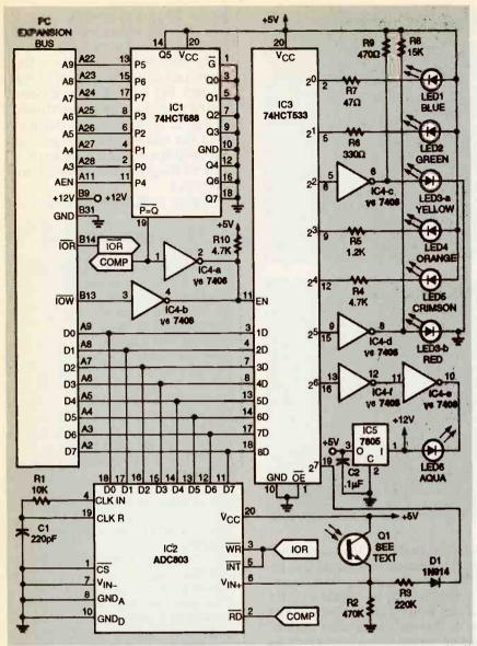
FIG. 1—COMPLETE SCHEMATIC. IC1 is an address decoder hard-wired to respond to I/ O ports 512–519. IC2 is an A-to-D converter that measures the voltage across R2, which depends on the amount of light shining on Q1. IC3 is an 8-bit inverting latch that the software drives to successively light each LED during a scan.
