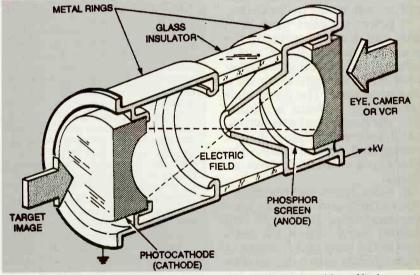
CUTAWAY VIEW OF SINGLE-STAGE image tube showing the position of its key parts.
