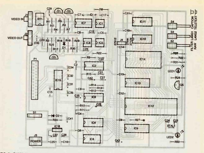
FIG. 7—PARTS PLACEMENT DIAGRAM. If you make your own double-sided board, solder all of the component leads on both sides of the board, and install a wire jumper in any through holes that don't have a component lead in them.
