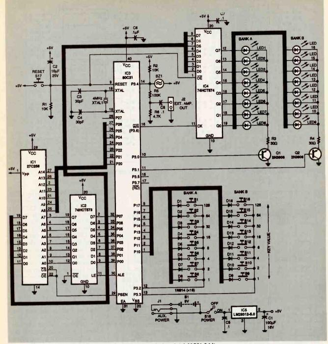
FIG. 1-C-GAME SCHEMATIC. The circuit is designed around an intel 80C31 8-bit microcontroller.
