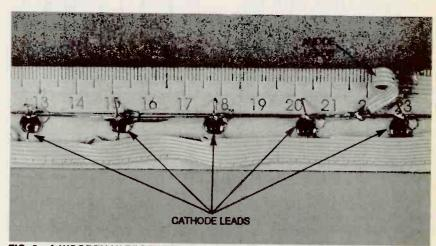
FIG. 8-A WOODEN YARDSTICK forms the body of the wand.
