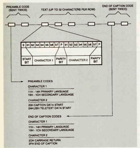
FIG. 2-VBI SERIAL DATA. Each "block" as shown represents a start bit and two seven-bit characters with parity.
