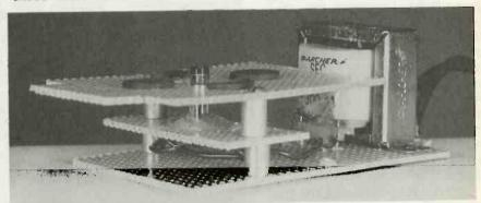
THREE-DECK ASSEMBLY in transformer module permits "docking" the flashlight module.
