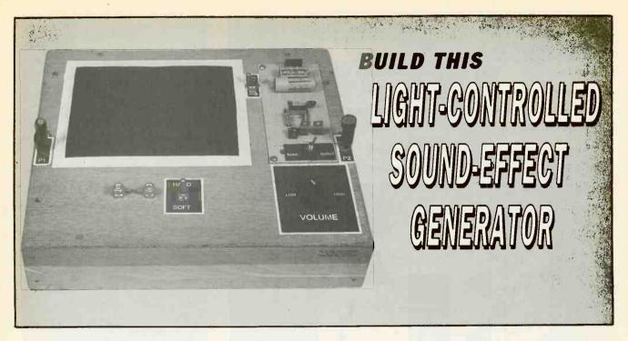
Generate weird sounds with our sound-effect generator based on a light-controlled, tone-burst oscillator.
