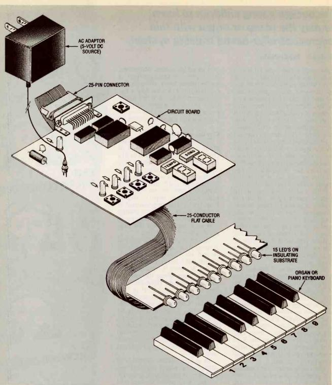
FIG. 1—MICRO-CONDUCTOR SYSTEM INCLUDES (top to bottom) outlet-mounted ACto-DC adaptor, circuit board with microcontroller, function displays and switches, and a fist-cable connected indicator panel that is placed above the right keys on the plano or crgan keyboard.
