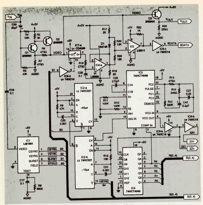
FIG. 4-VIDEO BUFFER AND PLL. Video is decoupled by capacitor C39 and then buffered by Q1 and Q2.
