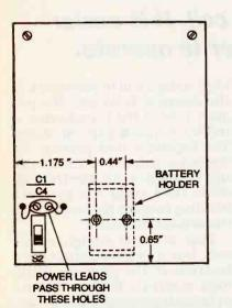
FIG. 6—DRILLING GUIDE. Four No. 2 screws and nuts hold the plastic backplate and battery holder in place.
