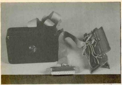
FIG. 2—THE PC INTERFACE CARD requires just enough space for five ICs, ten resistors, a couple of capacitors, and a diode. The reflectance probe contains six LEDs and the phototransistor cemented together with hot-melt glue and sealed in a light-tight box.
