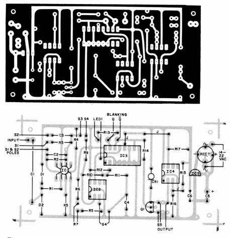
Fig. 2. An actual-size etching and drilling guide for a printed-circuit board is shown at top. Below it is guide for component placement.
