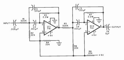
Fig. 1. Circuit for the Code Filter consists of cascaded pair of active stages formed by op amps IC1 and IC2.
