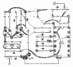
**Construction.** The circuit can be assembled on a small pc board using the foil pattern shown in Fig. 2. It can also be Wire-Wrapped using conventional techniques. Note that C5, C6, R9, R10, the neon lamp, and both transformers are not mounted on the board.
