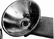
Final assembly of the author's prototype loing Alert is shown at left. Head assembly is mounted on piece of wood with the thermistor at the focal point.
