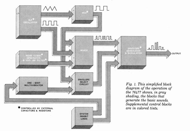
Desired sounds are all user defined. You simply switch into and out of the IC's circuit resistor and capacitor values and set a few logic states to "tailor" the audio parameter you require. Sounds of gunshots, explosions, sirens, musical instruments, "phaser" guns, etc., can be simulated. You can even create sounds you never heard before.
