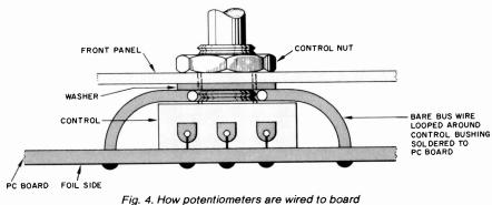
Fig. 4. How potentiometers are wired to board to provide support when mounted in case.
