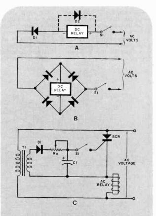
Fig. 6. Ac drive circuits: (A) single diode; (B) diode bridge; (C) thyristor.
