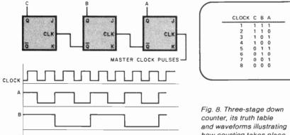
how counting takes place on the negative-going edge of the clock pulse.
