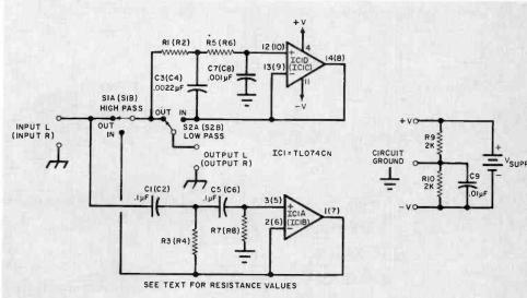
Fig. 2. Schematic diagram of the complete project.
