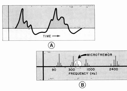
Fig. 1. Waveform of the human voice with microtremors is shown at (A), spectral content of voice is at (B).
