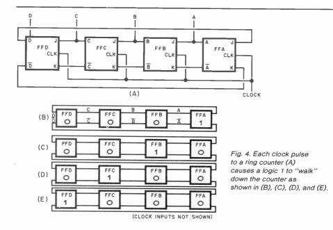
If both J and K equal 0, and a negative-going Clock pulse occurs, the Q output will remain unchanged. If J is equal to 1 and K equals 0 during the Clock edge, Q will become a logic 1 (set). When J equals 0 and K equals 1, a Clock pulse will force Q to equal 0 (reset). Finally, if J and K equal 1, the Clock will force Q to change its state or toggle. That is to say: if Q had been 0, it becomes 1 and if Q had been 1, it becomes 0.
