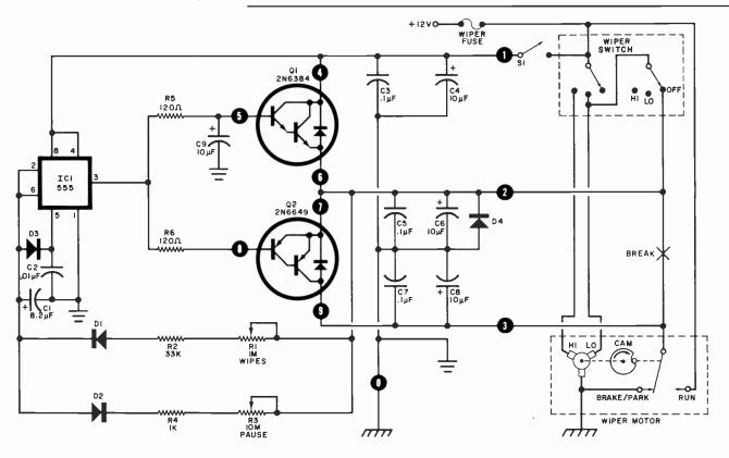
Fig. 2. The Auto-Wiper connects between the wiper switch and wiper motor after one lead is broken.
