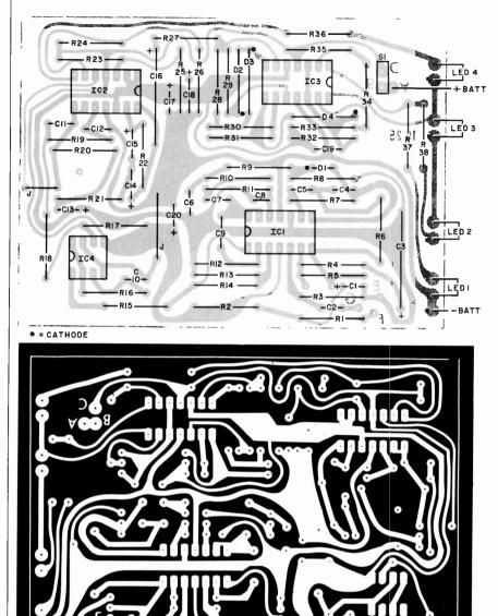
Fig. 6. Actual-size foil pattern and component placement guide for the voice analyzer. Be sure to observe polarities of electrolytic capacitors and diodes and orientation of ICs.
