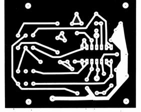
Fig. 3. Full-size etching and drilling guide for printed-circuit board is shown at left. Diagram for layout of components is above.
