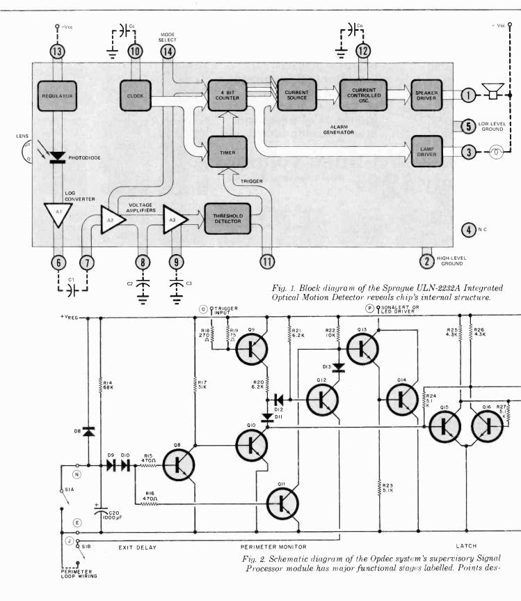
like a conventional optoelectronic alarm sensor (usually a CdS photocell) that triggers the alarm when the path between a light source and the sensor is interrupted, this novel IC senses the presence of an intruder by detecting changes in the amount of ambient light reaching it. As the intruder enters the
