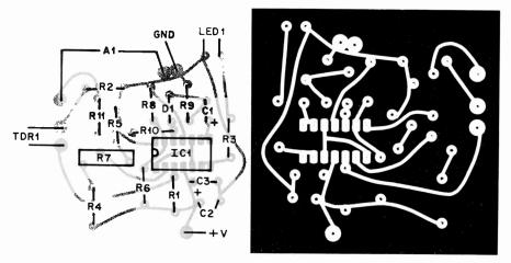
Fig. 5. Actual-size etching and drilling guide for a printed circuit board for the Infrared Road Icing Alert is shown above right. Component layout above left.
