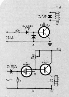
Fig. 5. Driver circuits with close differential operation: (A) single-stage transistor with zener; (B) two-stage FET and bipolar transistor.
