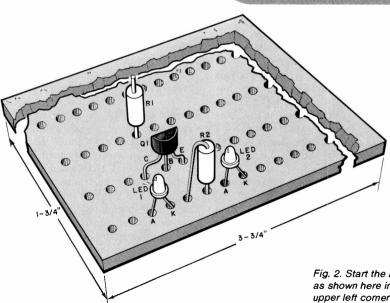
Fig. 2. Start the assembly as shown here in the upper left corner of board.
