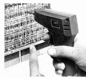
OK Machine & Tool BW-2630 motorized wrapping tool.
