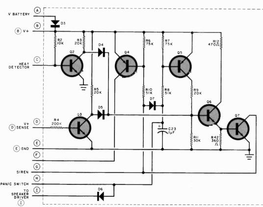
Fig. 7. Schematic diagram of Siren Driver module appears at left.
