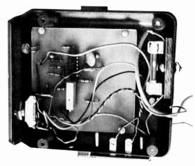
Since the temperature of the sensor is now approximately  $37^{\circ}F$  (the usual temperature that a refrigerator is set to), adjust *R7* until the LED just turns on. The system is now set up to sound off when the sensor "sees" a temperature below  $37^{\circ}F$ .
