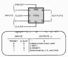
Fig. 2. Details of the 7476 flip-flop and its truth table.
