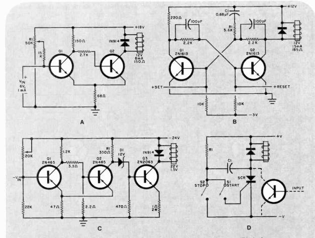
Fig. 3. Relay-driver regenerative amplifiers: (A) single-stage Schmitt trigger; (B) singlestage bistable; (C) Schmitt trigger with relay driver; (D) latching SCR control.
