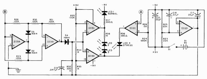
Fig. 5. The 8-to-12-Hz signals are rectified in IC3A and IC3B, integrated in C19 and used to turn on a comparator (IC3C, IC3D) that causes the LED (s) to glow. IC2C shuts down the LEDs when there is no 20-Hz signal, while IC2D creates a bipolar supply from a single 9-volt battery.
