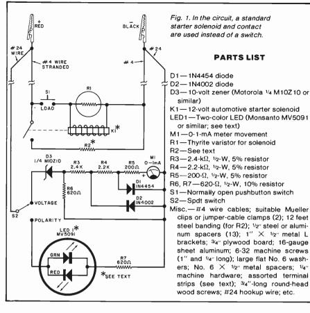
and diodes D1 and D2 make up a 0-to-6-volt dc voltmeter. When connected in series with 10-volt zener diode D3, this meter circuit becomes an expandedscale 10-to-16-volt dc voltmeter. Diode D2 protects the meter against reverse polarity, while diode D1 protects against overvoltage when the meter is connected in proper polarity.
