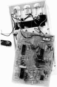
LEDs are positioned in window area, miniature microphone is put in center cutout at top of case.
