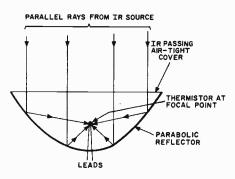
Fig. 2. A parabolic reflector focuses infrared rays onto the thermistor.
