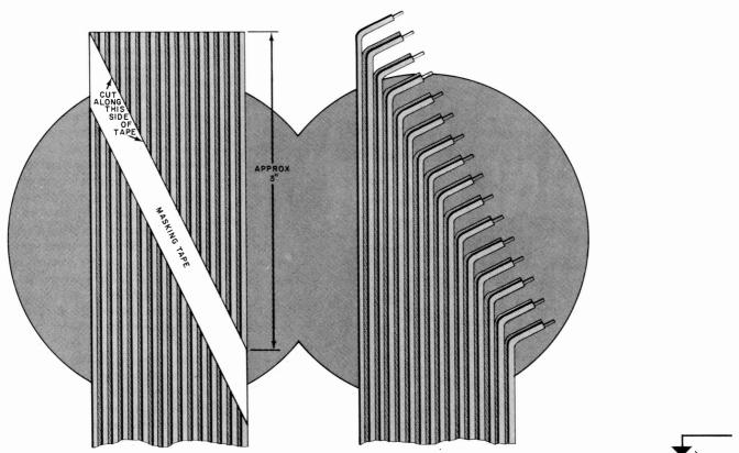
Fig. 3. The 16-lead ribbon cable is prepared as shown here with the leads cut diagonally so that they can be connected easily to circuits on the board.
