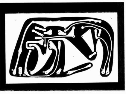
Fig. 6. Etching and drilling guide for the Siren Driver module's printed circuit board is shown above. Artwork for this and the other two pc boards on this page appears full-size.
