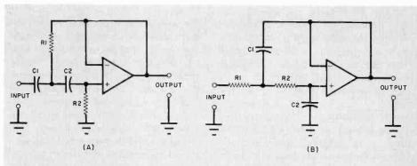
Fig. 1. Second-order high-pass (A) and low-pass (B) filters.
