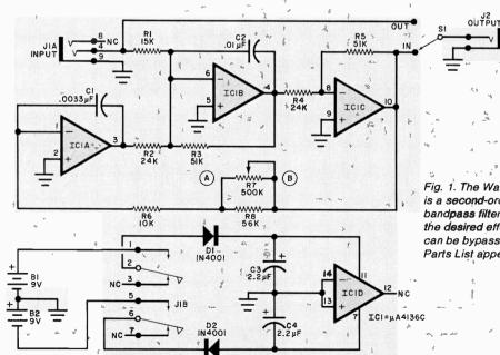
Fig. 1. The Wah-Wah Pedal circuit is a second-order, two-pole active bandpass filter that provides the desired effect. The filter can be bypassed by means of S1. Parts List appears on next page.
