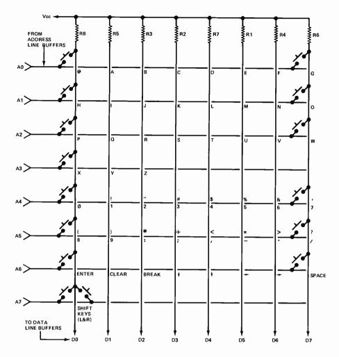
Schematic shows  $8 \times 8$  matrix layout of the TRS-80 keyboard, which is typical of boards of this type. A keyswitch is located at each intersection of the matrix to generate an output for a specific character.
