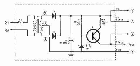
Fig. 3. This power supply can satisfy current demand of a complete Opdec system. Most of it fits on the Signal Processor's pc board.
