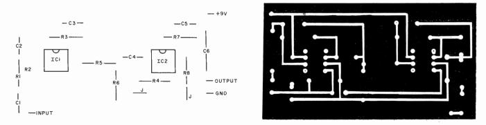
Fig. 2. Component placement guide for the Code Filter is shown at left, and actual-size pc board foil pattern is at right.
