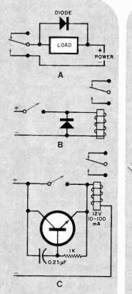
Fig. 1. Switchingtransient suppression: diode across inductive load (A) or relay coil (B); transistor circuit across switch contacts (C).
