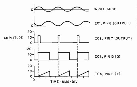
Fig. 3. Representative waveforms to be used in troubleshooting, with S1 on X1, S2 open, S3 on +, S4 on NORMAL, R7 three-quarters CCW and the timing capacitor selected for 1 ms/div.
