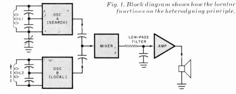
braid Faraday shield (more about the shield later) loses its effectiveness. A frequency of 650 kHz gives excellent sensitivity and offers convenience in final adjustment. As designed, the metal locator can detect a nickel in free air at a distance of 6" (152 mm) or buried at a depth of 3" (76 mm) or more.
