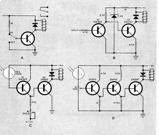
Fig. 2. Linear amplifiers as relay drivers: (A) single-stage; (B) two-stage inverting; (C) two-stage noninverting; (D) three-stage noninverting.
