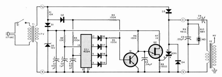
Fig. 1. Digital pulses from IC1 cause SCR1 to discharge C6 through primary of T2 to produce high voltage. Circled letters and symbol refer to foil pattern.
