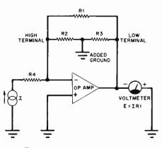
Fig. 4. An inverting op-amp circuit that can be used for in-circuit resistance measurements.
