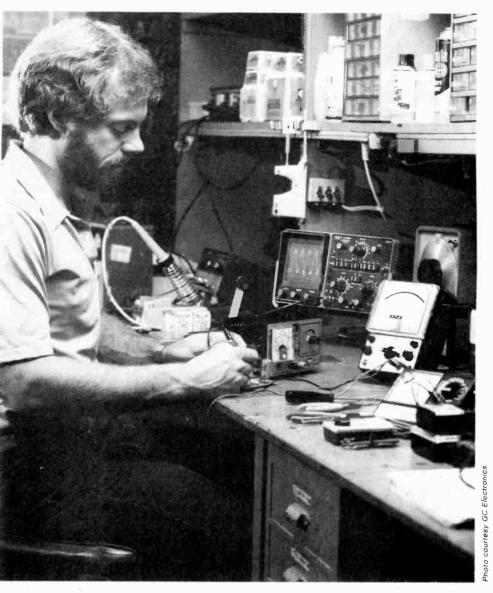
A well-planned electronics work area includes room for the project, test equipment, and storage. vent hand tools, hardware, and small components from rolling off the workbench and onto the floor.
