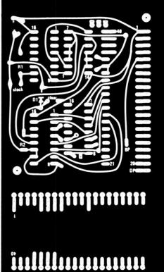
for some close work, so be sure to use a fine-tipped soldering pencil and smalldiameter solder. When soldering component leads to the board, apply the minimum amounts of heat and solder needed for good connections.
