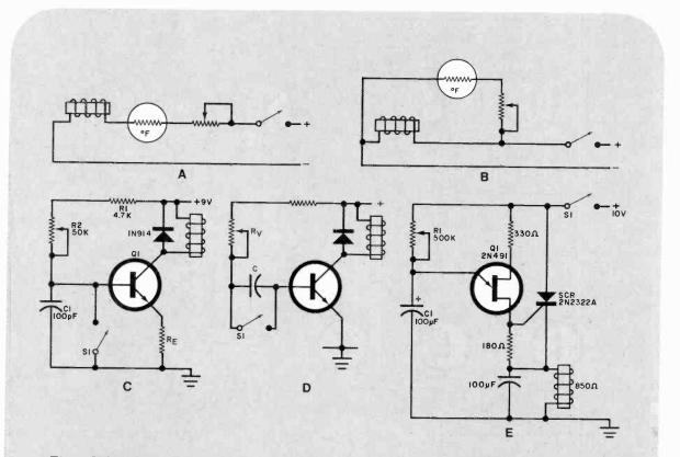
Fig. 4. Relay time-delay circuits: (A) thermistor-controlled slow-on/fast-aff; (B) thermistor fast-on/slow-off; (C) transistor-controlled slow-on/fast-aff; (D) transistor fast-on/slow-off; (E) unijunction transistor circuit with very slow on.
