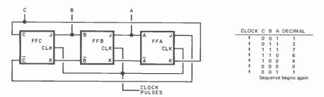
Fig. 6. Note the feedback from the last flip-flop to the first in a shift counter (left) with the truth table shown at right.
