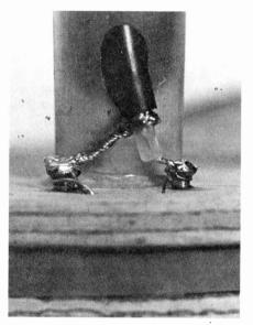
Fig. 10. Coax is routed to search coil through the shaft with ends soldered to the proper screws.
