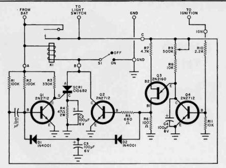
Fig. 1. The UJT turns off the lights by making Q2 appear as a momentary short circuit across SCR1. This causes the relay to open, removing power from lights and timer.
