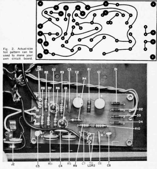
Fig. 3. After installing all components on board, make sure both trimmer potentiometers are accessible through holes drilled in side of chassis. This view also shows connections to other elements.
