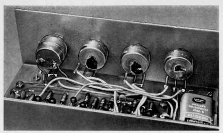
Fig. 3. All controls, except pots R28 and R29, are mounted on front panel. Battery holder and printed circuit board are mounted inside the chassis; use rubber feet on under side.
