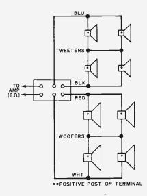
Fig. 5. Tweeters and woofers are wired in seriesparallel to present 8-ohm impedance to amplifier.
