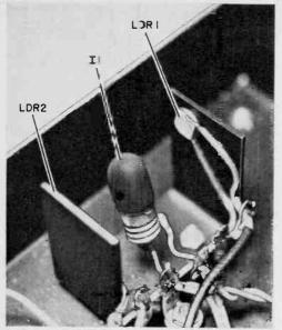
Lamp I1 is painted flat black and small dots of paint are removed on each side to shine on LDR's. Dot where paint was removed appears black here.
