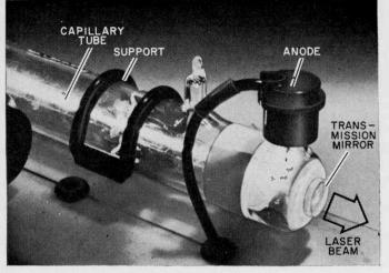
Close up of "business end" of the laser. Note use of rubber supports which secure laser in place. Make sure that exit optics are clean and laser is rigidly mounted on a chassis.
