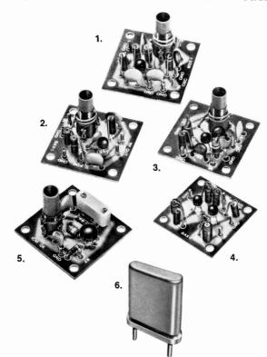
1. MXX-1 TRANSISTOR RF MIXER A single tuned circuit intended for signal conversion in the 3 to 170 MHz range. Harmonics of the OX oscillator are used for injection in the 60 to 170 MHz range. Lo Kit 3 to 20 MHz, Hi Kit 20 to 170 MHz (Specify when ordering)......\$3.50 ĩ
