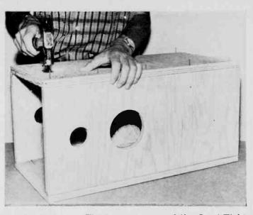
Fig. 2. Start construction of column by gluing and nailing together front, sides and rear. Note that speaker cutouts must all be in a common direction.
