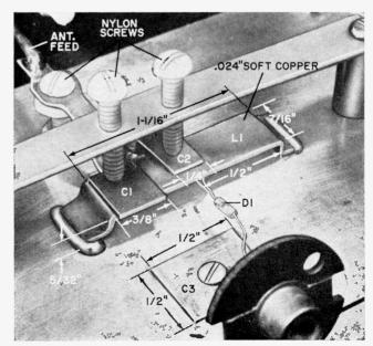
Fig. 7. Construction details of receiver. Strapline L1 is the same as used in the transmitter. Be sure to install mica insulators under capacitors C1, C2, and C3. Receiver uses the same antenna construction as that used with the transmitter.
