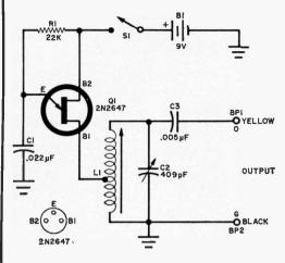
Fig. 1. Operating frequency is function of L1 and C1. Time constant of R1 and C2 allows Q1 to function as relaxation oscillator. R.f. output is taken off from BP1 and BP2.
