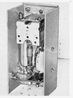
Orient C2 mounting bracket as shown at top, and use small L brackets for mounting circuit board.
