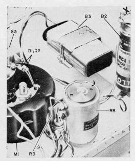
Standard potentiometer may be used for R8 instead of 10-turn unit. Diodes mount on meter terminals.
