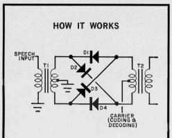
With no speech applied to the primary of T1, when the applied encoding carrier is positive going (with respect to ground), the currents in the primary of T2 and the secondary of T1 (through diodes D1 and D4) are out of phase so that no carrier signal is developed in the secondary of T2. When the encoding carrier is negative going, the same thing happens as the current flows through diodes D2 and D3. Thus none of the encoding carrier gets through output transformer T2.
