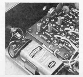
Battery can be conveniently mounted inside chassis with dual AA cell holder; use a conventional snap-on connector. Holes drilled directly in line with R28 and R29 (see top center of photo) provide access for tuning bass and woodblock oscillators. Mount output jack on rear.
