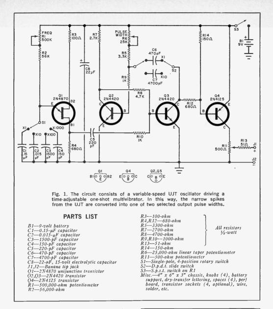
to increase the pulse width to more than 100 microseconds, the generator may start to divide the frequency. To insure stable operation, it is good practice to start with a narrow pulse width and then increase it as necessary.
