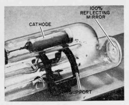
At cathode end of the laser tube, the mirror is 100% reflective to keep light from escaping there.
