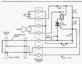
Fig. 1. Fence wires form closed loops and are resistively balanced with system. Imbalance due to short or open circuit will trigger alarm system.
