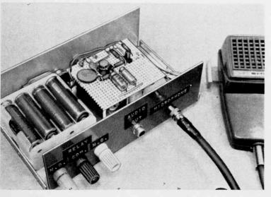
The three relay contacts – normally open, normally closed, and armature are terminated in three binding posts on the rear apron. These are connected as required by the external equipment being controlled, which can be either a tape recorder or transceiver.
