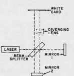
the white card. You can adjust the optics slightly to make both pairs visible. Further adjustment of the optics will cause one pair of dots to be superimposed on the other pair.
