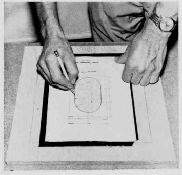
Fig. 3. Provided with crossover network is template that determines dimensions of cutout on bottom of enclosure. Use carbon paper to transfer dimensions to bottom plate. tionality. The ear can still identify the location of a multi-directional speaker due to the fact that direct sound reaches the ear before the reflected sound; but the placement of the column is less critical than that of conventional systems.
