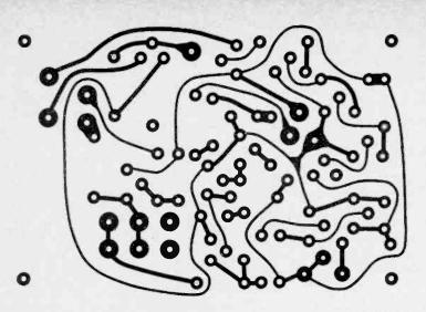
Fig. 2. Actual size foil pattern for the alarm. It can be easily duplicated with some reasonable care.
