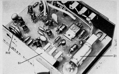
When mounting the PC board in the chassis make sure you can gain screwdriver access to R12 to that delay time can be adjusted as desired. If you have no need to vary this time, eliminate the hole.
