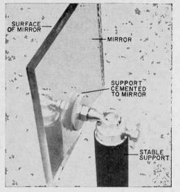
Fig. 3. Tripod support is removed and cemented to the rear surface of the front-surface mirror. Metal nut on tripod screw clamps the mirror tight.
