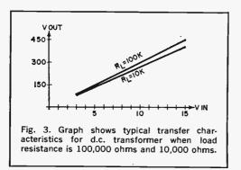
sembly from shorting out against the case. Besides providing insulation, the chart gives you a handy reference for the d.c. transformer's transfer characteristics.
