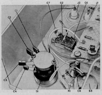
Fig. 3. Close-up view shows oscillator timing capacitors mounted on S1 and multivibrator capacitors mounted on S2. Perf board mounts on spacers.
