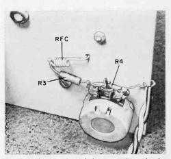
Fig. 4. Underside view of the transmitter showing the location of the RFC and R3. One end of the RFC feeds through a hole and contacts Q1 emitter.
