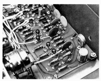
Bolt assembled circuit board to chassis via short spacers and #6 hardware. Note proper method of neatly dressing hookup wires.
