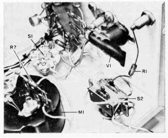
Switch S2 reverses the polarity of the ion chamber voltage. Resistor R1 is a safety resistor to reduce current flow in case of accidental short between cage and case.
