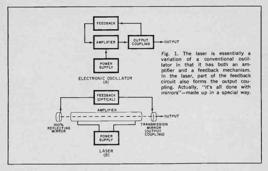
compare it with a conventional electronic r.f. oscillator—the principles of operation of the two are quite similar.
