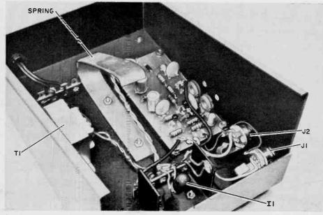
Interior view of the Waa-Waa showing the location of all parts. Note the two holes for the trimmer potentiometers. The lips on the chassis top limit the wooden foot pedal-at-the top of its travely
