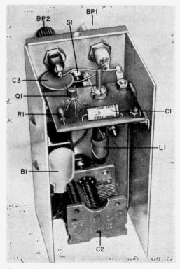
Fig. 4. Mount battery to side of box with length of aluminum stock,  $1_{\!/}''$  spacers, and #6 hardware.
