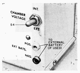
Switch S4 is used if it is desired to use a higher voltage for the ion chamber for more sensitivity.
