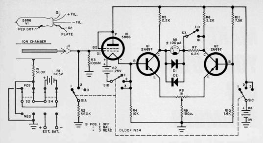
lons detected by the ion chamber develop a small voltage drop across the very high resistance of R3. This voltage is amplified and operates a transistorized bridge. Sensitivity depends on the value of R3 which must be extremely high to make the circuit effective.
