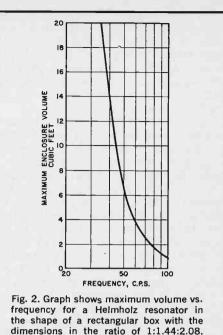
at Electro-Voice states that the optimum dimension ratio is 1: 1.44: 2.08 (see Fig. 2). In other words, a typical bookshelf enclosure might have an inside depth of 1 ft., an inside height of 1.44 ft. (about  $17\frac{1}{4}$ "), and a length of 2.08 ft. (about 25"). Or the 5 cu ft "universal" enclosure shown in Fig. 3 would have approximate inside dimensions as follows: A 30"; B 21"; C  $14\frac{1}{2}$ ".
