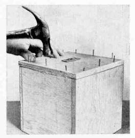
Fig. 5. Mount screw-type terminal strip to rear of cabinet; then glue and nail rear wall to cabinet shell, trueing up sides, top, and bottom as you go.
