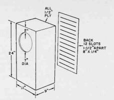
Fig. 4. Compact (1 cu ft) enclosure for 8" speakers has all sides lined with 1" absorbent material. Back is lined with soft cloth. Slots may be made by cutting strips of  $\frac{1}{2}$ " plywood to proper width and mounting them on a frame width  $\frac{1}{2}$ " spacing. Or cut a row of 10 holes  $\frac{1}{2}$ " in diameter to give about the same area as the 8" x  $\frac{1}{4}$ " slot.
