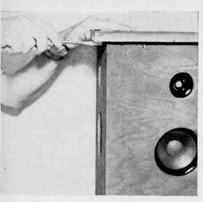
Fig. 6. Screws driven through column walls and into cleats secure top plate in place on enclosure.
