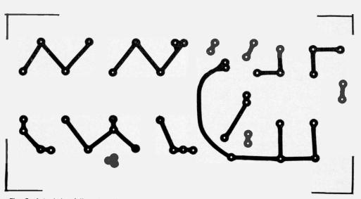
Fig. 3. Actual-size foil pattern for automatic start supply. Drill mounting holes at the four corners. 1971 Spring Edition
