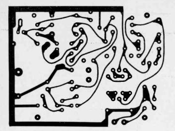
Fig. 2. Actual size foil pattern for the scrambler. This layout can be used only with subminiature transformers such as the Lafayette TR98 or similar types.
