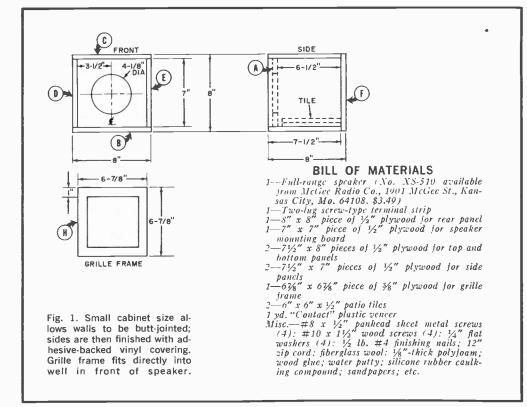
saw since small boxes do not require the same degree of bracing and careful joining of parts that are musts with large enclosures.
