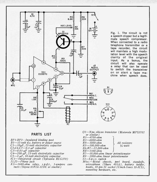
phone input J1, audio output J2, and the three relay contact binding posts are on the rear. As with any high-gain amplifier, leads should be kept short and direct to prevent feedback and high-frequency oscillations.
