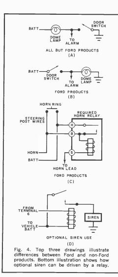
(ground). Connect the lead from terminal 5 to either side of the fuse that supplies the radio (or any other accessory that is powered only when the ignition key is in either the ignition or accessory position).
