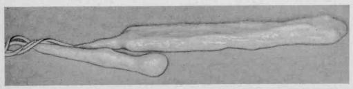
Fig. 2. Entire length of heater element and sensor, plus about 2" of connecting cables, must be thoroughly coated with epoxy potting compound to provide an airtight seal for the immersion elements.
