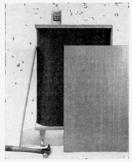
Once plywood end plates are secured to flue tile, glue and nail front and sides to the end plates.
