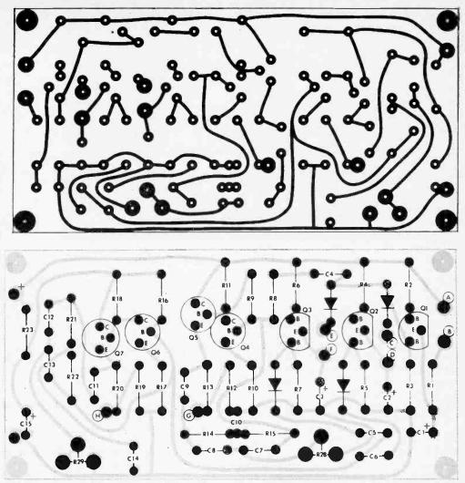
Fig. 2. Actual-size printed circuit board etching guide is shown at top. Directly above are component placement and orientation on circuit board after etching and drilling.
