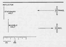
Fig. 8. Basic interferometer is used to measure frequency. As the movable half of the reflector is brought closer to the antennas, a series of "nulls" will be seen on the receiver meter. You measure the distance between nulls to determine frequency.
