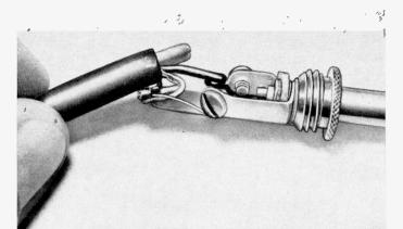
Fig. 5. When connecting plug to microphone cable, use only two shorter contacts. Do NOT allow cables to touch long one.
