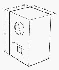
Fig. 3. "Universal" enclosure recommended by T. W. Richardson for "orphan" loudspeakers. Tune enclosure to 40 Hz. Use  $\frac{3}{4}$ " plywood, well braced, and glued and screwed together with glue blocks inside the corners. Volume should be at least 5 cu. ft. Typical values for A, B, and C would be 30", 21", and 14.5" respectively. If tuning equipment is not available, try 4 in. for E and  $\frac{3}{2}$  in. for F.
