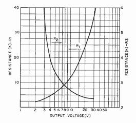
Fig. 2. Resistance values (in kilohms) for R1 and R2 in feedback circuit versus desired output volts.
