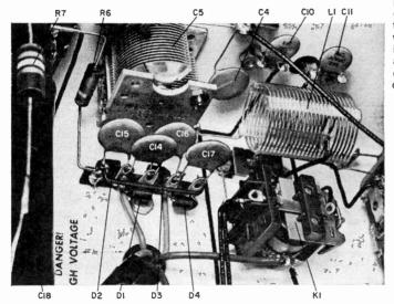
Fig. 4. Details of vacuum tube L-bracket (top) and rectifier and bypass capacitor mounting (bottom). The bracket is a narrow piece of scrap aluminum bent into an L-shape as shown with the vertical section about 11/3" long; mount the socket so that pin 4 faces the chassis. Also clearly shown in lower photo are the 4.36 screw and nut that prevents the rotor of C5 from opening fully to avoid accidental operation on 20 meters. Note method of "countersinking" L1's turns on both sides of tapped turn.
