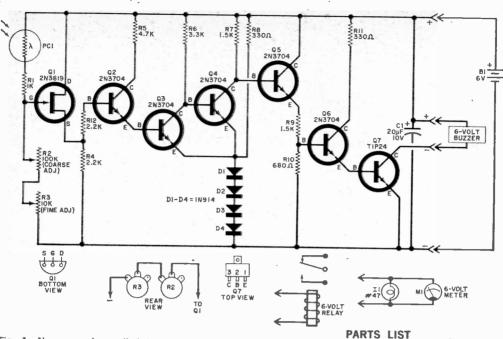
Fig. 1. No power is applied to output indicator until PC1 "sees" a predetermined level of infrared.
