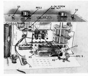
photos and called out in Fig. 2. Otherwise, the considerable amount of heat generated by V1 will be trapped within the chassis. Four rubber feet, at least  $\frac{1}{4}$ " thick, should be fastened to the bottom of the box so that it will clear the operating table sufficiently for air to circulate easily through 25 holes drilled in the bottom directly beneath the tube.
