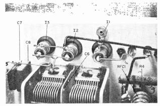
The three bulbs are press-fitted into ordinary rubber grommets. The crystal is mounted adjacent to 11. Note that 12 and 13 are connected in parallel.
