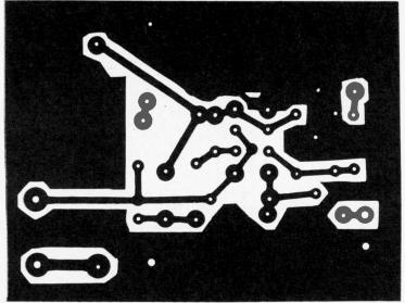
Fig. 2. Use this actual size layout for the PC board for the amplifier. Large amount of foil left on the board acts as an extra heat sink for ICI.
