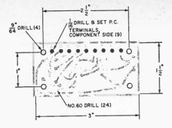
Fig. 2. Foil side of full-size PC board (right) is drilled as shown above and components mounted as shown in Fig. 3.
