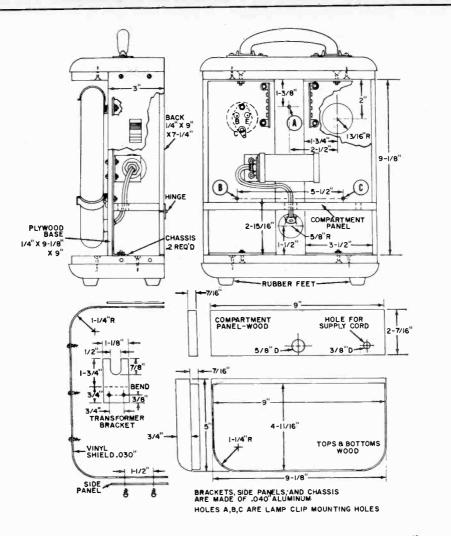
Fig. 2. If you want to duplicate the author's prototype, follow the construction details shown here. Note that the two transistors are mounted through the wooden front panel and the metal chassis. All wiring is done after components are mounted.
