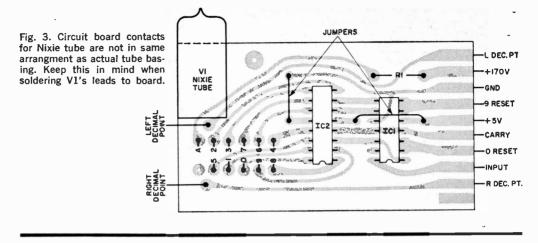
or used with a PC-board edge connector. After mounting and soldering IC1 in place, install the second jumper.
