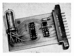
The jumper wire shown at center of photo should not be allowed to touch case or leads of decoder.
