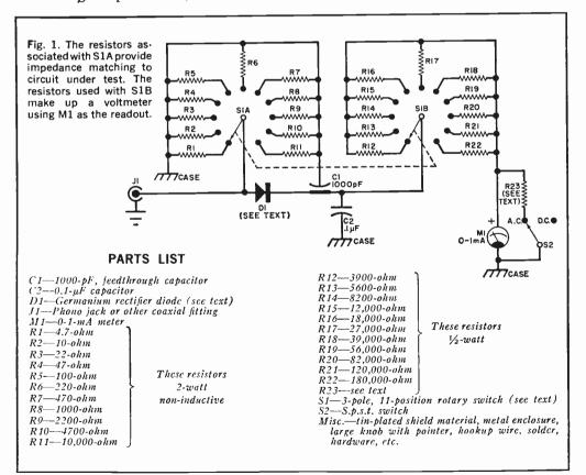
recalibrate the scale in accordance with Table I. When this is done, mount the meter in the case.
