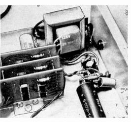
Fig. 5. Terminal strips and point-to-point wiring should be employed when assembling power supply.
