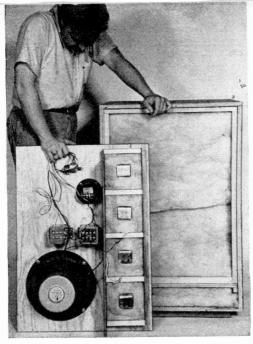
Fig. 3. For proper damping, loosely folded fiberglass wool should fill entire enclosure volume.
