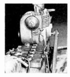
bracket provides belt adjustment. Overcharging is prevented by the car's voltage regulator. When not in use, the fan belt goes back in place and the mower engine stores neatly away in your car's trunk.
