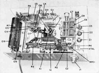
rig is tuned for maximum output as indicated by I2 and I3.
