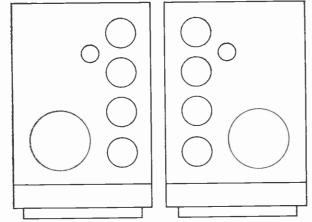
Fig. 4. Speaker mounting boards must be mirror images of each other for proper balancing of stereo.
