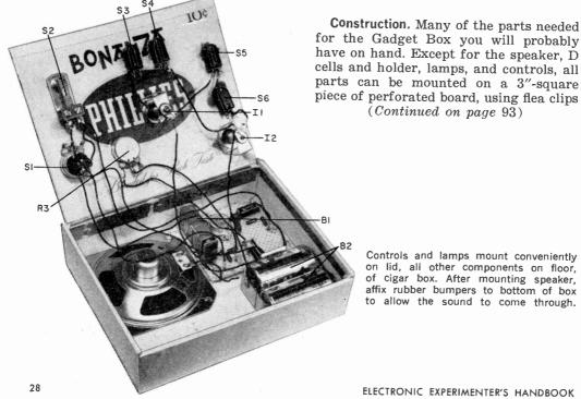
have on hand. Except for the speaker, D cells and holder, lamps, and controls, all
