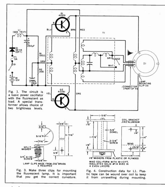
works from a conventional 12-volt d.c. car, boat, or trailer battery. It produces large-area illumination without harsh glare and has two levels of illumination —bright, or subdued for extra-low battery drain. Efficiency is high, thus getting the most from the battery, and generated heat is almost non-existent. You can attach the fluorescent light to the end of a 20-ft, conventional two-conductor rubber-covered appliance cord and position it where it is needed.
