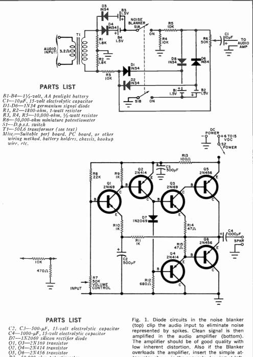
low inherent distortion, Also if the Blanker overloads the amplifier, insert the simple attenuator shown in the separate drawing at left.
