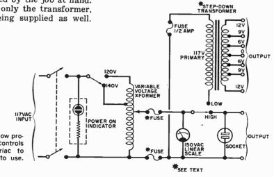
Circuit diagram shows how protective devices and controls are connected to Variac to give ease and variety to use.
