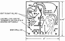
ONE REQ'D-MAKE FROM 1/16" SINGLE-SIDED FIBERGLASS PC MATERIAL
