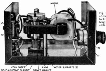
Fig. 2. View of inverted chassis shows driver magnet fixed to knob secured to motor shaft. Magnet must be as close as possible to non-magnetic frame top.
