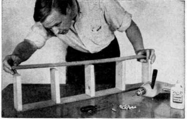
Start construction of midrange speaker enclosure by assembling sides, ends, and compartment separators. Use glue and screws to anchor the members together.
