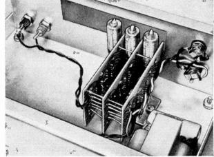
By mounting DCU's side by side so "common" holes line up with each other, assembly is simplified, and possibility of wiring errors is minimized.
