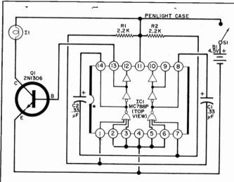
Fig. 1. The IC and associated components form a 2-kHz oscillator. This drives the transistor which in turn powers the flashlight lamp. In operation, the lamp flashes are so fast that the lamp appears to be turned on all of the time.
