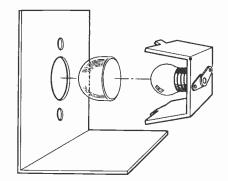
ceiver. Remove the #47 lamps, and replace them with #51 lamps. Then place colored dome-type lenses (for example, red for main tuning and green for bandspread) over the lamps, and replace the lamp holder on its bracket. —Gary Hummell
