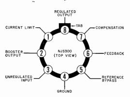
Fig. 1. Voltage-regulator pin arrangement. Components are added to provide for various load types.
