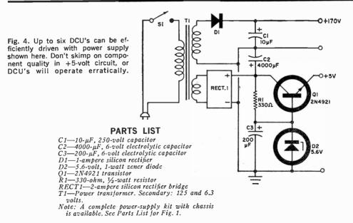
170 volts d.c. to drive the Nixie readout, and 5 volts d.c. for the IC's. The schematic of a power supply sufficient for six DCU's is shown in Fig. 4. If any other power supply is used, be sure that its outputs do not exceed 170 and 5 volts, since the Nixie tube and the IC's can be irreparably damaged by voltages that are too high.
