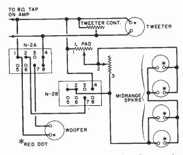
Fig. 2. To obtain proper phasing, be sure to wire all speakers together as shown here. Terminal numbers are stamped right on crossover networks. Tweeter control is supplied by the manufacturer.
