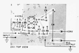
Fig. 3. Install the components as shown here. If you don't have a 16-ohm speaker, use two 8-ohm units in series. Be sure they are phased right.
