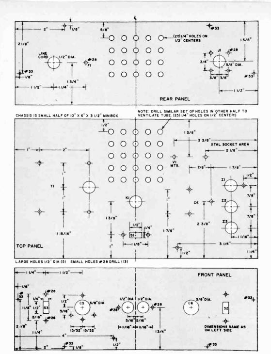
Fig. 2. Drilling specifications for the chassis. The three photos on the opposite page show the various holes and the location of all parts, Don't forget to drill 25 holes in the other half of the chassis, directly opposite the holes on the top panel. Crystal socket holes are drilled as required.
