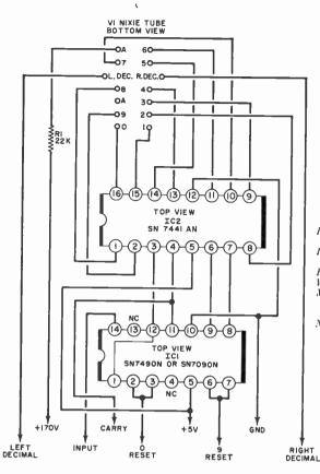
(TTL) is used; this gives the unit an operational speed of 18 MHz, twice that of the older circuit, which uses resistortransistor logic (RTL). Also, because TTL requires a much larger input trigger level, erratic indications due to line transients or other electrical noise have been almost eliminated.
