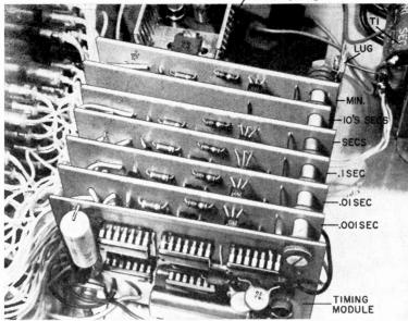
Fig. 9. Timing module and DCU circuit boards should be stacked for space conservation and neatness. Use 1/2"-long insulated spacers (or metal spacers and fiber washers) between each board for adequate separation. Board designations from bottom to top are M2 through M8.
