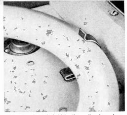
Fluorescent lamp is held by three clips (one shown here). Two of them are at same potential as the transistor collectors to aid fluorescent starting.
