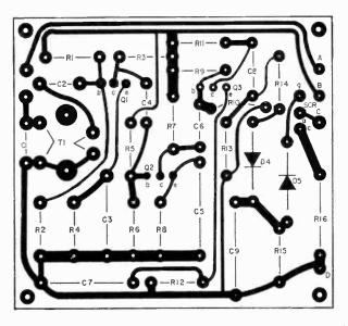
Fig. 6. Actual-size printed board for the demodulator. This also shows where the various components are to be installed on the finished circuit board.
