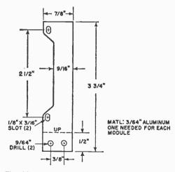
Fig. 11. If necessary, to avoid interference with components or wiring, deepen the notched cutout.
