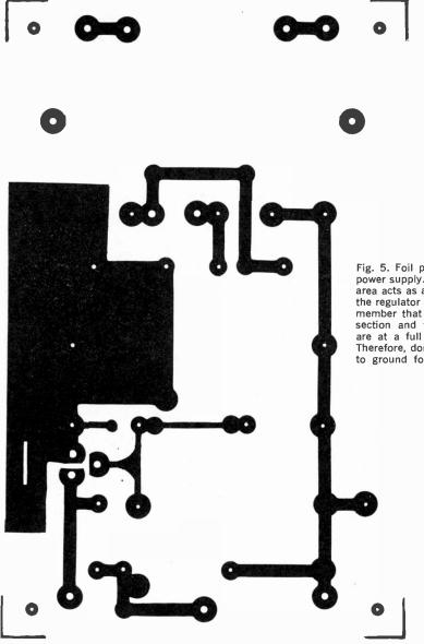
Fig. 5. Foil pattern for the power supply. The large foil area acts as a heat sink for the regulator transistor. Remember that both this foil section and the heat sink are at a full 24-volt level. Therefore, don't short them to ground for any reason.
