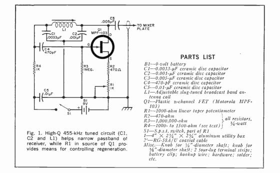
should be eliminated or at least considerably suppressed. So, the FET-QM is switched in, with the result that the passband narrows, and signal B is now to all means and purposes rejected. The FET-QM passes signal A and suppresses signal B, making the desired signal stand out.
