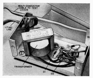
The transformer is mounted directly on the chassis with its secondary connected to the diodes mounted on terminal strip.
