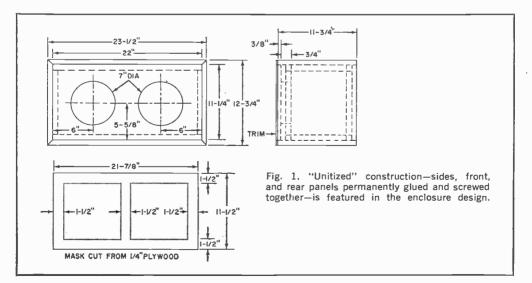
your workshop for making the beveled edges, be sure to adjust the sizes of the panels used so that the enclosure has the same inside dimensions called out in Fig. 1.
