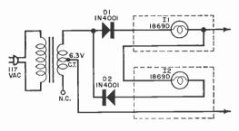
The lamps are connected so that, with equal potential on both probes, both lamps glow very dimly.
