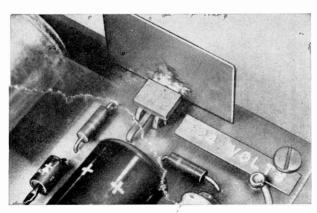
In the power supply, the copper heat sink is soldered to both transistor; tab and PC board foil.
