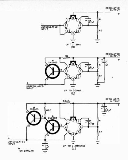
Fig. 3. Circuit at (a) provides a regulated output under 12 mA. Booster transistor is added in circuit (b) for output to 300 mA with smoothing capacitor. Second transistor (c) provides up to 2 A.
