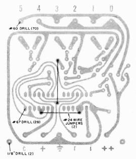
Fig. 3. Drill the PC board as shown here, and add the two insulated jumpers on component side of board.
