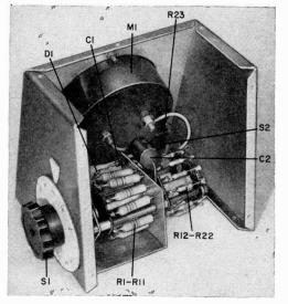
Mount the resistors, shield, C1, and D1 before installing the switch in the chassis. Grounding, through switch mounting hardware, must be tight!
