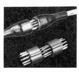
lengths of wire. Then solder the wires to the appropriate pins on the male connector. Finally, slip a 1" length of heat-shrinkable tubing over each connector, and shrink it in place.
