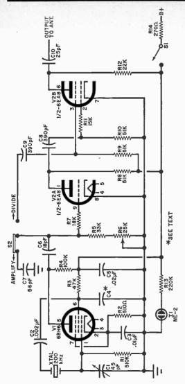
No tuned circuits are used, giving the crystal oscillator a harmonic-rich output. The second stage (V2) acts as a frequency divider controlled by R6.
