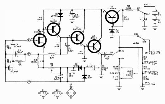
Fig. 1. The twin-T feedback oscillator incorporates both positive and negative feedback for stability and waveform purity. Frequency can be changed by replacing the twin-T filter.
