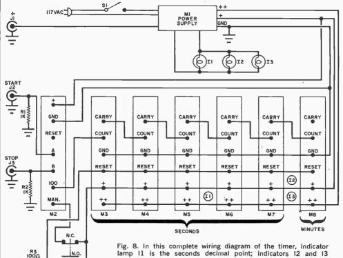
lamp 11 is the seconds decimal point; indicators 12 and 13 comprise colon that separates minutes from seconds readouts.
