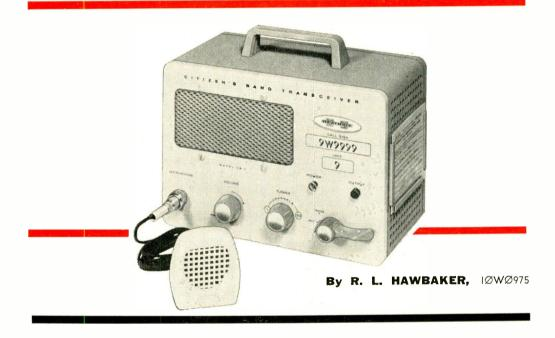
F YOU OWN one of the popular Heathkit CB-1 Citizens Band transceivers, here's a neat way to add an efficient squelch circuit to the receiver section. The squelch will block almost all of the "between-stations" superregenerative hiss and manmade noise—yet, if set properly, it will pass the weakest r.f. carrier. Installation involves adding only a few components and making some simple wiring changes.
