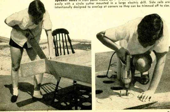
Speaker holes in front panel should be 4" in diameter and can be drilled most easily with a circle cutter mounted in a large electric drill. Side rails are
