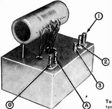
tion. The antenna is connected to terminal 1, and a jumper wire is connected from ter-
