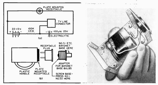
Very simple circuit at left may be mounted on a piece of Masonite as shown at right.
