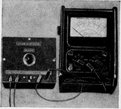
Front panel view of the lie detector. Any one of the readily available v.t.v.m. units may be used. The' common 1000 or 20,000 chms-per-volt meter will not permit efficient operation of the detector.
