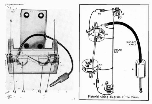
**Underchassis view** of mixer (above, left). Exact position of the two potentiometers is not critical. The author's potentiometers are equally spaced along one side with the input jacks at the ends. The cable to the recorder passes through a grommet in the side of the box. Use the proper plug for the tape recorder or amplifier at the end of this cable.
