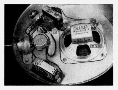
Interior view of banjo with various components identified and their relative positions indicated. The chassis is an aluminum cake pan, which contains the on-off switch SI.
