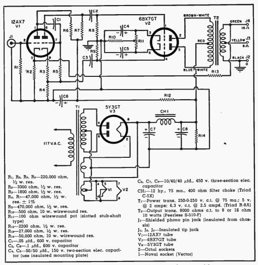
Fig. 3. Complete schematic of the 4-watt amplifier. It may be operated from most tuners and preamplifiers and provides adequate output for ordinary home listening.
