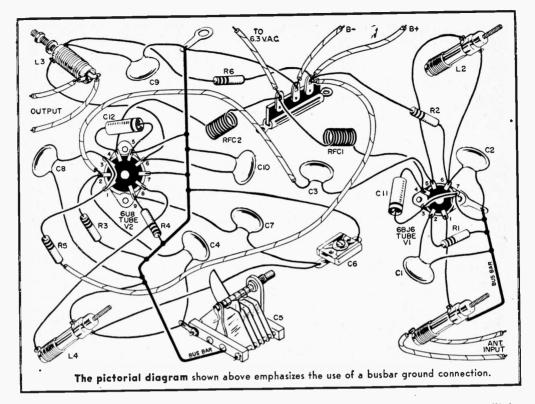
and L3 to 4000 kc. Apply voltage to the tuner and check with the grid dip oscillator to see that the oscillator circuit is oscillating at 45 mc. Final tuning can be completed on received signals.
