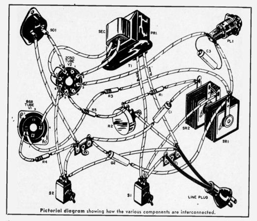
the output socket; the primary flash will now fire the slave lamps instantaneously. Once a photo is taken, flip *S2* to the down position at once before inserting flash bulbs for the next round.
