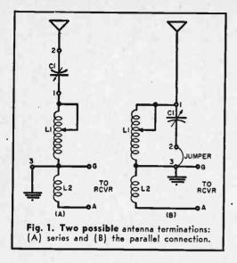
minal 2 to terminal 3. 'The coil, variable capacitor, and antenna-to-ground capacity are now in parallel. This connection is most frequently used when antenna impedance is high. Antennas that are very short will probably require such a parallel connection.
