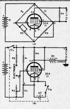
Above. Fig. 1. Schematic diagram and parts list of home-built lie detector. (A) is a simplified diagram of (B) indicating the resistance bridge.
