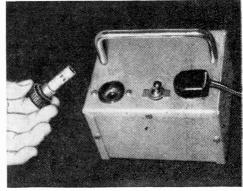
Weighing less than 21/2 pounds, the first unit is housed in a 3" x 4" x 5" utility box. Fuse holder is modified to take the 11/2-volt penlite cell as shown in Fig. 3 on page 76. Placing the handle off-center makes for proper mechanical balance.
