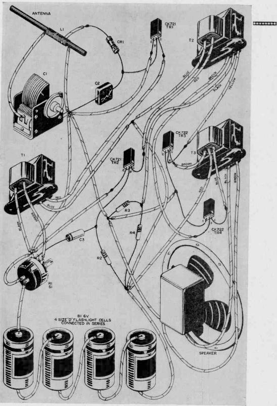
**Pictorial diagram** (on opposite page) and parts list (below) for the complete transistorized receiver.
