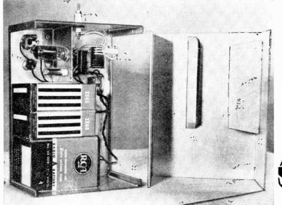
**Back view** of the R/C transmitter showing the position of the batteries, the subchassis bolted in place, and the position of the antenna loading coil, L4 above the tank coil.
