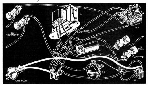
Fig. 4. Pictorial diagram of the alarm.
