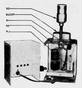
**Rear view** of control unit with cover removed. Note the subchassis on which the tube and relay are mounted. Holes in back and top are for ventilation.
