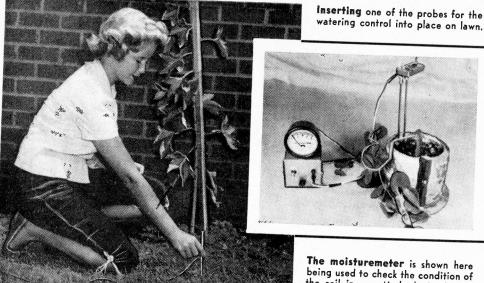
being used to check the condition of the soil in a potted plant. It can also be used to check moisture in a lawn or garden soil, after calibration.
