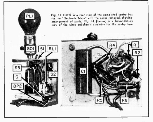
minum subchassis, with most of the circuit wiring completed before the subchassis is mounted in the cabinet. Above- and belowchassis views of the wired subchassis are given in Figs. 13 and 14 respectively.
