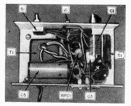
Fig. 5. Bottom view of the Hart-25 chassis. Most of the major components are visible, except the socket for VI, the 6W6GT, which is hidden by the variable tuning capacitor, CI.
