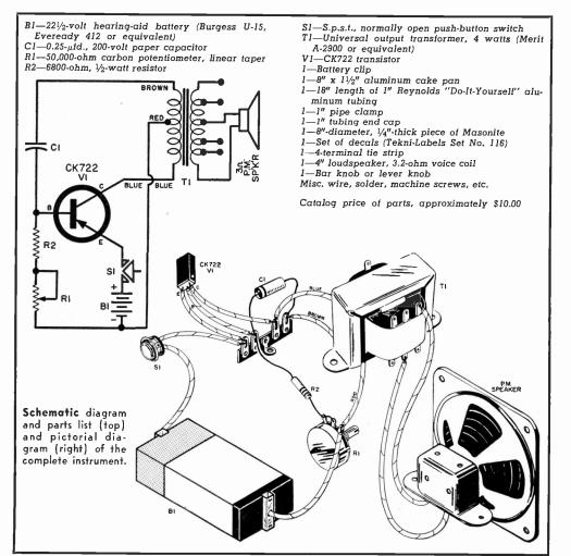
base circuits to start and sustain oscillation. The "common emitter" circuit is employed and is roughly analogous to a vacuum-tube circuit in which the emitter (E) acts as cathode, the base (B) as grid and the collector (C) as plate.
