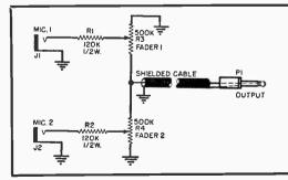
*R*<sub>4</sub>. Audio level obtained from each microphone now depends upon the settings of R3 and R4. Either of the two inputs may be emphasized, both may be turned "off," or both may be turned to full volume, depending on how the controls are set. The combined signals are led into the "mike input" jack of the recorder or amplifier.
