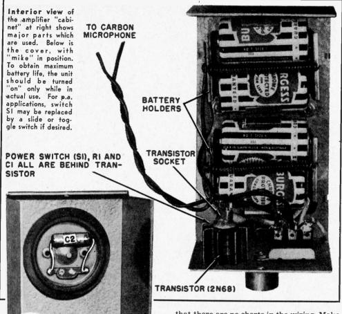
2N68. If desired, *n*-*p*-*n* junction type 2N102 may be used in place of the 2N68, provided the battery polarity is reversed as well as the leads to capacitor C1.
