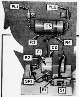
Fig. 1 (above). Rear view of "Winking Clown" with protective cover removed and the various components identified.
