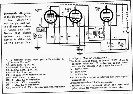
trol are mounted on the front of the cabinet and the other parts on a metal chassis. Before finally mounting the parts, position them tentatively on the chassis. Work out an arrangement in which as many as possible of the wires between parts are short and direct, but space the components far enough apart so that you will not be cramped when doing the actual wiring.
