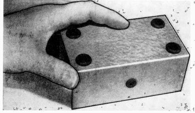
**Drill four holes** in the bottom of the metal box and insert rubber grommets to prevent scarring or scratching of furniture.
