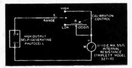
source, throw switch S to its low position and adjust rheostat R for half-scale (0.5 ma.) deflection of the meter. Tighten the rheostat shaft lock. This completes the adjustment.
