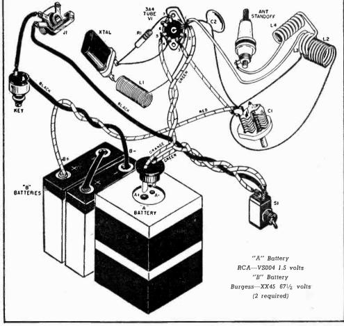
cover holes. Mount the tube and crystal socket on the chassis before bolting the chassis to the cover with 4-40 %'' machine screws.
