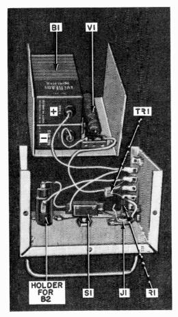
ment. Check Fig. 3 carefully for assembly details. When completed, a Burgess No. 7 penlite cell will fit nicely inside.
