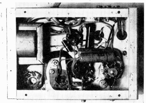
Fig. 2. Under chassis view of the amplifier showing how components are mounted.
