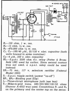
dary were not used) T2-Output trans. 10,000 ohms to 2500 ohms (Stancor A-4713 or equiv.) The bottom half of the split secondary was not used) V1—117L7GT tube
