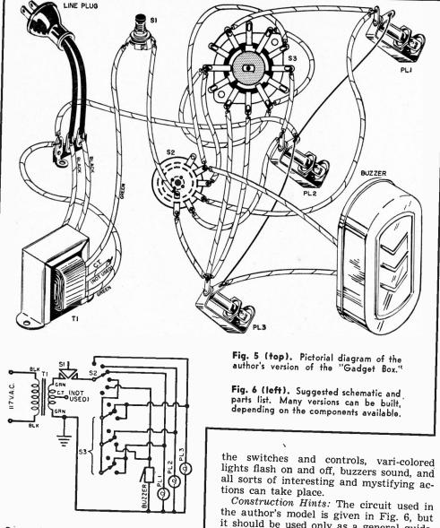
Buzzer-6-8 wolt buzzer (Edwards No. 725 or equivalent) PLI, PL2, PL3-
