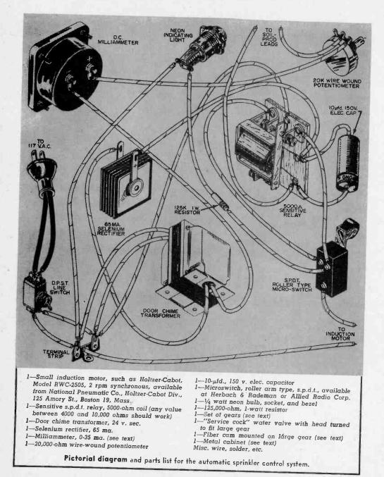
garden. Insert them to the desired watering depth probably 3" to 5". With the water valve in the "off" position, rotate the gear wheel with the fiber cam attached so that the cam just releases the microswitch arm; then secure the gear wheel to the valve head and turn the control unit on. The motor should turn the valve to the "on" position where the motor will stop. When the area being monitored has received sufficient moisture, adjust the potentiometer so that
