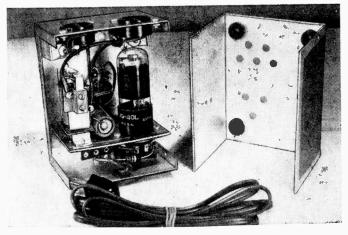
Fig. 6. The timer is shown here with the wiring and assembly completed, but before the two parts of the cabinet are assembled. Note the position of the sub-chassis and parts layout. The layout is not critical but it is best to keep it neat and compact.
