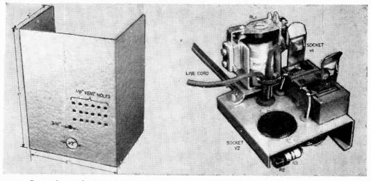
Rear of case for Photoelectric Light Switch.
