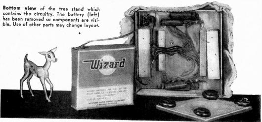
the pliers, instead of up the wire to the plastic. Put spaghetti tubing over the resistor leads before soldering. The lamp on the tree top, which will not flash, does not need the extra lead to run down into the base. Connect a resistor to one lead of this lamp and a wire to the other to reach the "B--" bus wire.
