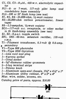
chassis and cabinet are used, this presents no problem; but in the case of the compact unit shown, great care in planning and layout were necessary. The sockets recommended in the parts list require a  $1\frac{1}{4}$ " hole for the four-prong socket (868) and a 1" hole for the octal socket (2050). These holes are punched one behind the other, allowing ample room between them for the bulge in the thyratron envelope.
