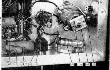
**Close-up view** showing wiring of "volume control" oscillator and part of the power supply.
