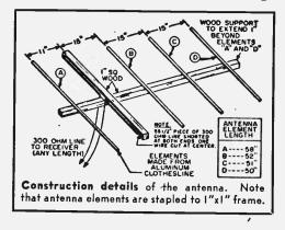
300-ohm twin lead for the lead-in and radiator. If all parts are purchased new, total cost should not exceed \$1.50.
