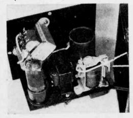
Under chassis mounts rectifier and electrolytic.
