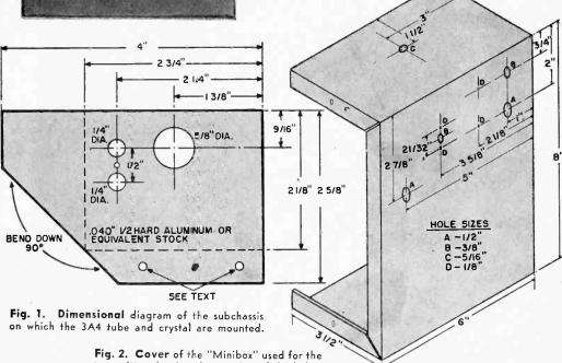
transmitter showing the position of the holes.
