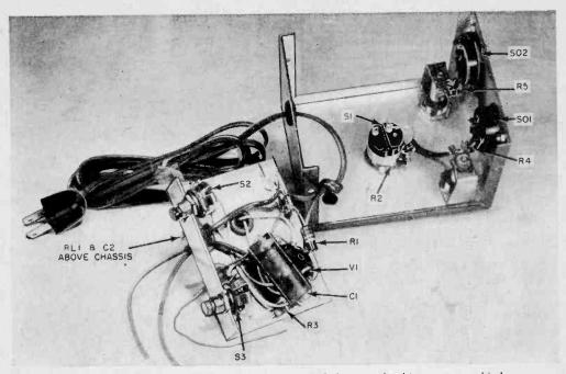
Fig. 2. All possible wiring is done before the subchassis and cabinet are assembled.
