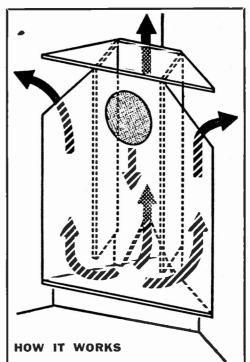
The Mark II is a labyrinth type of enclosure. Air passages created by the maze help load and damp the speaker cone. Loading enables an efficient transfer of acoustic energy (sound) from vibrations in the speaker cone to air mass in the listening room. Damping reduces bass boom by restricting excessive cone excursions at resonant frequency.
