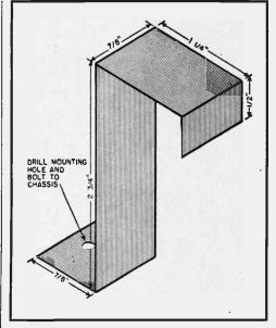
Fig. 3. Bracket for holding the B battery. This part may be made from copper, brass or aluminum.
