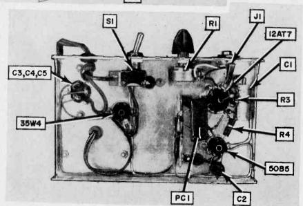
Only a few general precautions need be observed when wiring the amplifier. Carefully follow both the schematic and pictorial wiring diagrams, checking one diagram against the other as the wiring proceeds. Keep all signal leads as short and direct as possible. Insulate bare leads with spaghetti tubing. Don't bend the leads of the printed circuit plate too sharply as they may break off close to the plate.
