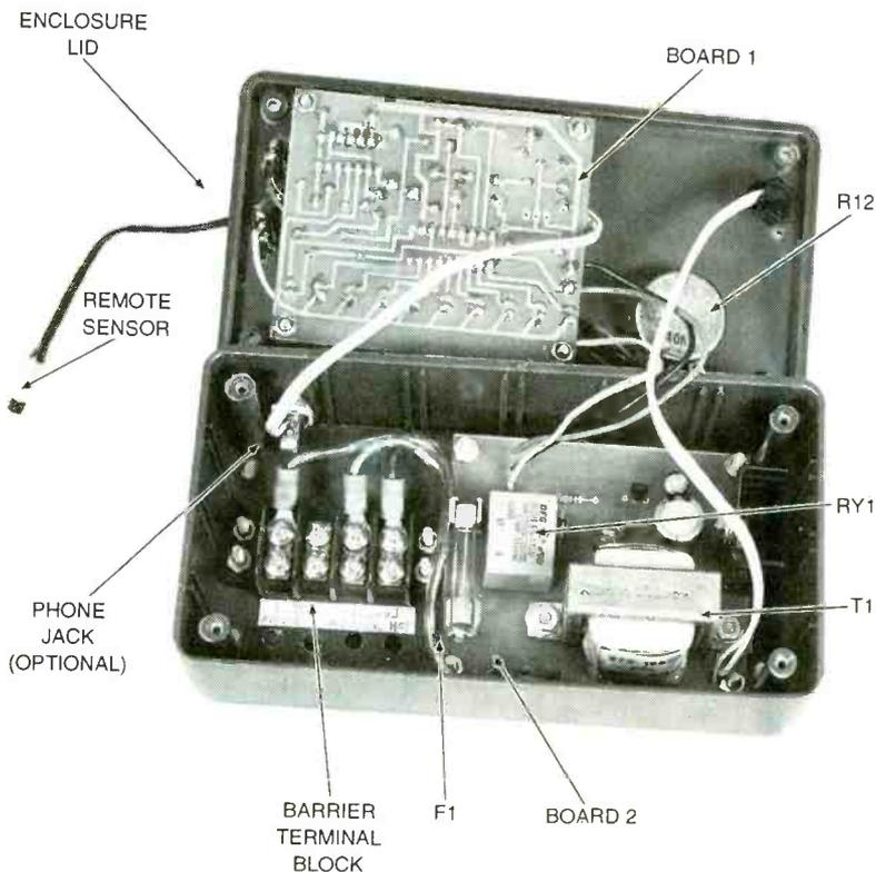
The two printed-circuit boards, as well as the off-board components that make up the Electronic Climate Controller's circuitry, are easily housed in and mounted on the unit's simple plastic enclosure. The optional barrier block makes it easy to wire the unit into your existing climate control system, while the optional phone jack allows for easy connection of a remote sensor.
