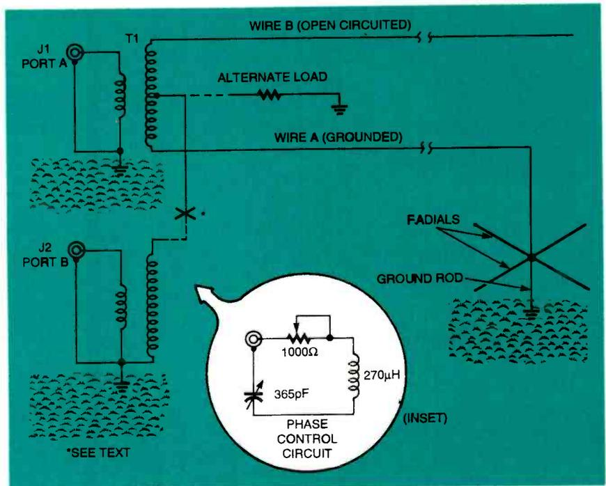
Fig. 10. Steerable-notch Beverage antenna.
