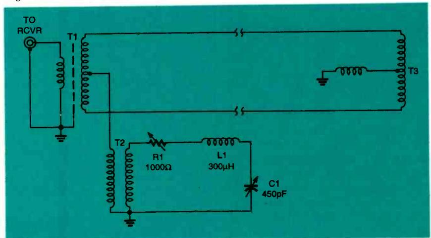
Fig. 11. Balanced version of the steerable-notch Beverage.
