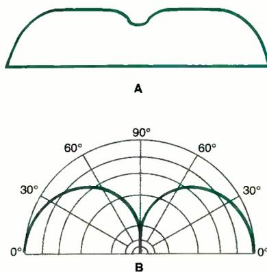
Fig. 1. The cross section of a bagel sliced horizontally in half (A) can represent the ideal elevation pattern for a quarter-wave vertical antenna over perfect ground (B).
