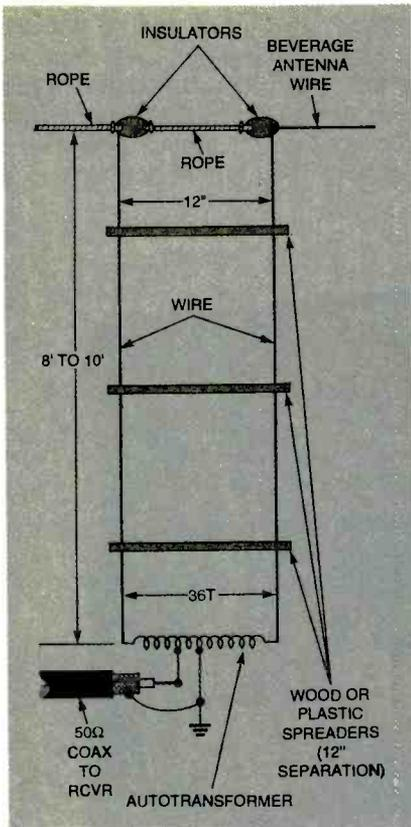
Fig. 9. Zepp-fed Beverage antenna.
