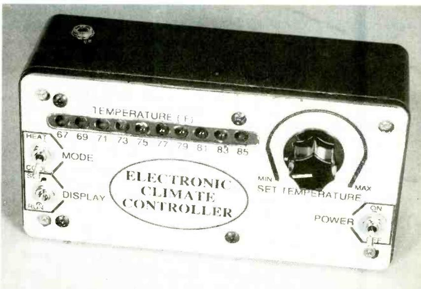
The appearance and functionality of the finished project can be greatly enhanced by affixing a photocopy of the author's front panel label to the lid of the enclosure. The label includes switching designations as well as outlining the significance of each lighted LED.
