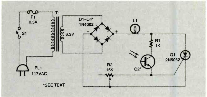
Fig. 7. This trick circuit uses a photo-transistor and SCR to control lamp L1. Light impinging upon Q2 turns on the lamp—removal of the light turns the lamp off.
