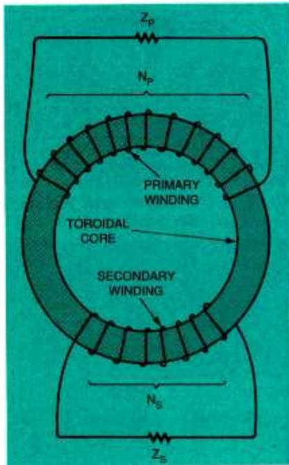
Fig. 6. Toroid transformer for the receiver end.
