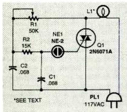
Fig. 10. This circuit is used in many lamp-dimmer applications. Once the lamp is lit, continuous control of its brightness is obtained by varying potentiometer R1.
