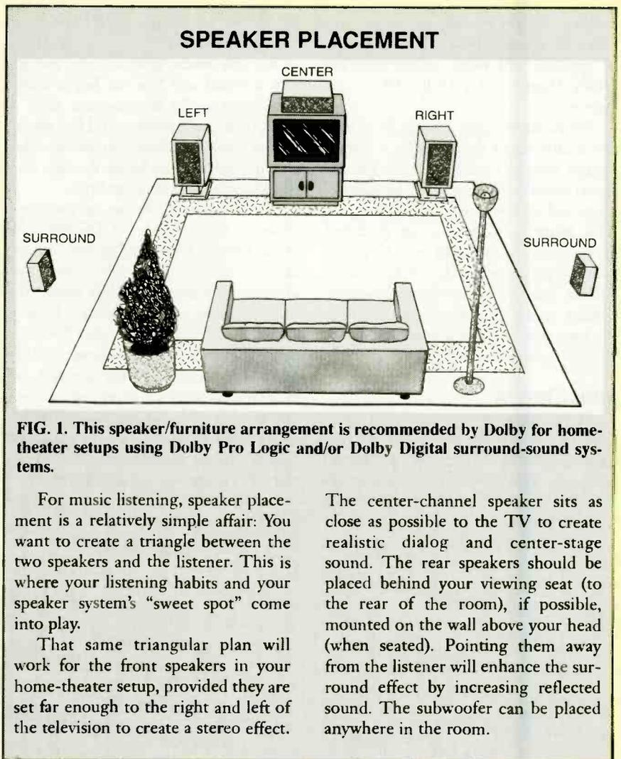
**FIG. 1.** This speaker/furniture arrangement is recommended by Dolby for home-theater setups using Dolby Pro Logic and/or Dolby Digital surround-sound systems.
