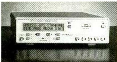
The unit automatically acquires and tracks satellites, and calculates time, frequency, and position within 2 to 15 minutes after power-up. Synchronization is confirmed via a front panel LED indicator. The actual deviation can be read on a 2 × 20 character LCD. In the field, the geographic position can be read from the LCD screen.
