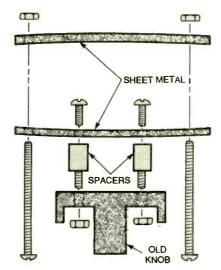
Fig. 1. The paint-shaker module can easily be made by mangling a perfectly good printer-platen knob.
