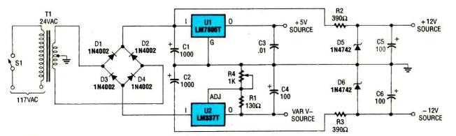
Fig. 2. This power-supply is more than adequate for the ADC. In fact, you can leave out certain components if you don't need an adjustable negative-voltage supply.
