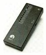
measured. The device's bandwidth goes from 20 to 10,000 Hz, enabling it to measure almost all extremely low frequency (ELF) and some very low frequency (VLF) fields. The ten-segment LED bargraph has two ranges and a power on/off indicator.
