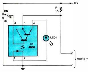
Fig. 3. A simple but versatile bouncless switch can be made from one opto-isolator and a couple of additional components. (Note: the external LED is optional.)
