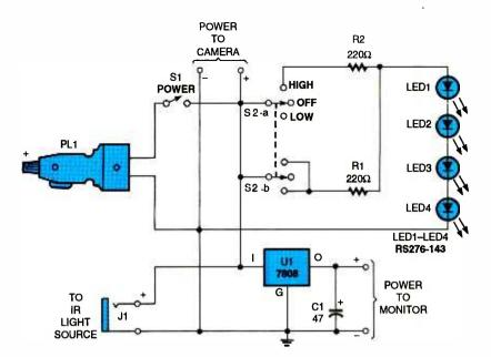
Fig. 3. Power for the NightVision View Scope is provided by a 12-volt, 7-amp/hour battery pack. The supplied power is regulated to 8 volts by U1, and is then used to power the video monitor.
