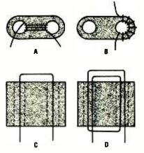
Fig. 3. Binocular cores can: be center wound (or normal) (A), edge wound (B), have a single-turn winding (C), or have a multiple-turn winding (D).
