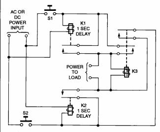
Fig. 6. This circuit is sure to keep both of your hands from the business end of a tool during operation. To use it one must depress and hold down both SI and S2.
