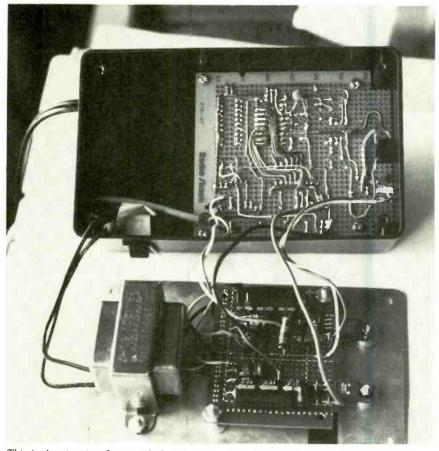
This is the circuitry for the whole prototype. It fits into a  $6/4 \times 3^{3/4} \times 2$  project box with an aluminum cover. The box contains the transformer, power-supply circuit board and the main-circuit board nicely with little room to spare.
