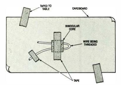
Fig. 4. For this method of winding binocular transformers a piece of cardboard is needed to secure the core.
