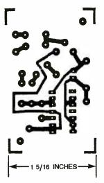
Fig. 7. The IR-illuminator circuit was assembled on a printed-circuit board. A template for that printed-circuit layout is shown here full size.
