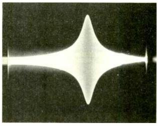
Fig. 1. Here is the output signal of the RSG-30 after passing through a 10.7-MHz IF-transformer-based tuned LC resonant circuit. Note the peaked response of the transformer.
