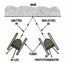
Fig. 5. This simple arrangement can be used to detect the blood density in an area of the skin by bouncing some infrared light off its surface.
