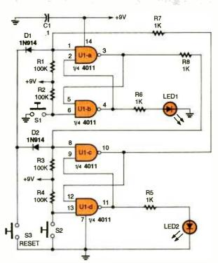
Fig. 2. This first-response monitor functions in the same manner as the previous one, but uses a digital IC---a 4011 quad 2-input NAND gate-instead of SCR's.
