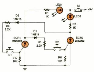
Fig. 1. The analog first-response monitor is built around a pair of cross-coupled SCR's, each of which receives its gate trigger current from the anode of the other SCR.
