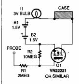
Fig. 5. This simple tester is very useful and doesn't require a return lead provided your body is at least slightly grounded.
