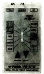
equipment, the VG-510 is also a handy tool for video editing. Black burst can be used to lay down black on tapes and to record SMPTE color bars with tone at the beginning of the tape. Audio output is 1 kHz with an adaptor included for 120-volt studio use. The unit measures  $5\frac{1}{2} \times 3\frac{1}{2} \times 1\frac{1}{2}$  inches and weighs less than a half pound without batteries.
