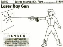
Advanced project produces a burst of light energy capable of burning holes in most materials. Hand-held device uses rechargeable batteries. 500 joules of flash energy excite either a neodynium glass, yag or other suitable 3" laser rod. This is a dangerous CLASS IV project (individual parts/assemblies available).
