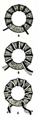
Fig. 1. These toroid cores: are A) single wound; B) bifilar wound (three wires would be trifilar wound); and C) twisted bifilar wound.
