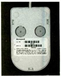
Here's an underside view of the Honeywell mouse. It's lack of a ball mechanism offers some significant advantages over standard devices.
