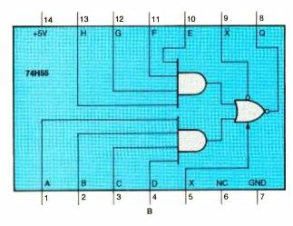
Fig. 1. The 7455 comes in two forms: a plain unit in the lowpower and lower-power Schottky formats (A), and an expandable device in the high-power style (B).
