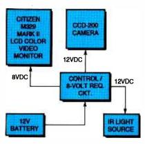
Fig. 1. The NightVision View Scope is comprised of four subassemblies: a camera, a video monitor, a control/ voltage-regulator circuit, and an IR light source.
