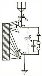
Here's the schematic of a tapped-coil crystal set that is very similar to the NBS version. Tuning capacitors (dotted lines) are not used.
