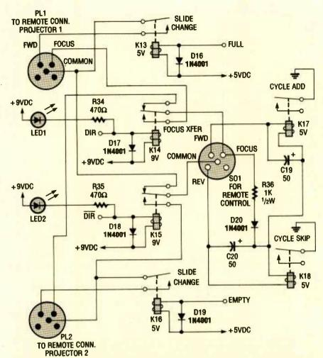
Fig. 6. The transfer relays provide the required transformer-winding isolation, transfer the remote control functions to the active (full bright) projector, and send a slidechange command to the projector that has just gone full dark.
