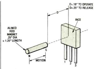
Fig. 4. If the south pole of a permanent magnet is brought in proximity to the sensor area (within about .18 inches of its face), as shown here, the Hall-effect switch's output transistor turns on, completing the ground path for LEDI, causing it to light.
