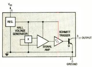
Fig. 1. The UGN-3113U is a magnetically operated, solid-state Hall-effect switch comprised of a Hall-voltage generator, a signal amplifier, a Schmitt trigger, and a transistor-output circuit, as shown by this block pinout diagram.
