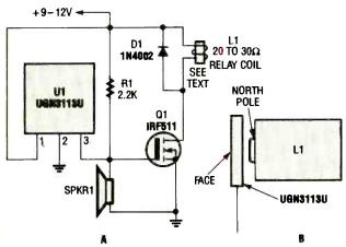
Fig. 7. While not intended for this application, Hall-effect switch can be used a the basis for a rather unusual oscillator, as shown here.
