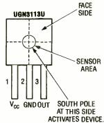
Fig. 2. In operation, the UGN-3]13U Hall-effect switch is activated by bringing the south pole of a permanent magnet within a specified distance of the device's sensitive area (located on the face side).
