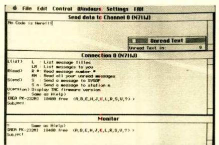
AEA's MacRATT is an Apple-friendly terminal program for use with their popular PK-232MBX Multi-Mode Data Controller. Used together they let you communicate over the full range (HF and VHF packet, AMTOR, WEFAX, ASCII, Baudot RTTY, and manual Morse code) of digital modes.
