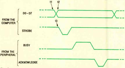
Fig. 2. Once a computer sets up the data on the parallel data lines, it signals the peripheral with a low-going strobe pulse. The peripheral responds by sending the busy line high until it's ready for more, and/or it waits until its finished with the data and sends a low-going acknowledge pulse.
