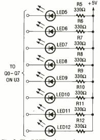
Fig. 2. The POST codes can be displayed by 8 LED's. This is a good low-price alternative to using the T1L311's.
