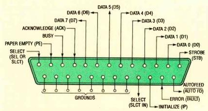
Fig. 1. The parallel port on most IBM-compatible (and some non-compatible computers) looks like this. The arrows pointing away from the DB-25 connector are outputs, the ones pointing to the connector are inputs, and the remaining pin outs (shown with circles) are grounds.
