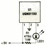
Fig. 3. When U1 is connected as shown and no magnetic field present, the output transistor is off (open circuited), so no ground path through the output transistor is provided, thus, LED1 remains dark.
