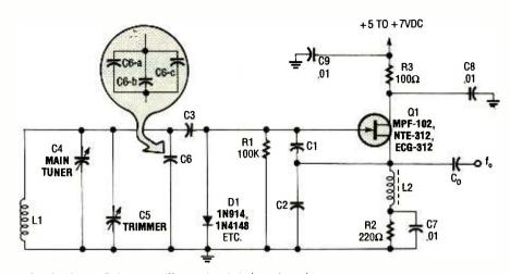
Fig. 2. This basic Colpitts oscillator circuit is based on the junction field-effect transistor (Q1) whose drain is kept at RF ground by decoupling capacitor C8.
