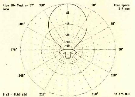
Shown here is a representative polar antenna pattern printout from the YO software package. YO can model stacked Yagis, dual-driven and tapered elements, matching networks, and account for skin effect, and ground effects from HF to microwave.
