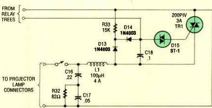
Fig. 5. The Triac lamp dimmer circuits are controlled by the relay trees and they, in turn, control the projector lamps.
