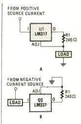
Fig. 2. Adjustable regulators that float can be used as current limiters. Positive regulators can limit the current from a voltage source to a load (A), and negative regulators limit the current from a load to ground.
