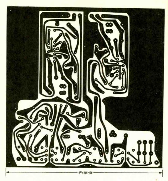
Fig. 2. The amplifier can be purchased in kit form (with all the components necessary to assemble the circuit), or you can etch you own board using the foil pattern shown here.
