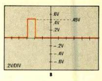
Fig. 4. Increased vertical sensitivity will enhance the accuracy of your readings. As proof of that, the detail lacking in A shows up in B.
