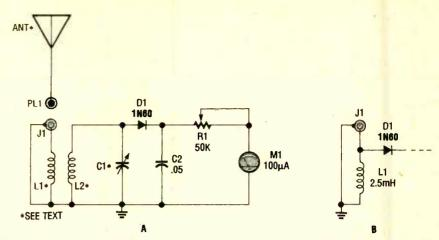
Fig. 6. To build a tuned RF wavemeter follow the schematic shown in A. For an untuned version replace L1, L2, and C1 in A with L1 in B as shown.
