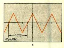
Fig. 5. Increasing horizontal sensitivity will enhance the accuracy of your time readings. The expanded version of the wave in A is shown in B.
