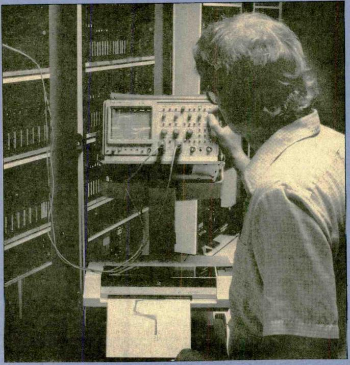
While this mode is useful for close inspection of typical waveforms, it will not readily display small transient signals, which often require even faster sweep rates. Most scopes today have a "delayed sweep" feature that overcomes that. It allows a user to view any portion of a waveform at a very fast sweep rate to yield high horizontal resolution,
