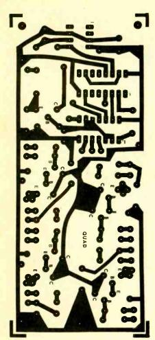
Fig. 2. The Quad Tracer was built on a printed-circuit board, measuring 4% × 2% inches; here is the full-scale template of that PC pattern.
