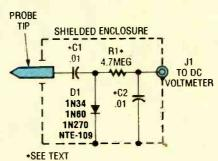
Fig. 2. This RF-detector probe can allow your DC voltmeter to indicate the presence of powerful radiowaves.
