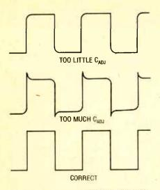
Fig. 3. This diagram shows the effects of the probe's capacitive reactance on an input square-wave signal.
