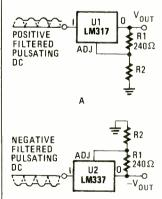
Fig. 1. Adjustable regulators are easy to use. Whether you need a positive (A) or a negative (B) output voltage, you just have to add two resistors and a filtered source of pulsating DC.
