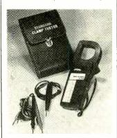
ture meter readings. Also supplied are a set of voltage test probes, a resistance test probe, a spare fuse, a carrying case, and an operating manual. The compact instrument weighs just over 16 ounces.
