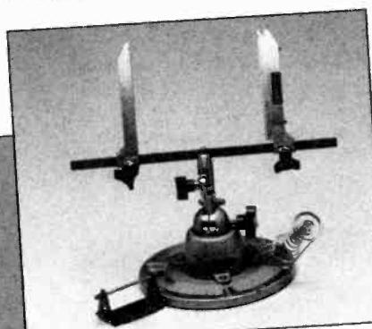
**ELECTRONIC WORK CENTER:** A complete combination to make work areas more efficient and manageable! Circuit Board Holder gently, but firmly, holds PCB's up to 12" wide. Add our Standard Base (moves in three planes), Tray Base Mount (with parts wells), and Solder Station (self-centers wire and holds iron at perfect angle) for a great combo! Model #324. \$54.95.
