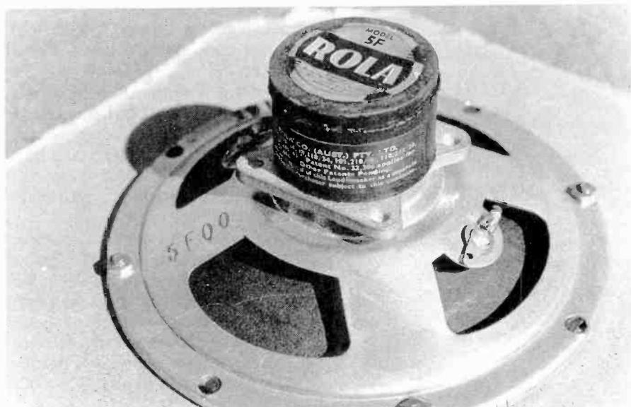
*This Rola permag loudspeaker still has the flange and bolt holes where the field coil bolted on in an earlier design. A number of manufacturers retained the field coil frame for some of their early permanent-magnet speakers.*
