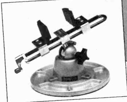
**MULTI-PURPOSE WORK CENTER:** Self-Centering Extra Wide Opening Self-Centering Extra Wide Opening Head (opens to 9"), famous "split ball" Standard Base (moves in three planes), Standard Base Mount (with parts wells), and convenient Tray Base Mount (with parts wells) handle difficult to hold items with ease! Model #350. \$52.95.
