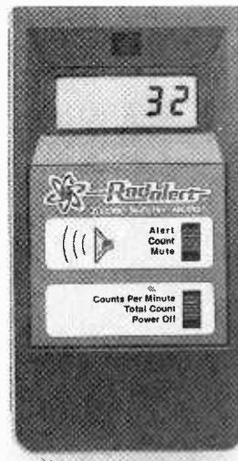
level. The unit can be interfaced to a computer for recording monitored levels, or to an external warning device. The Geiger-tube radiation detector is sensitive enough to measure radiation from uranium-oxide pottery glazes, old radium-dial clocks and watches, gas camping-lantern mantles, and rock collections. The Radalert is powered by a 9-volt battery; a jack is provided for an optional AC adapter.
