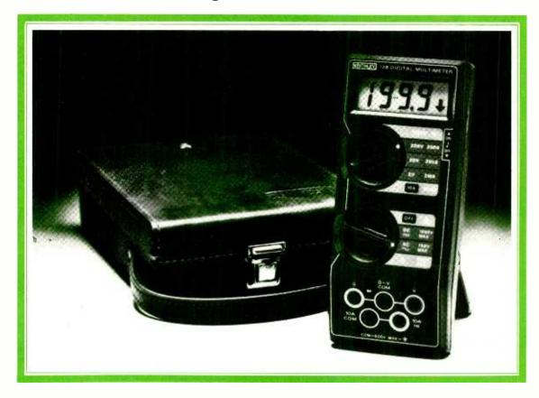
THE Keithley Model 128 Digital Multimeter was designed for the general-purpose service market. It offers 0.5% basic accuracy, 3½-digit, 0.6" LCD display, resolution to 1 mV/0.1 ohm, 10-ampere ac/dc current capability, and resistance measurements to 20 megohms. One of its interesting features is a presettable "beeper" that operates on all ranges and functions. The beeper
