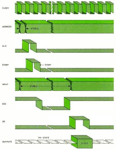
Fig. 2. Timing diagram of the analog-to-digital converter IC.
