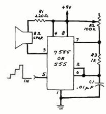
Fig. 5. A simple voltage-controlled oscillator.
