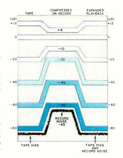
Fig. 1. Waveforms showing the dynamic range of the CX noise-reduction system.
