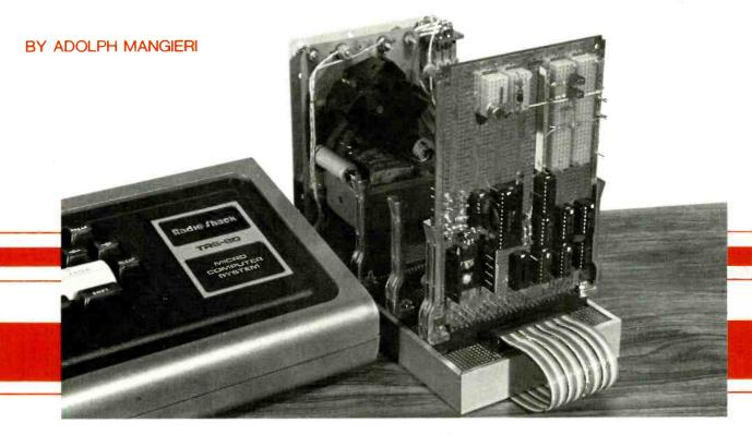
IGITAL computers "speak and understand" only the binary language of electrical ones and zeros. Unfortunately, the binary language is not suitable for direct measuring of physical quantities such as voltage, pressure, temperature, light, or other continuously varying (analog) parameters. To utilize the digital computer in measurement and control systems, an analog-to-digital interface is required. Fortunately, such analog-to-digital converters (ADC) are now available at low cost.
