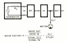
Where  $P_i$ 1 is the signal input power required to generate a signal-to-noise output ratio of 1.
