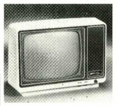
including vertical size. Bandwidth is greater than 12.5 MHz, and rise-time is about 60 ns. Dc-coupled circuits are used, refresh rate is 60 Hz, and power dissipation is 26 W. It is housed in an orchard brown cabinet and compatible in style with Apple systems. Address: Zenith Data Systems, 1000 Milwaukee Ave., Glenview, IL 60025 (Tel: 312-391-8181).
