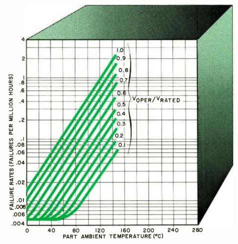
Fig. 1. A typical chart of the effects of temperature on failure rates for general-purpose ceramic capacitors. (MIL-C-11015).
