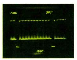
Fig. 4. Color bar pattern test showed good results although the edges of some individual colors lost some sharpness.
