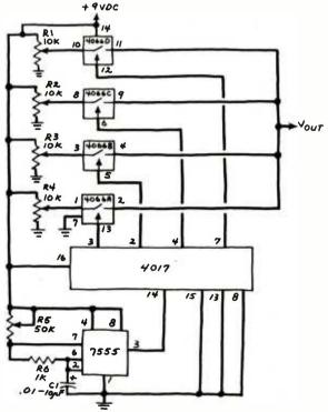
Fig. 2. Programmable four-step function generator.
