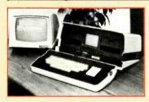
The Osborne 1 computer measures 20.5"W x 13"D x 9"H and weighs 23.5 lb. The main pc board uses the Z80A processor with a 4-MHz clock; memory size is 64K RAM, 4K ROM. Interfaces are RS-232 C and IEEE 488. User controls consist of a 69-key detachable keyboard with a 12-key numeric pad; brightness and con-
