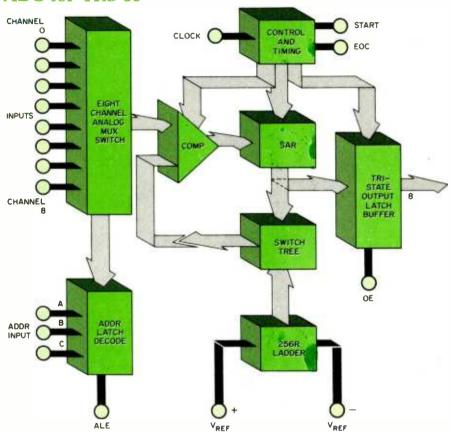
Fig. 1. Block diagram of the circuits contained in the ADO809 analog-to-digital converter used in the project.
