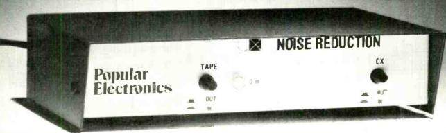
everything below -40 dBV is boosted 20 dB. As the signal increases from -40 dBV to 0 dBV, the gain reduces so that by 0 dBV there is 0 dB or unity gain. Above 0 dBV, the gain continues to fall so that a +12-dBV input is reduced by a -6-dB gain for a +6-dBV output.
