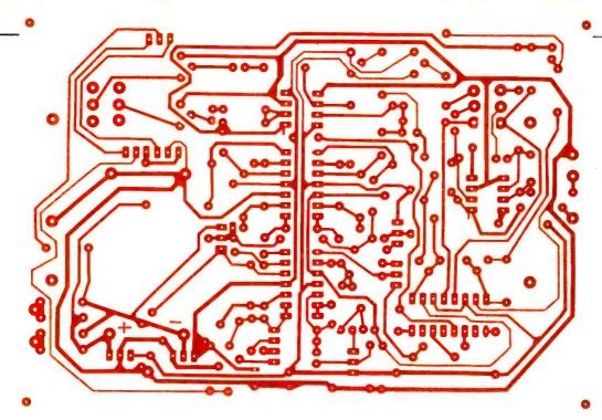
Fig. 3. Actual-size foil pattern for the printed-circuit board is shown above.
