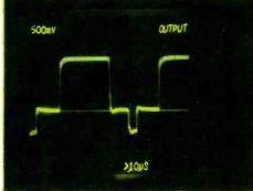
Fig. 3. In the window-pattern test, the scope picture, here, shows loss of high-frequency performances; but the window on the TV set was excellent.
