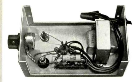
Photo showing how the author assembled his prototype of the electronic electroscope on an aluminum chassis.
