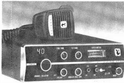
tice filter is said to provide a high degree of adjacent-channel rejection. On transmit, a speech compressor increases average modulation levels. The clarifier or "fine-tune" control is claimed to have exceptionally smooth operation and a center-notch position for easier adjustment. \$359.95.
