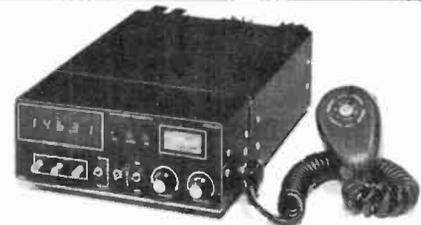
**First** and only school with designed-for-learning, 400-channel, digitally-synthesized VHF Transceiver to give you the only fully-up-to-date 2-meter equipment for complete training in commercial, amateur, and CB communications. The design incorporates circuitry and components representative of the latest state of the art. Circuitry is on five plug-in circuit cards to take full advantage of NRI "Power-On" training.
