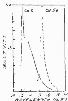
Fig. 1. Spectral response of CdS and CdSe photoresistors.
