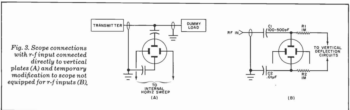
Fig. 3. Scope connections with r-f input connected directly to vertical plates (A) and temporary modification to scope not equipped for r-f inputs (B).
