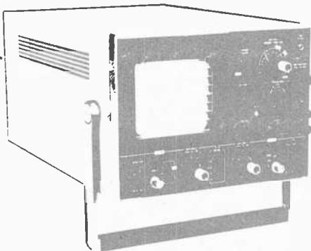
**E**VERYONE who gets into electronics, either vocationally or as a hobby, hopes to own an oscilloscope. This isn't surprising, considering that the scope is one of the most versatile test instruments ever to become available. Not only can an oscilloscope display a "picture" of the actual signal in a circuit under test, it can also measure the signal's amplitude, frequency, and time period.
