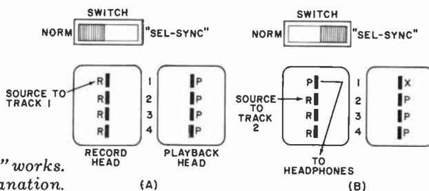
Fig. 2. How "Sel-Sync" works. See text for explanation.
