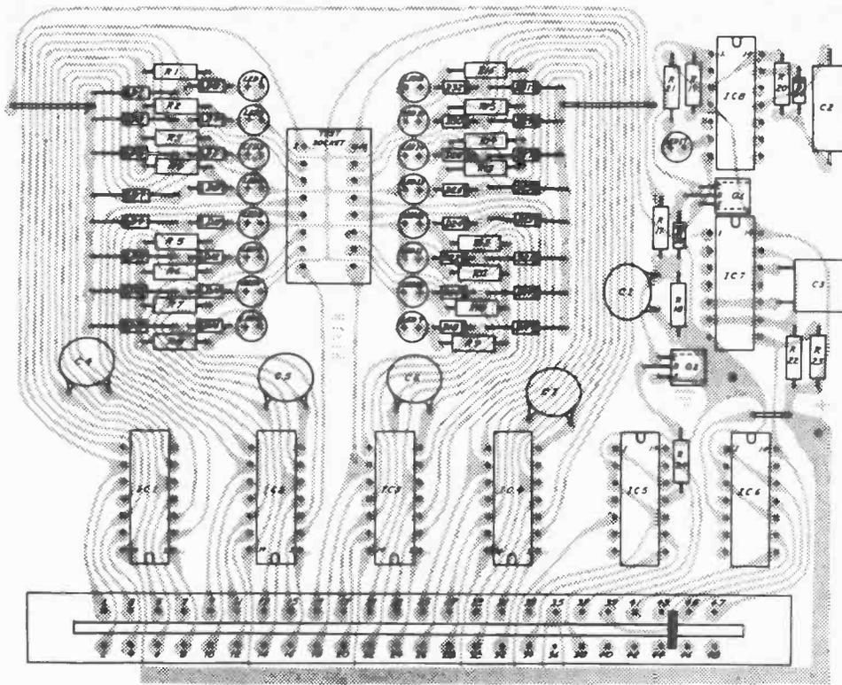
Fig. 4. Etching and drilling guide (right) and component layout (above) for main pc board. Note: etched and drilled pc boards for this and Fig. 5 are available from Select Circuits, 1411 Lonsdale Rd, Columbus, OH 43227 for \$18.95 a pair.
