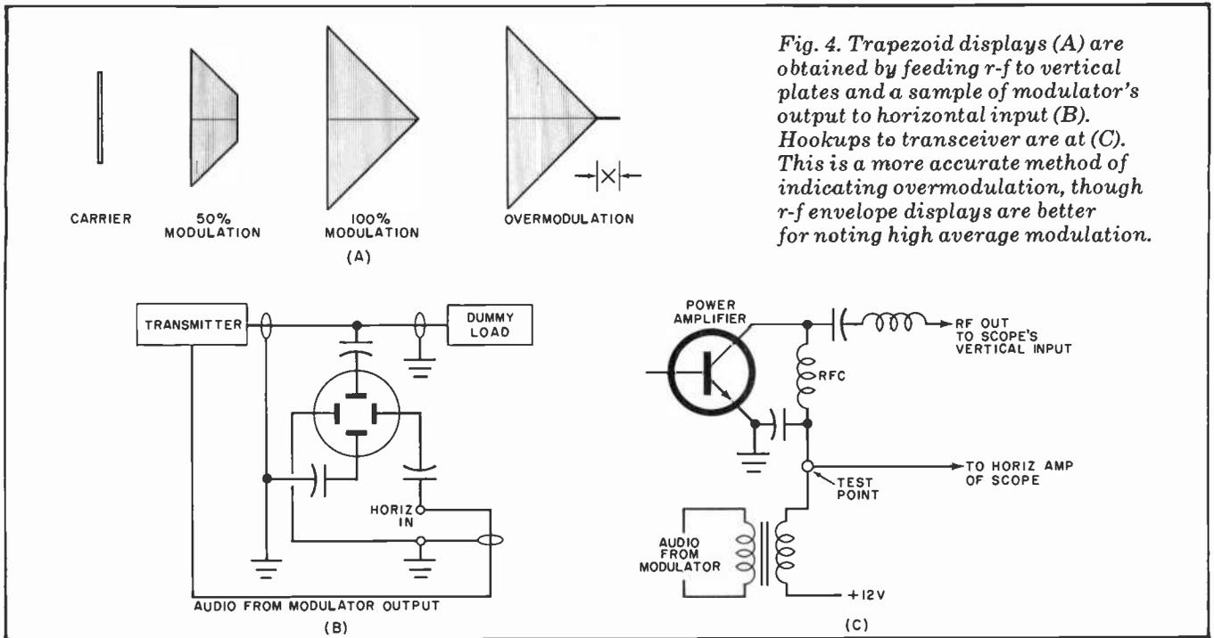
Fig. 4. Trapezoid displays (A) are obtained by feeding r-f to vertical plates and a sample of modulator's output to horizontal input (B). Hookups to transceiver are at (C). This is a more accurate method of indicating overmodulation, though r-f envelope displays are better for noting high average modulation.
