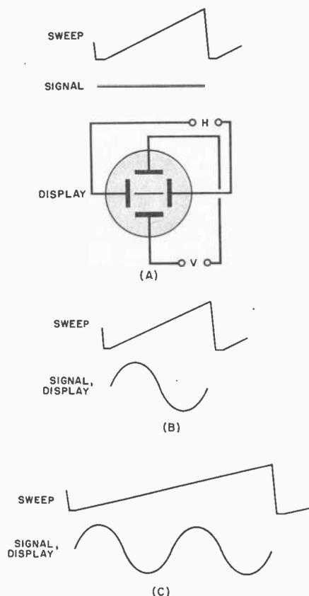
Fig. 3. Display depends on horizontal input and sweep.
