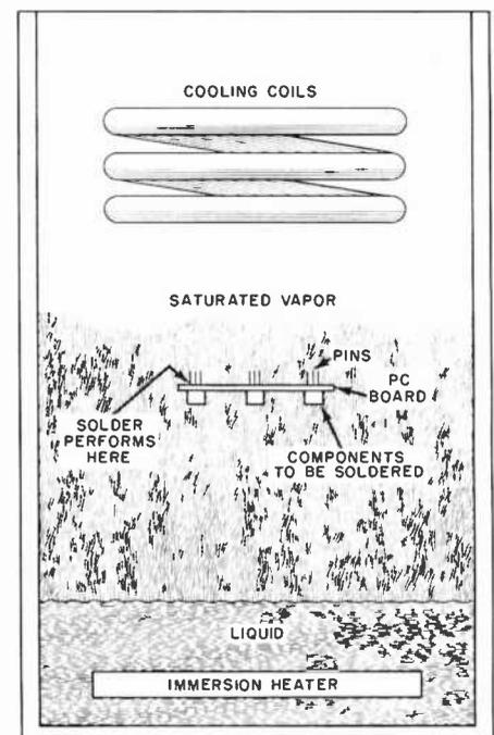
*Mac's sketch of condensation soldering system shows how boiling liquid is heated to form saturated vapor. When the vapor condenses above, the latent heat of vaporization melts solder.*
