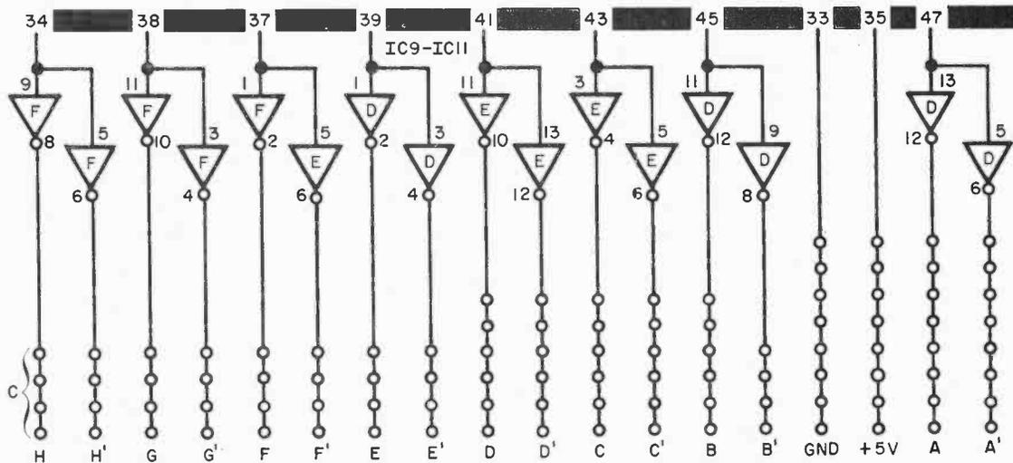
**About the Circuit.** The tester puts both IC's through their paces in parallel, covering all possible input combinations. The logic state at each input and output
