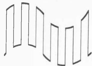
Fig. 7. Display with electronic switch in chop-mode operation.
