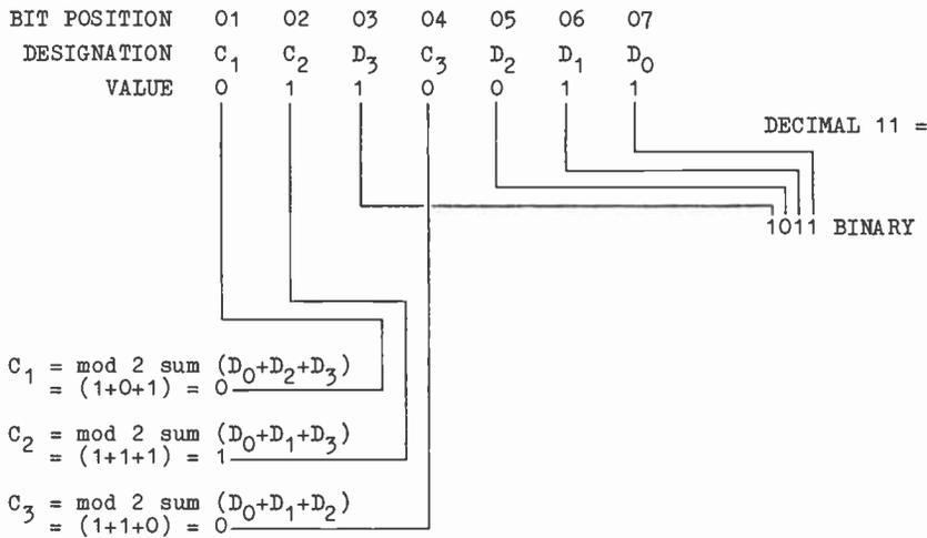
Fig. 3A. How Hamming-code check digits are generated.
