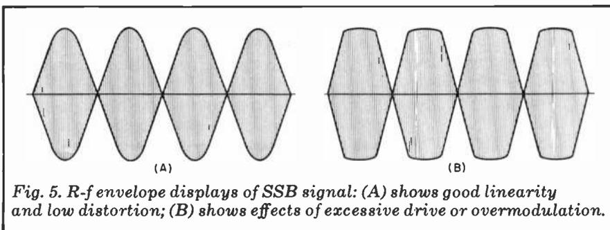
Fig. 5. R-f envelope displays of SSB signal: (A) shows good linearity and low distortion; (B) shows effects of excessive drive or overmodulation.
