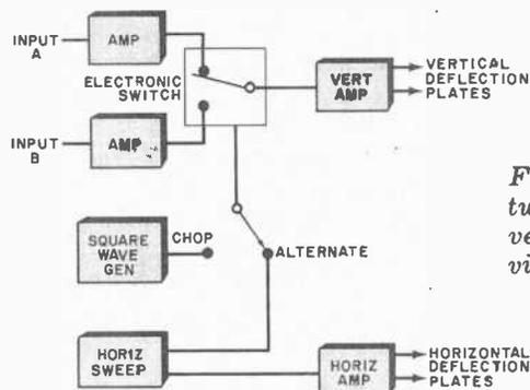
Fig. 6. In dual-trace scope, two signals are fed to vertical-deflection plates, via an electronic switch.
