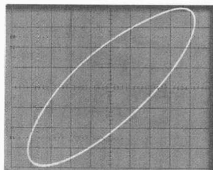
Fig. 8. Lissajous figures are used for phase measurements.
