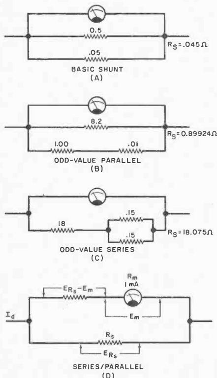
Fig. 2. Various configurations for using shunts with meters.
