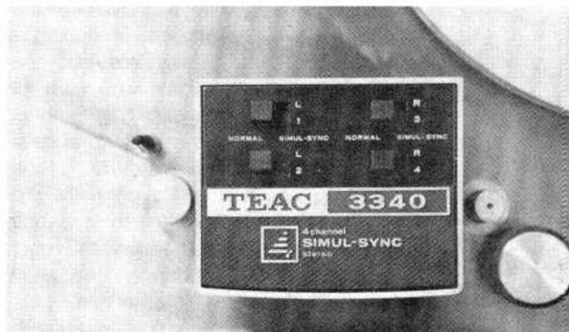
Closeup of "Simul-Sync" track switches on Teac 3340.
