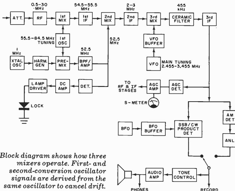
*Block diagram shows how three mixers operate. First- and second-conversion oscillator signals are derived from the same oscillator to cancel drift.*
