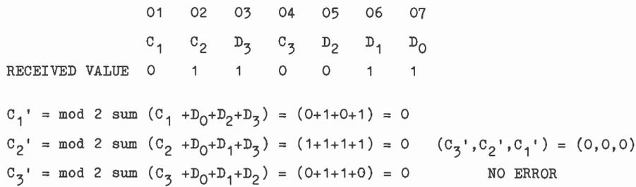
Fig. 3B. Check digits show that word was transmitted correctly.
