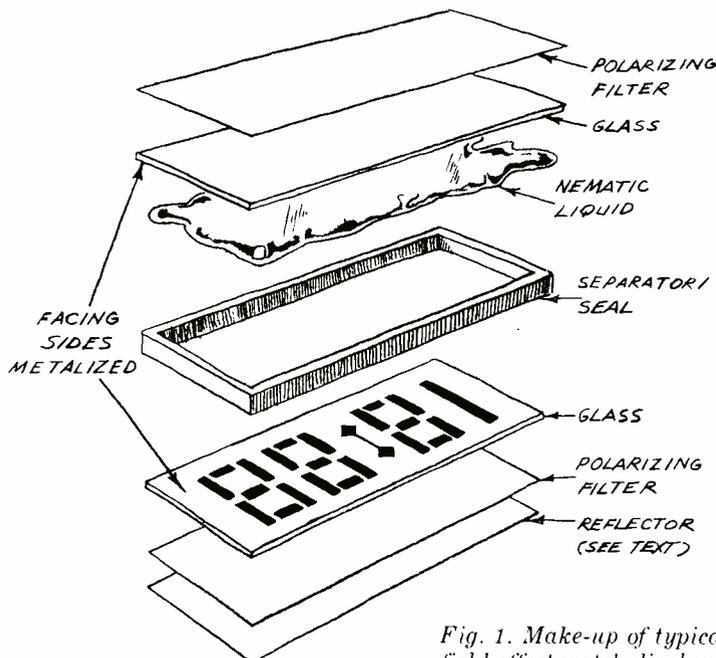
*Fig. 1. Make-up of typical field-effect watch display.*
