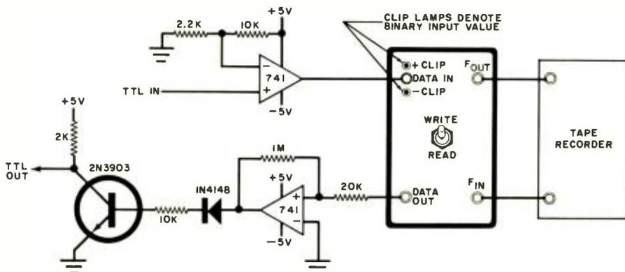
Fig. 6. Two op amps can be used in an external circuit to make the Translator compatible with TTL.
