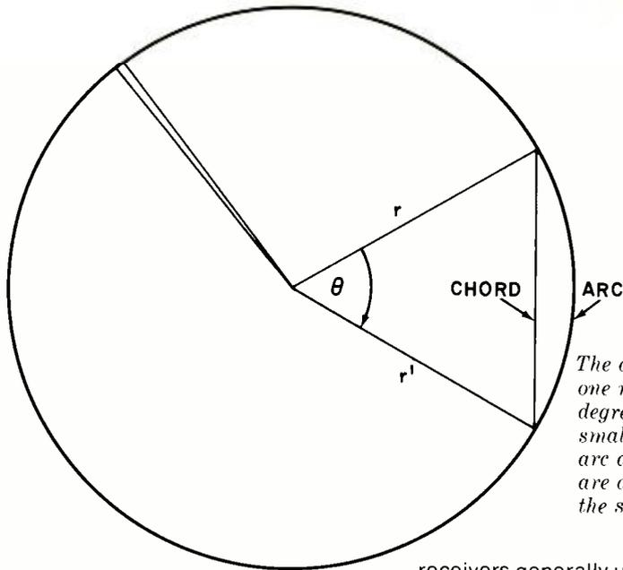
*The angle, theta, is one radian or 57.3 degrees. For very small angles, the arc and the chord are approximately the same length.*
