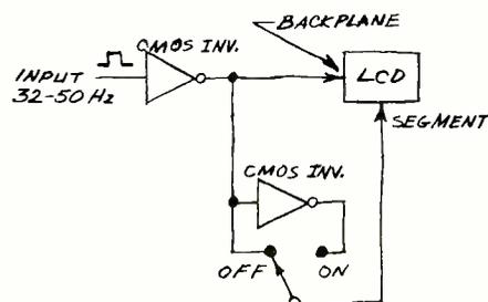
Fig. 3. Practical circuit for driving an LC display.
