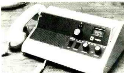
This feature permits private listening, and, Johnson claims, increased clarity of transmissions in noisy environments. Received signals can also be heard through a built-in or external speaker. An illuminated meter doubles as a received signal-strength and relative r-f output indicator. Squelch and volume controls are included.
