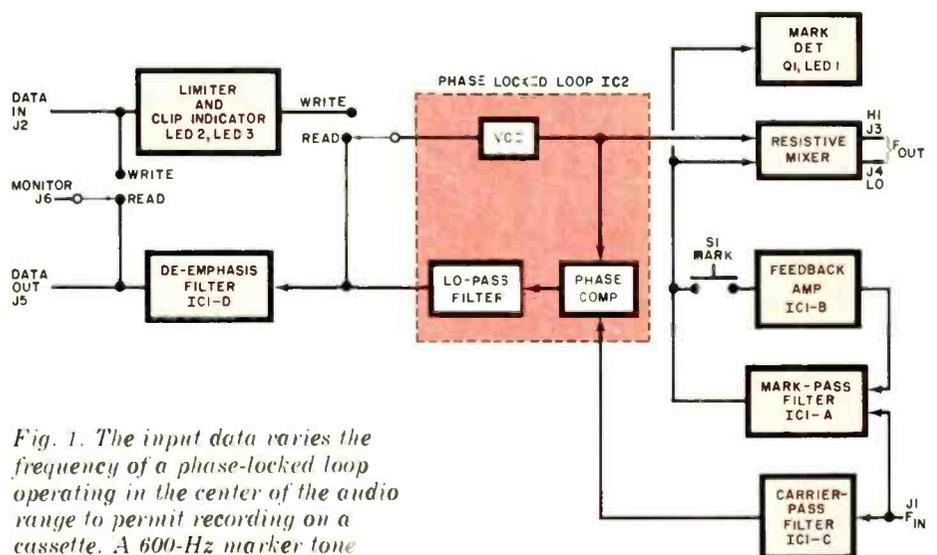
Fig. 1. The input data varies the frequency of a phase-locked loop operating in the center of the audio range to permit recording on a cassette. A 600-Hz marker tone can be inserted at any point.
