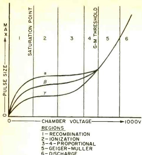
Fig. 4. Chamber voltage vs pulse size.
