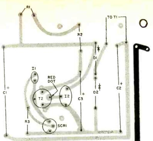
Fig. 2. Actual size foil pattern for the strobe cube is shown at right. Components are mounted as shown above.
