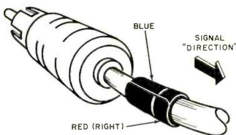
Wide blue band designates signal on color-coded band installed on cable.
