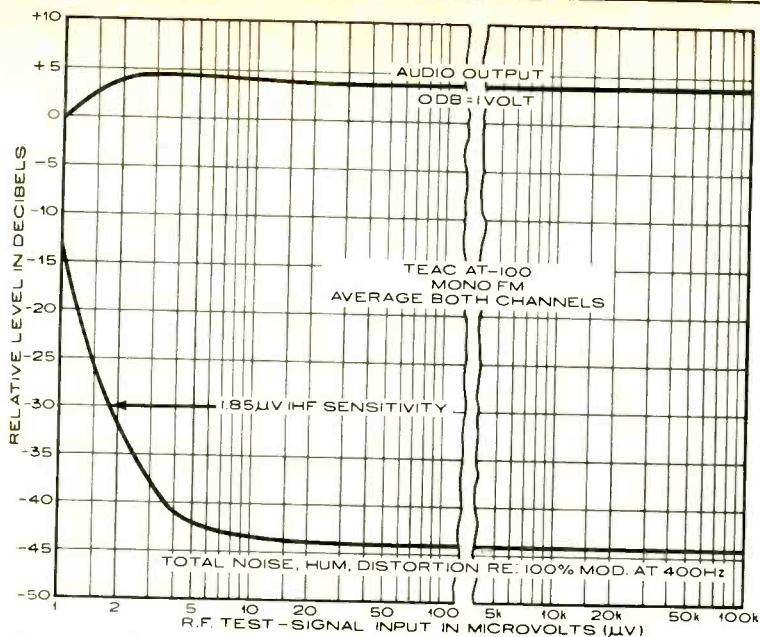
**Teac AT-100 tested out at 1.85  $\mu$ V IHF sensitivity. Audio output was 4.5 dB at 3  $\mu$ V r-f test signal input level, 4 dB out to 100,000  $\mu$ V.**
