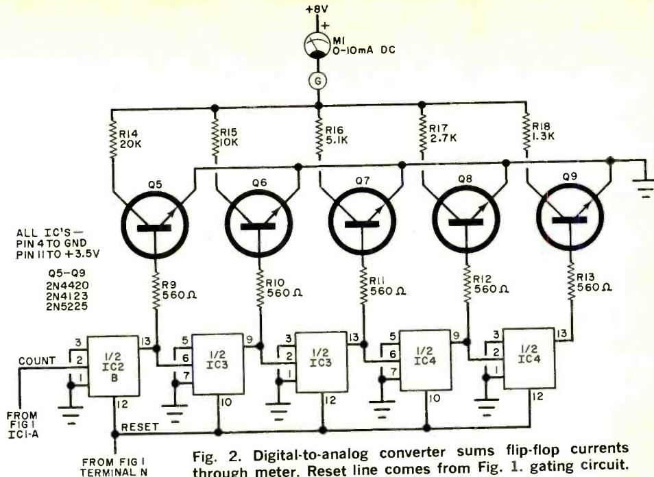
Fig. 2. Digital-to-analog converter sums flip-flop currents through meter. Reset line comes from Fig. 1, gating circuit.
