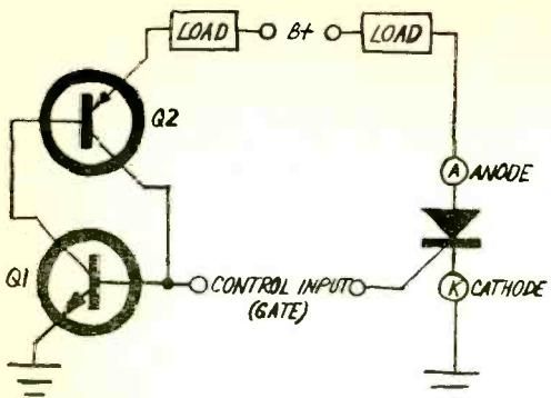
Fig. 1. The transistor circuit at left is equivalent to actual SCR at right.
