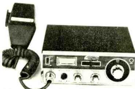
produces the last i-f. Channels are changed by switching in different crystals in proper combination at the first mixer. A delta-time setup at the second conversion oscillator has three positions which permit the receiver's frequency to be shifted by a given amount around the center frequency.
