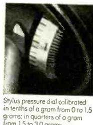
Stylus pressure dial calibrated in tenths of a gram from 0 to 1.5 grams; in quarters of a gram from 1.5 to 3.0 grams.
