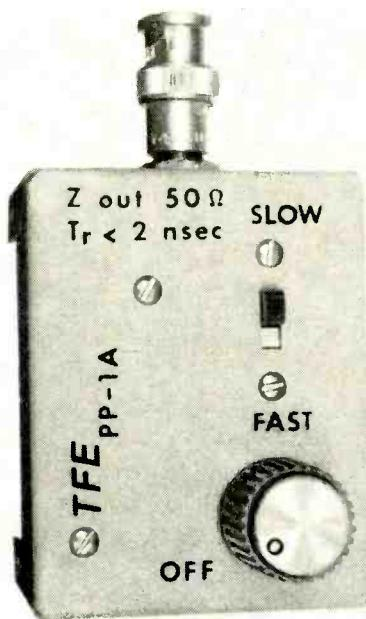
A SQUARE-WAVE generator is useful to have around an electronics workshop or on a home workbench for checking rise times of oscilloscopes, calibrating probes, toggling logic circuits, checking audio amplifiers, and the like. Such a generator can also be used by hams and SWL's to provide accurate frequency markers out to 30 MHz or so, due
