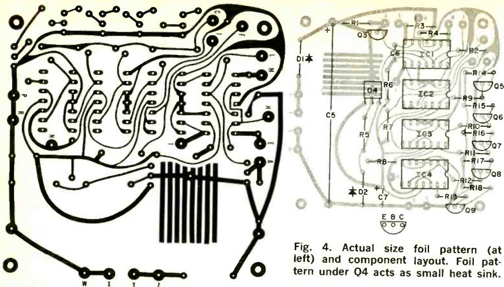
Fig. 4. Actual size foil pattern (at left) and component layout. Foil pattern under Q4 acts as small heat sink.
