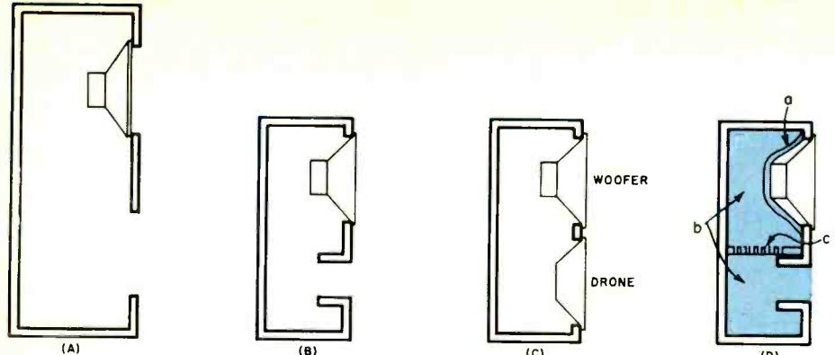
**Fig. 1. Types of reflex speaker systems.** (A) The classic bass reflex—full-size enclosure with port area equal to speaker cone area. (B) Ducted-port compact. (C) Auxiliary radiator reflex. (D) Methods of treating resonance problems include (a) collar of resistive material over speaker, (b) enclosure stuffed with damping material, (c) resistive panel. All the methods are usually not employed together.
