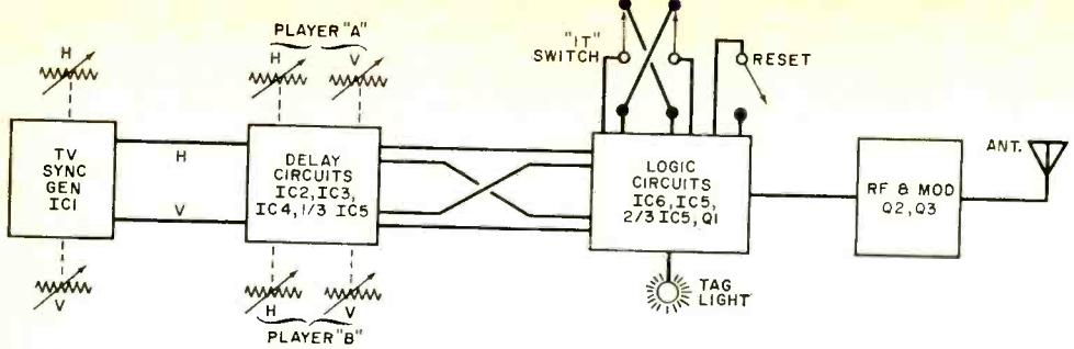
**Fig. 1.** The circuit of the TV Tag can be divided into four parts: a sync generator (same frequencies as monochrome TV), delay and logic sections, and r-f oscillator.
