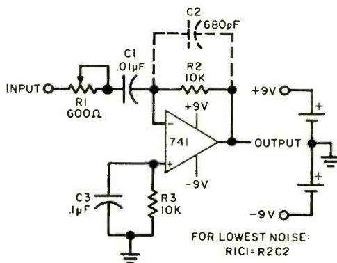
$$\text{HIGH FREQ. CUTOFF: } f_0 = \frac{1}{2\pi R_1 C_1}$$
