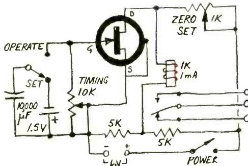
even better than those obtained with the original project. My circuit can be set for from 1 to 101 seconds and has a zero-set for the relay to put in just the right amount of current. I am sending along the schematic diagram of my design, hoping it can be of some use to your readers.
