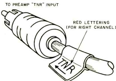
**If color coding is out, install this kind of label with simple lettering.**
