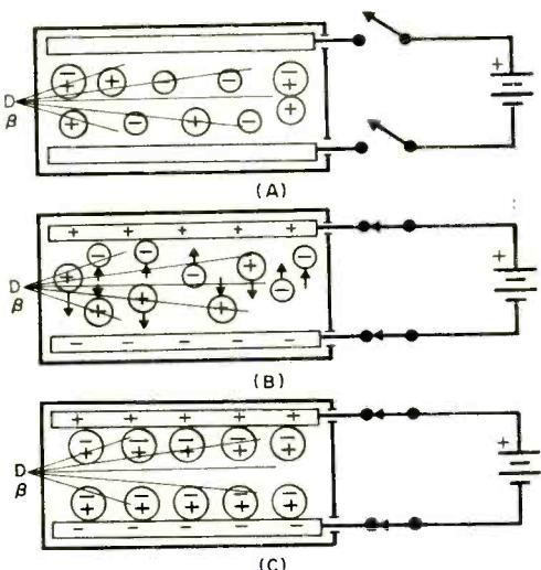
**Fig. 2. Neutralization of ions is shown.**
