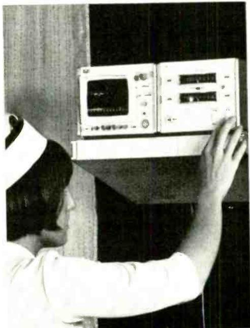
**Bedside instruments monitor the patient's ECG, heart rate, and blood pressure. (Courtesy: Hewlett-Packard)**
