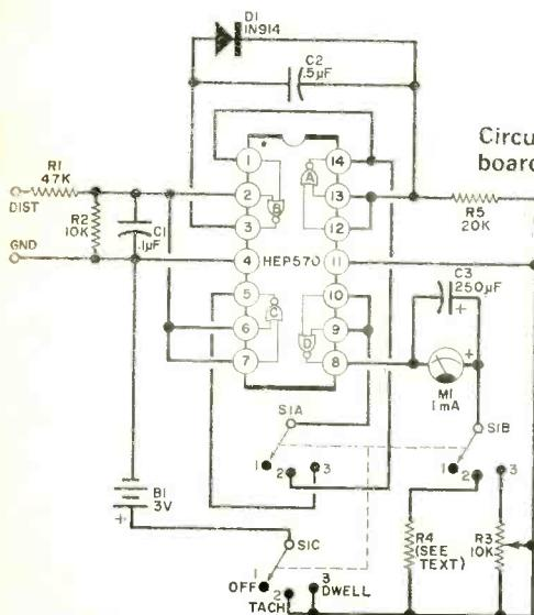
**Calibration.** To calibrate the dwell scale, Set S1 to position 3 and, with the two input leads shorted, adjust R3 for a full-scale deflection. This represents the angular distance between the lobes of the distributor can shaft; i.e. 45° for an eight-cylinder engine (60° for six cylinders; 90° for four).
