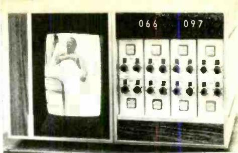
**Closed-circuit TV permits observation of patient from central station. Instruments at right monitor heart rate and blood pressure. Digital readout shows parameters for a selected patient. (Courtesy: Smith Kline Insts.)**
