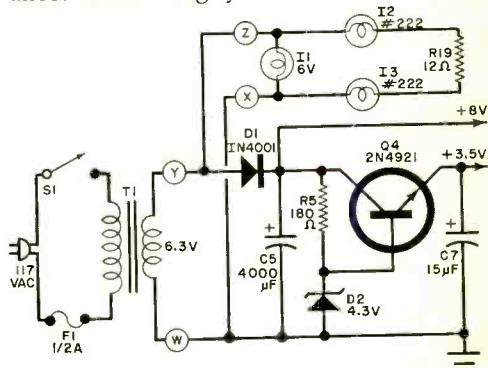
Fig. 3. Circuit for dc supply and ac supply to beam lights.
