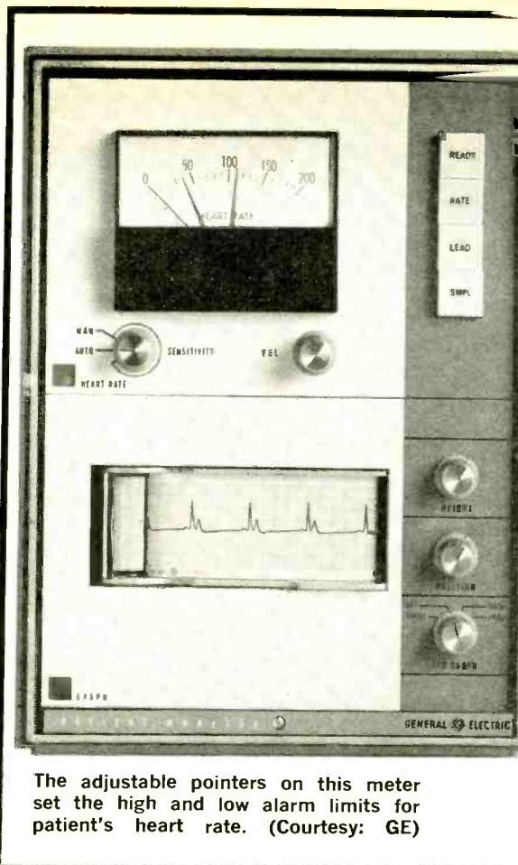
The adjustable pointers on this meter set the high and low alarm limits for patient's heart rate. (Courtesy: GE)
