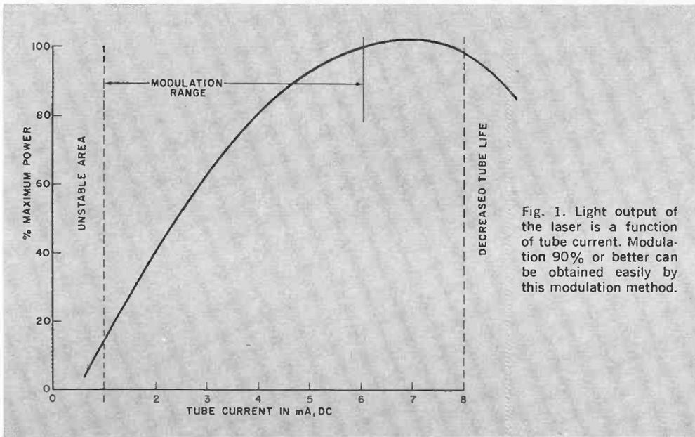
Fig. 1. Light output of the laser is a function of tube current. Modulation 90% or better can be obtained easily by this modulation method.
