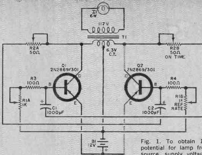
Fig. 1. To obtain 117-volt driving potential for lamp from 12-volt d.c. source, supply voltage is converted to a.c. via oscillator and stepped up.
