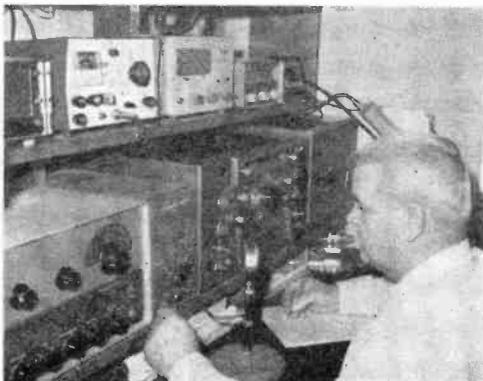
Charles Cash, W9LNC, Cayuga, Ind., is a Civil Defense Radio Officer and ARRL Emergency Coordinator. He works 80-meter CW with a Knight-Kit T-150 and National HRO and 2 meters with a Clegg 99'er as well as with a Heathkit Two-er transceiver.
