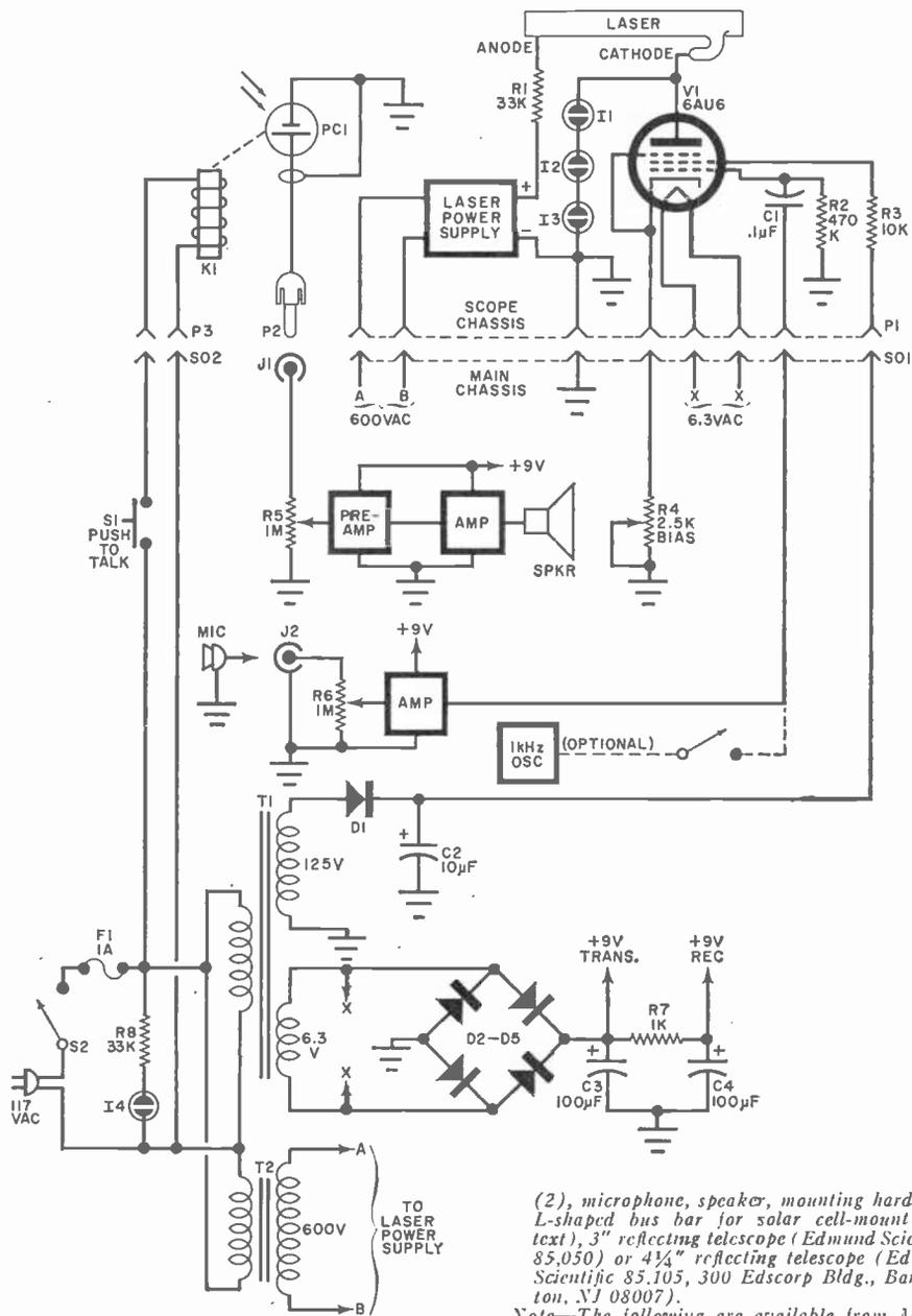
T2—Power transformer; secondary 620-650 volts at 50 mA
