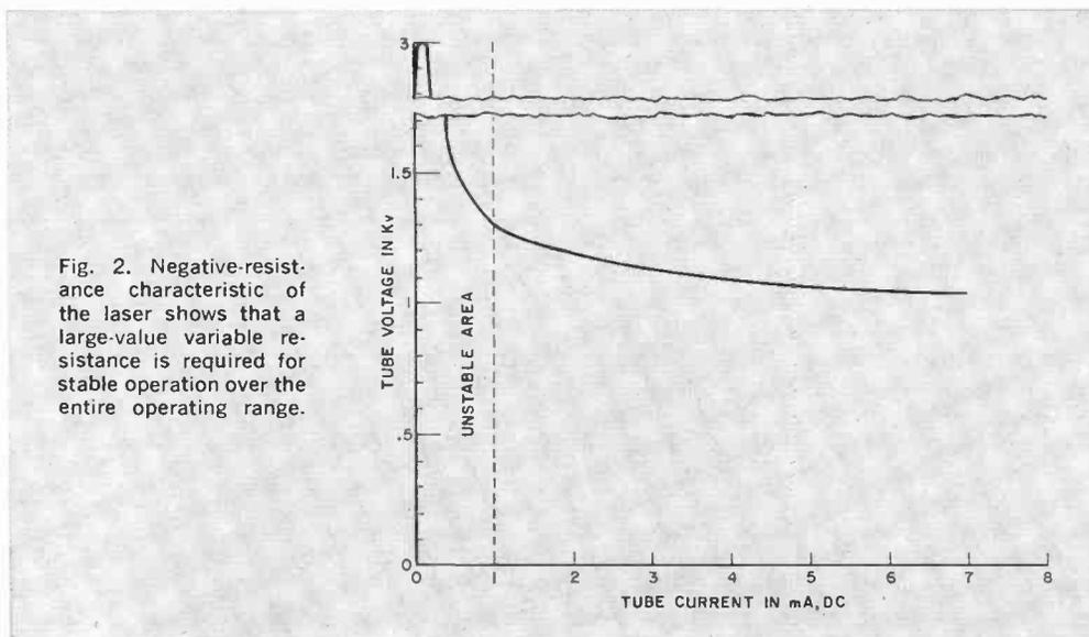
Fig. 2. Negative-resistance characteristic of the laser shows that a large-value variable resistance is required for stable operation over the entire operating range.
