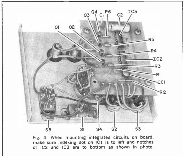
Fig. 4. When mounting integrated circuits on board, make sure indexing dot on IC1 is to left and notches of IC2 and IC3 are to bottom as shown in photo.
