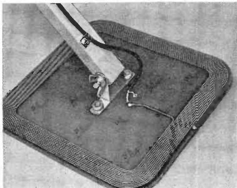
Search coil (left) is a double-sided piece of copper-clad fiberglass PC board. Top side has a coil etched out of the copper. On the bottom is a continuous band of copper connected to coax shield.
