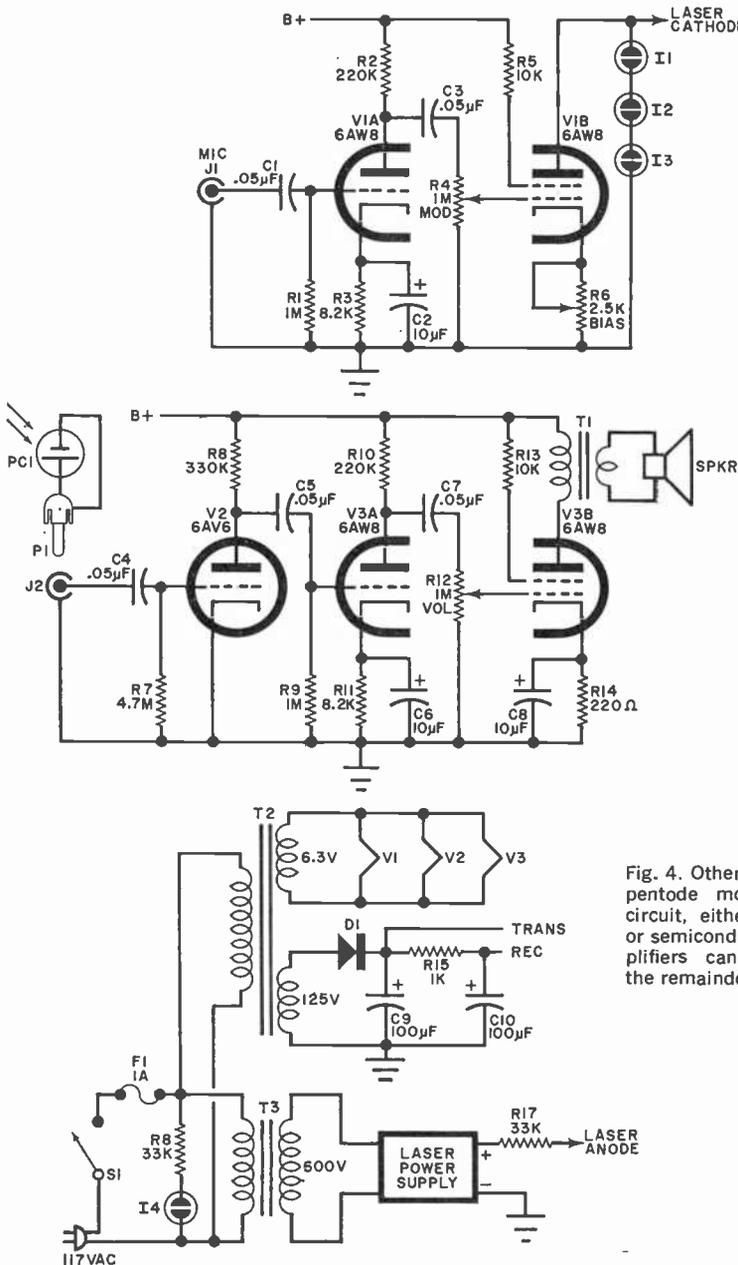
Fig. 4. Other than the basic pentode modulator ( $V1B$ ) circuit, either vacuum-tube or semiconductor audio amplifiers can be used for the remainder of the circuit.
