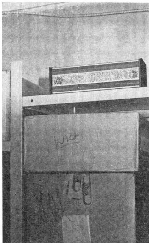
Unobtrusively set on a storeroom shelf, DeltAlert ultrasonic alarm fans 35-kHz energy out at a horizontal angle of about 100° and vertical angle of 40-45°. Used in this storeroom (a 2-car garage), it immediately sensed any "foreign" movement and energized a loud alarm bell for thirty seconds.
