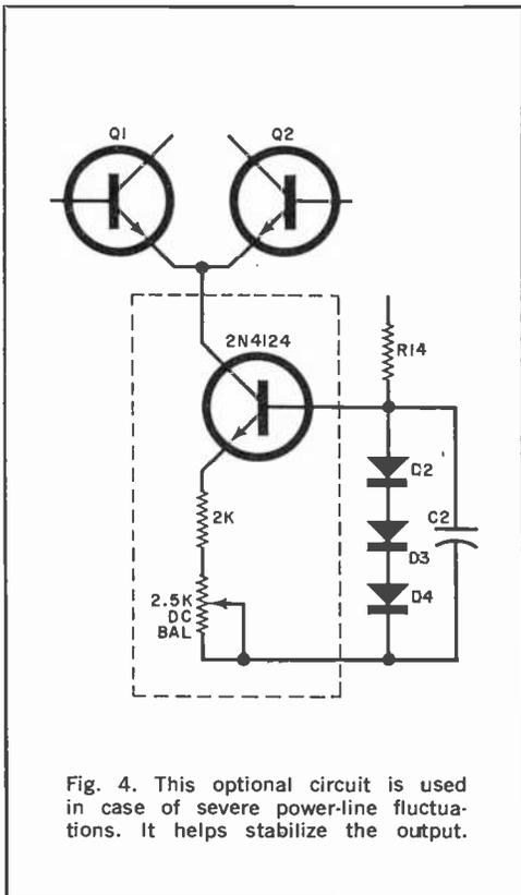
Fig. 4. This optional circuit is used in case of severe power-line fluctuations. It helps stabilize the output.
