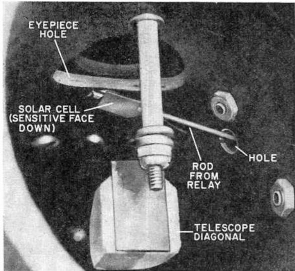
In the simple transceiver, the solar cell is mounted within a tube having a dark interior—in this case, it's a clean Polaroid print coater. Cell is affected by ambient light so that it must be shielded during use. Any method of mechanical mounting may be used to position the cell correctly.
