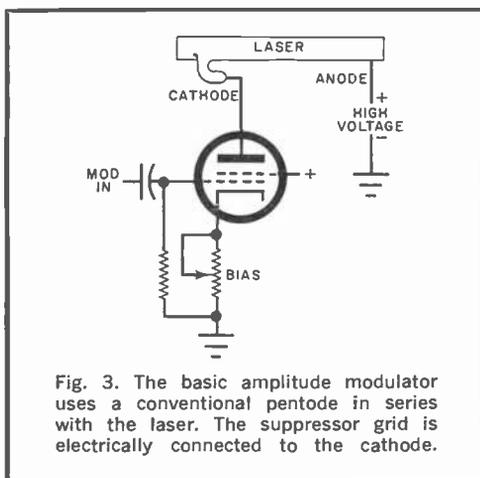
Fig. 3. The basic amplitude modulator uses a conventional pentode in series with the laser. The suppressor grid is electrically connected to the cathode.
