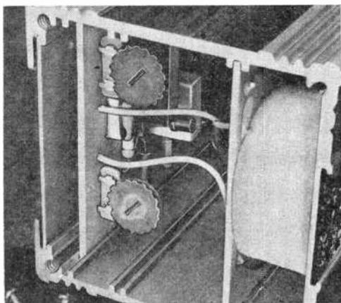
Two controls, for sensitivity (top) and time interval, are conveniently located just inside one end of the chassis. Sensitivity is easily set by connecting a lamp to the normal alarm outlet and walking back and forth through ultrasonic field. Time interval depends on the type of alarm used.
