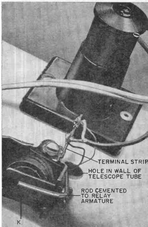
The transmit/receive relay is mounted to the telescope tube with the solar cell and rod passed inside through a hole cut in the telescope tube wall.
