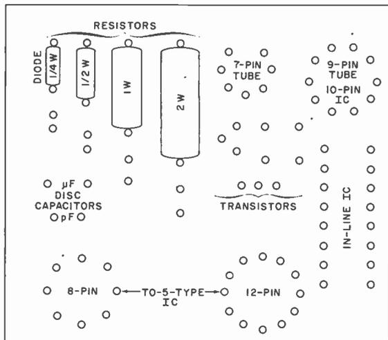
Fig. 1. Template guide, shown actual size, gives minimum hole spacing for most commonly used components. Most signal and low-current diodes fit into  $\frac{1}{4}$ -watt resistor slot; other silicon diodes fit into  $\frac{1}{2}$ - or 1-watt resistor slots. Eliminate one dot in upper right drawing for nine-pin tubes.
