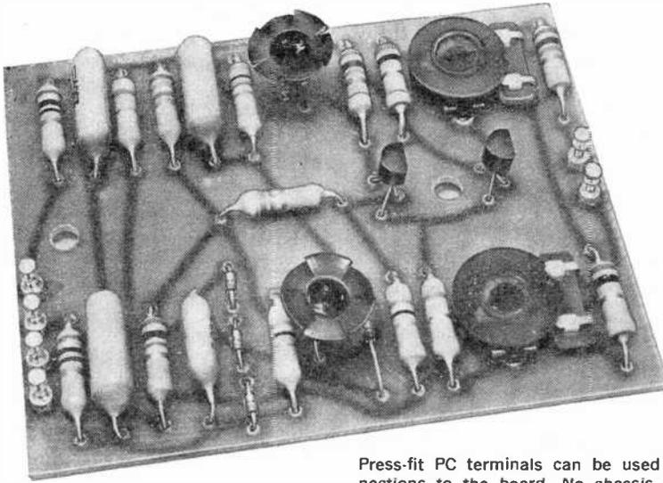
Press-fit PC terminals can be used to make connections to the board. No chassis is shown here because board is designed to be mounted in an existing single-wave generator and get its d.c. power either from the generator supply or a built-in source of +18 and -18 volts. The squarer can be switched in through a switch on the front panel.
