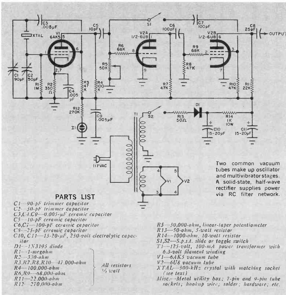
*R5* set at approximately mid-range, an uncontrolled oscillation of about 50 kHz is obtained. However, by injecting the 500-kHz signal from *V1* into the multi-vibrator, a very stable 50-kHz signal appears at the output.
