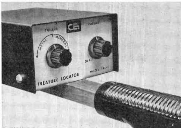
Knob at left (above) controls beat note frequency and offers some indication of "type" of detected substance. Other knob controls volume and on/off switch. Earpiece connection is on back of the box.
