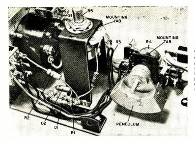
Wiring and assembly Is open but very rigid. The pendulum must have room to swing freely. The shaft of zero-G setting potentiometer R5 is accessible through a hole in cover of the metal box.
