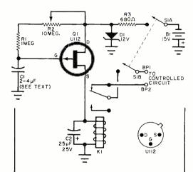
Almost any p-channel FET similar to the recommended U112 can be used. A type n-channel may work if the polarities are reversed.
