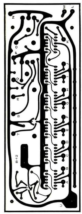
Fig. 2. Actual-size printed-board foil pattern layout. Because of circuit complexity, such a board is necessary to avoid troublesome wiring errors.
