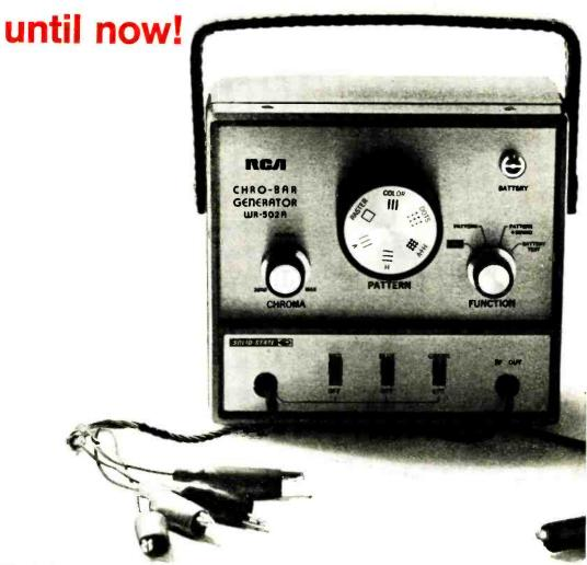
The RCA WR-502A CHRO-BAR color-bar generator is all solid-state, battery operated... Provides color bars, dots, crosshatch, vertical lines, horizontal lines, blank raster... has rock-solid stability. It's the greatest yet. The CHRO-BAR. \$168.00\*. RCA Electronic Components, Harrison, N.J.
