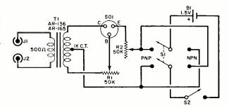
St., Arleta, Calif. 91311. Although it does not permit quantitative measurements, it can be used to find out if a transistor provides modest gain and will reject open, shorted, excessively leaky, and very lowgain units. The instrument could be quite valuable for quick checks of bargain or lowcost "surprise package" transistor purchases.
