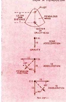
All forces acting on the pendulum mass act on its center of gravity, which is eccentric with respect to its pivot point. The lever arm is the distance from the pivot point to the center of gravity and transmits the force acting on the center of gravity to the pivot in a rotational manner.
