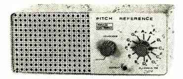
The completed Pitch Reference can be dressed up by using a commercially available dialplate (see Parts List). The cover should have one or two one inch holes at the rear to prevent any cabinet resonances.
