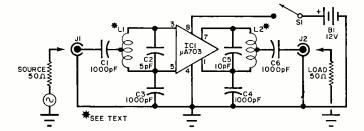
Fig. 3. Believe it or not, the circuit shown here will amplify signals up to 200 MHz. The secret is the specially designed Fairchild type  $\mu$ A703 linear IC.
