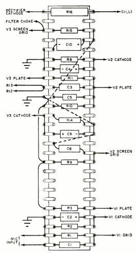
Fig. 3. Use of a terminal board or tag strip speeds assembly and lends a neat, professional appearance.
