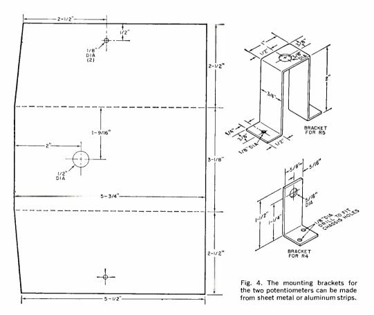
Fig. 3. The cover forms a cowl over the front panel. If desired, the front can be cut in a straight line.
