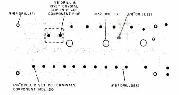
Fig. 3. Drill the PC board as shown here. The three largest holes mount the filter capacitors' standoffs. The use of PC terminals is optional. They are not supplied with the kit.
