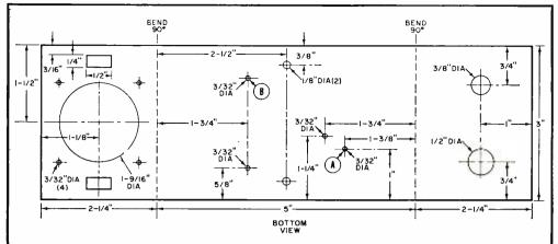
Fig. 2. The author bent a chassis and cover out of sheet metal. The bending, drilling, and cutout information is shown above. The two slide switches are soldered to the rear of the front panel.
