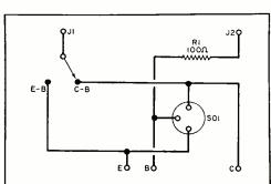
Containing only a resistor and a mounting socket, the circuit can be used to test pnp or npn transistors, in or out of use.
