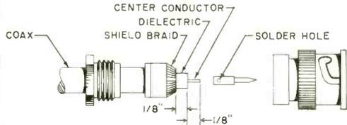
place it with a UG-1094A/U BNC connector. Replace the fitting on the test cable with a UG-88/U BNC connector (see drawing). Since the shorting switch in some VTVM probes can be erratic on the low resistance range, it is a good idea to make a straight-through test cable for this function, using a UG-88/U BNC connector, a length of RG-58A/U, and two alligator clips.
