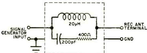
generator used should have the impedance of a typical antenna. If it does not, then a series impedance should be added so that it and the internal impedance of the generator will match the receiver input.
