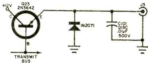
been added and is connected from the emitter of Q23 to ground. See diagram. The parts needed for the various changes are available from most radio distributors.
