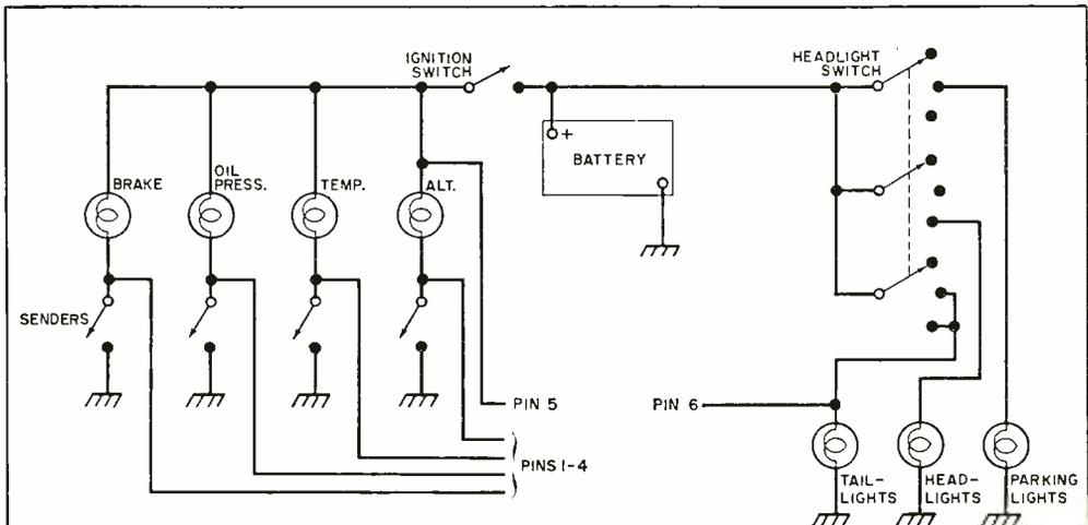
Fig. 3. Typical warning light wiring used in most American cars. The senders (except for brakes) are mounted somewhere on the engine. Make sure that pin 6 goes to the taillight connection.
