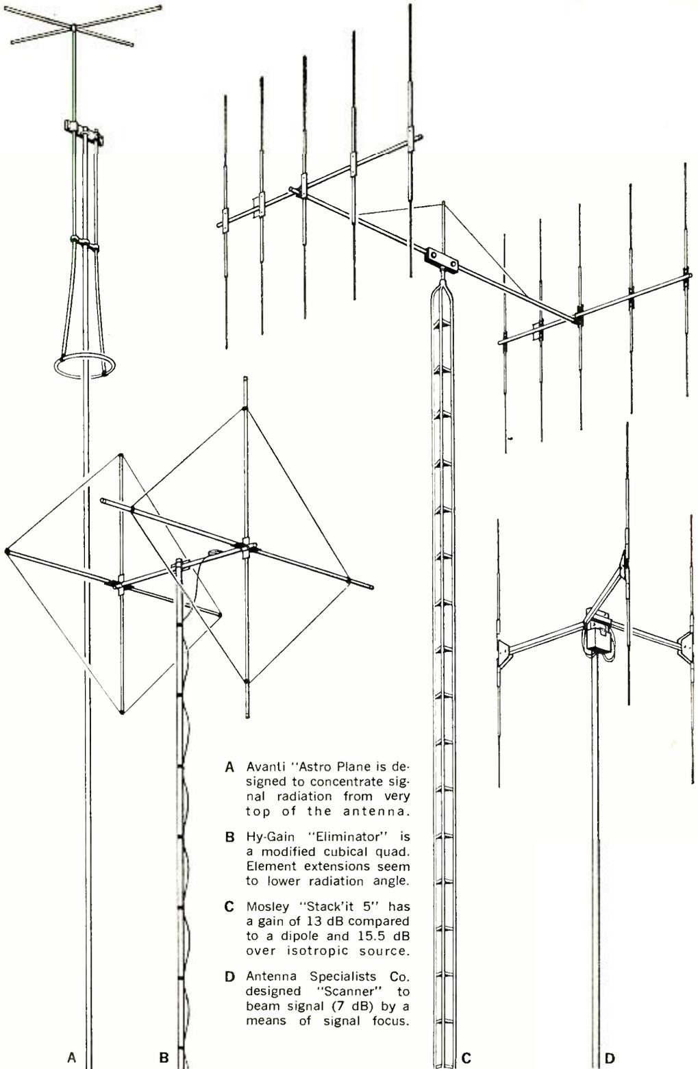
**A** Avanti "Astro Plane" is designed to concentrate signal radiation from very top of the antenna.
