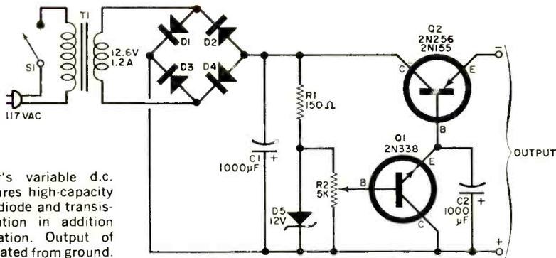
Fig. 1. Bill Lahr's variable d.c. power supply features high-capacity filtering and zener-diode and transistor voltage regulation in addition to bridge rectification. Output of power supply is isolated from ground.
