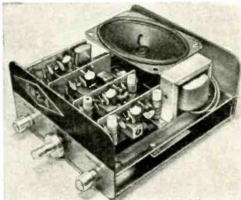
Not visible in this closeup photo are the i.f. and audio stages under the miniature speaker. Transformer is for 117-volt a.c. supply, but receiver may be operated from a 12-volt d.c. car battery.
