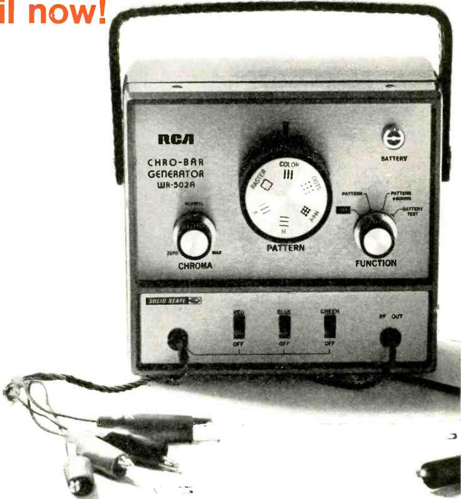
The RCA WR-502A CHRO-BAR color-bar generator is all solid-state, battery operated... Provides color bars, dots, crosshatch, vertical lines, horizontal lines, blank raster... has rock-solid stability. It's the greatest yet. The CHRO-BAR. \$168.00\*.
