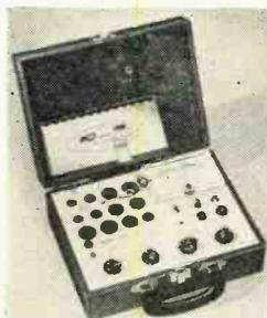
plished with the *B & K Model 606 "Dyna-Jet"* tube tester. It checks for shorts, grid emission (in a unique 100-megohm sensitive circuit), leakage, gas, and cathode emission under simulated load conditions for more accuracy. Each section of multi-section tubes is checked. The Model 606
