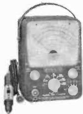
**V-70 VACUUM TUBE VOLTMETER KIT:**
