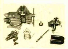
Vises, like other tools, are made in different sizes to suit different work. A spring clip, forced into the end of a bottle cap or a solder reel, makes a good emergency vise for light holding jobs. A magnet can also serve at times as a third hand.
