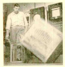
**Drop test** checks the packaging. It's important because set quality doesn't mean much unless the product can safely survive the rigors of shipment.
