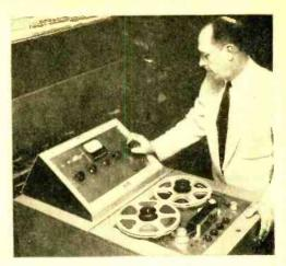
Martin Bender, designer of the console, adjusts output level control during test. Below, bottem view of console, showing how tuning-fork amplifier hinges out for easy accessibility. Smaller amplifier sitting on shelf is used for monitoring.
