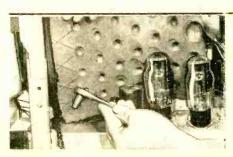
Easy ratchet movement—plus the offset angle of this tool—is a big help when you have to turn a screw or nut in a half-hidden corner. The rubber pad in background is used to protect TV tube from accidental slips.
