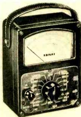
Instrument's nineteen ranges include: 6 d.c. voltage ranges to 5000 volts; 6 a.c. voltage ranges to 5000 volts; 3 resistance ranges to 200 megohms; and 4 d.c. ranges to 10 amperes. Supplied complete with all parts, a pair of 4-foot test leads, and complete instructions, this v.o.m. kit is available at \$26.50 f.o.b. Chicago. For full specifications, or to order, write to *Allied Radio Corporation*, 100 N. Western Avenue, Chicago 80, Illinois.
