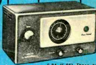
**S-94 (S-95)** These two new Clivc Patrol receivers are over 10 times as sensitive as previous models, greater increased audio power output and built-in relay squelch system. Perfect for monitoring, police, fire, taxicab, telephone-mobile, forestry, Civil Defense. The S-94 covers 30-50 Mc and the S-95 150-173 Mc. Built-in speaker and provisions for headphones. Eight tubes plus rectifier. 105/125 V. 50/60 cycle AC/DC.
