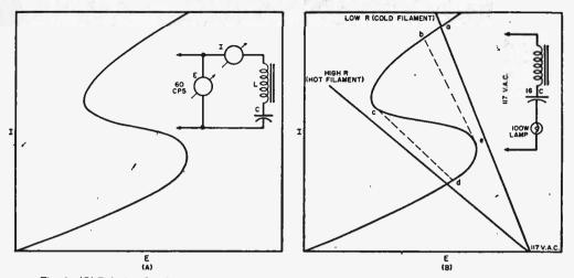
Fig. 1. (A) Relationship between current and voltage with a saturable inductance in series with capacitor chosen. See text. (B) Series circuit of L and C with tungsten filament lamp added. Load lines corresponding to hot and cold resistance values are indicated.
