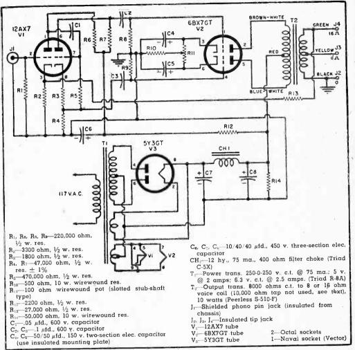
Fig. 4. Complete schematic of the 4-watt amplifier. It may be operated from most tuners and preamplifiers and provides adequate output for ordinary home listening.
