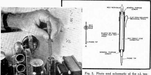
Fig. 2. Photo and schematic of the r.f. tester for hams. Use it to check for presence of r.f. energy in oscillators and amplifiers.
