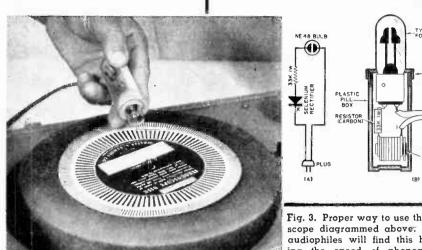
Fig. 3. Proper way to use the 60-cycle stroboscope diagrammed above. Technicians and audiophiles will find this handy for checking the speed of phonograph turntables.
