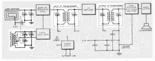
Fig. 1. Basic receiver adjustments (dotted boxes) that a layman can make. See text.
