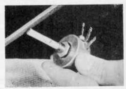
Any saw burrs on the new shaft should be filed off. Wires may be shifted one at a time from old to new control or a sketch of the original wiring may be made before removal of control.
