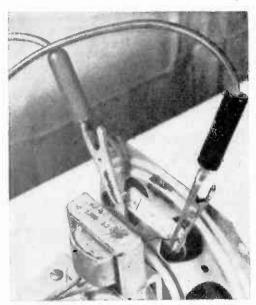
Fig. 4. How a multitester can be connected across the loudspeaker voice coil terminals.
