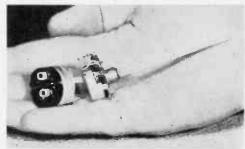
Most radios and TV sets have "on-off" switch attached to and operated by the volume control shaft. The switch section fits over back of control after the cover plate has been removed.
