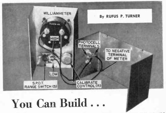
high position of this switch, the photocell is connected directly to the milliammeter (M). Very little light then is required for full-scale deflection. In its low position, the 1000-ohm radio volume-control-type rheostat (R) is switched in series with the cell and meter, so that higher illumination levels can be accommodated by the same meter.
