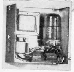
FEW CENTS a year pays for the power A this alarm consumes while standing guard duty. It is intended for power-line operation and draws approximately 50 milliwatts (.05 watt). Simply as a comparison, this unit could be operated continuously for 1000 hours yet cost no more than operating a standard 60 watt electric light bulb for one hour.
