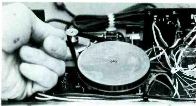
**Step 4.** The motor pulley drives a rubber belt (usually flat). The belt wraps around and spins the heavy, speed-smoothing flywheel. If the belt is dirty, worn, or stretched, it can slip on the motor pulley and allow slow or erratic tape movement. Severe looseness might prevent the belt from turning the flywheel at all. If the belt is dirty, clean it with isopropyl alcohol. If it's worn or stretched, replace it.
