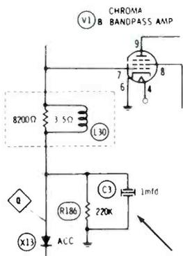
plate and screen voltages changed from about +150 volts without signal to approximately 50 volts with color.
