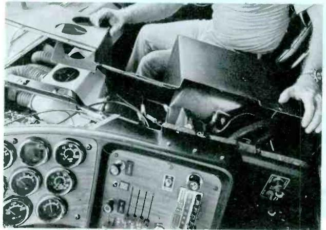
Fig. 3 Remove the self-tapping screws that hold the cover to the console. For total access, unclip the air-conditioner vents, and remove the cover. This allows you to trace good paths for the antenna and power cables, drill the holes and install the grommets, before replacing the cover.
