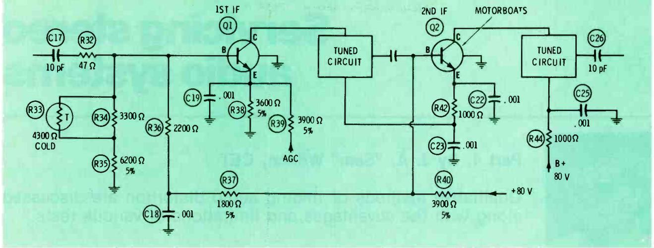
**Fig. 4** This partial schematic of the IF stages in RCA CTC38 chassis shows both transistors are in series with the supply voltage, and the bases come from a common voltage divider. A leaky 2nd IF transistor causes a motorboat of the video.
