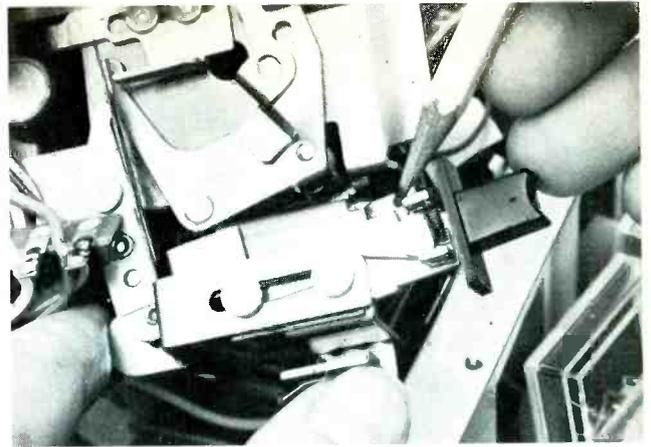
**Step 18.** A latching assembly catches the pause slide and holds it in the pause position. But when you push the Pause button again, the mechanism releases the slide, allowing all assemblies to return to whichever mode the unit was in. If the pause slide doesn't latch or release properly, check the latching assembly. Make sure it's free of caked lubricant and grime, and that its springs haven't slipped out of position or broken.
