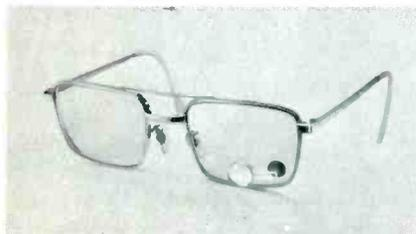
A product of **MecLab**, the loupe consists of a 11-millimeter lens with a swivel ball joint and soft mounting cup. The ball joint permits the lens to be positioned parallel to the glasses, giving best sharpness and least distortion. The loupe can be mounted in a bifocal area where it does not interfere with distant vision.
