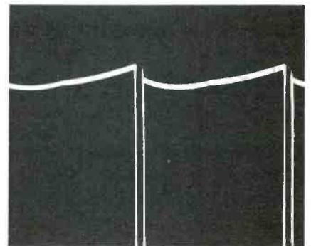
Fig. 11 A rounded sawtooth waveform between pulses can be seen at the collector of Q1, if the scope gain is increased enough to deflect the tips below the bottom of the screen. Most of the pulse amplitude is in the cut-off region of both Q2 and Q3, therefore Q3 amplifies the tiny sawtooth that actually reaches its base. Any deviation from the desired yoke-current waveform changes the shape of the small sawtooth at the base of Q3, and corrects for any non-linearity.
