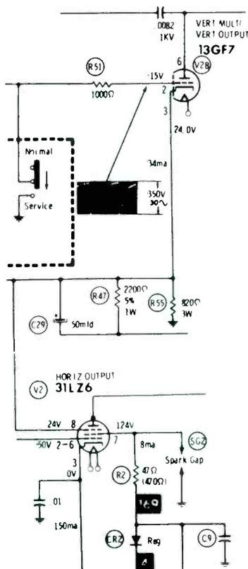
During the last inspection, I carefully checked the schematic and discovered that the cathode of the vertical-output tube was connected directly to the suppressor grid of the 31LZ6 horizontal-output tube. Remembering the charred R47, I
