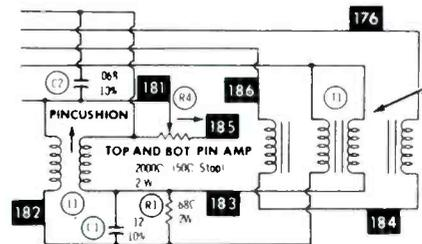
I removed the convergence board, convergence yoke, and also the cover of the deflection yoke. With the power on, I moved components and connections, using a plastic rod, and soon located where the pincushion transformer had broken loose from the circuit board. A quick soldering of the transformer connections, replacement of the components, and the repair was completed.
