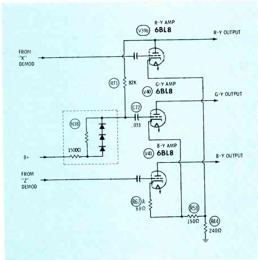
Fig. 6 A new type of matrixing is used in the production of the G-Y signal in Philco's 21ST90 chassis.
