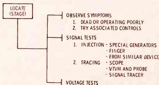
Fig. 6 Step Two of 1-2-3-4 Servicing
