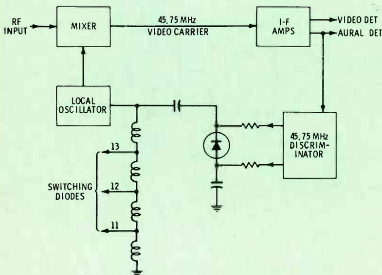
Fig. 3 The basic automatic-fine-tuning (AFT) loop.
