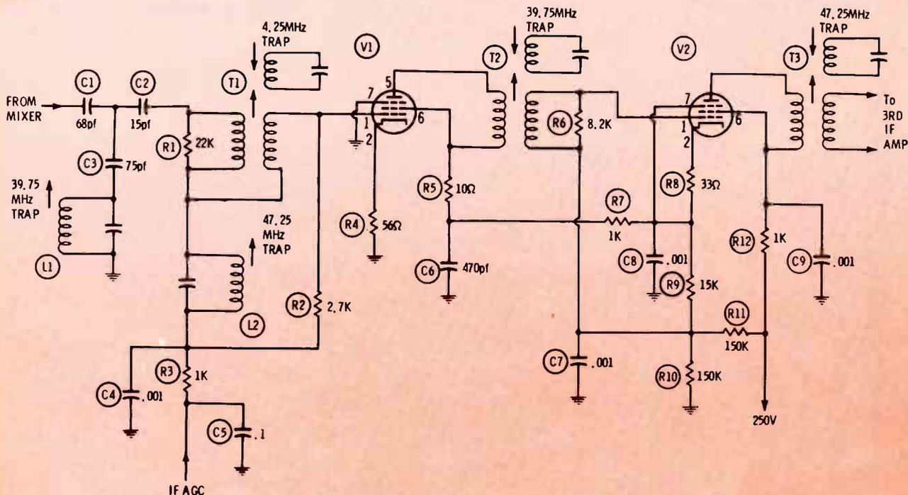
Fig. 4 Part of stagger-tuned IF strip that is used in many TV brands and models. This one is "B+ stacked" version, in which two tubes are in series across B+ line. Cathode and grid of V2 have high positive voltages.
