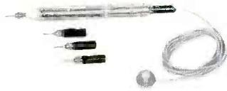
Gain 3000 at 2 KHz. Bandwidth 50 Hz to 200 MHz. Z 3500 $\Omega$  to 350 K $\Omega$ . Output 0.3 p-p volts. Noise -45db. Supplied with anti-overload probe tips: Eico PST-2, Kit \$19.95, Wired \$29.95.
