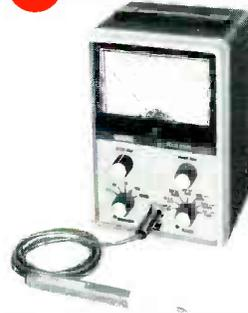
AC RMS/DCV: 0-1, 3, 10, 30, 100, 300, 1000V. P-P ACV: 0-2.8, 8.5, 28, 85, 280, 850, 2800V. DC Input Z 11 M $\Omega$ . Ohmmeter 0.2 $\Omega$  to 1000 M $\Omega$ . 4 1/2" 200  $\mu$ A meter. Eico 240, Kit \$59.95, Wired \$79.95. With 6 1/2" meter & AC/DC Current readings.
