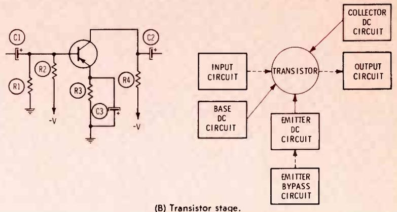
**Fig. 3** Circuits in typical amplifier stages. Other signal circuits include feedback circuits, tuned circuits. Bypass circuits are often called decoupling circuits.
