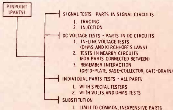
Fig. 8 Step Four of 1-2-3-4 Servicing.
