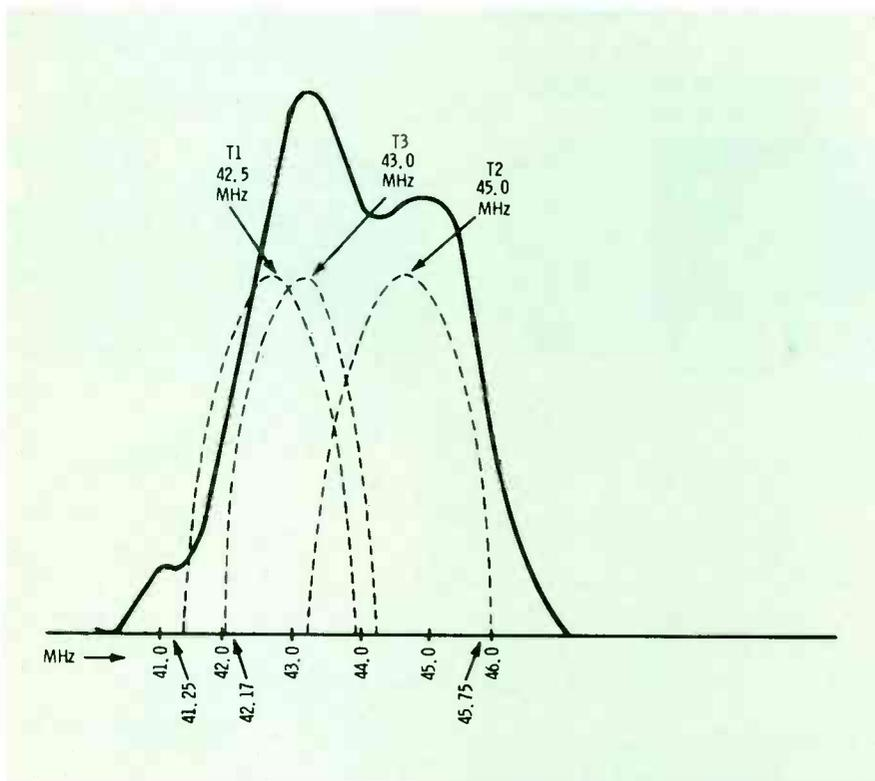
**Fig. 5** Individual responses of stagger-tuned IF transformers combine to form IF response curve. Heavy line is the net response traced at all frequencies in the IF passband. It is the same curve you see traced by the sweep generator and scope in Fig. 3B.
