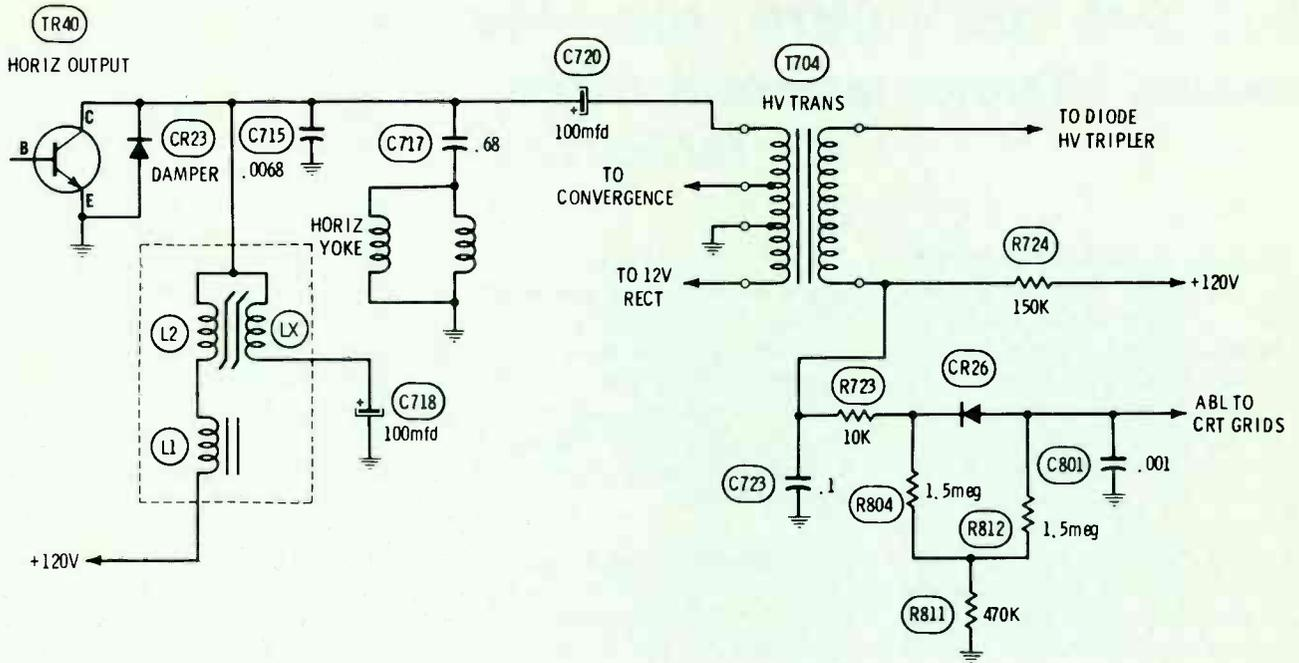
**Fig. 15** Hitachi models CFA-450 and CSU-690 employ a saturable-core reactor as the high-voltage regulator. CRT current through the high-voltage tripler determines the amount of bias supplied the CRT by the automatic brightness limiter (ABL) circuit.
