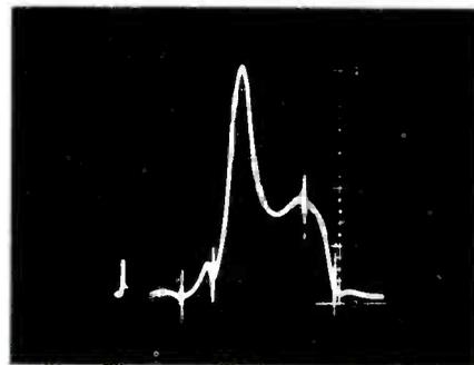
**Fig. 6** This is what the response curve of Fig. 3B would look like with decoupling capacitor C7 open; degeneration isn't quite as bad as with C6 open (Fig. 3A).
