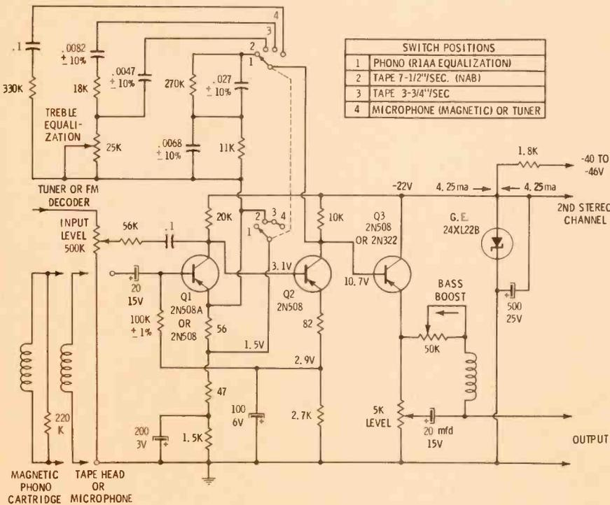
**Fig. 6** Typical solid-state preamplifier circuit.
