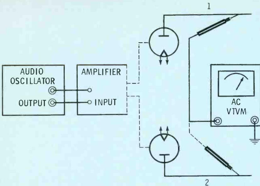
Fig. 2. Test setup for checking AC balance.
