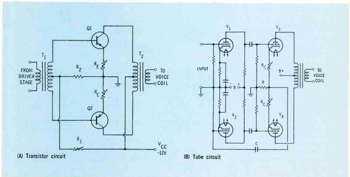
Fig. 1 Basic transistor—and tube-type push-pull circuits.
