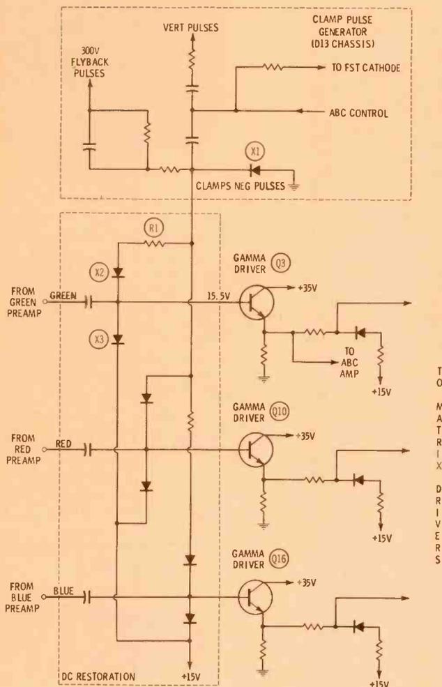
Fig. 5 Schematic of DC restoration circuit.
