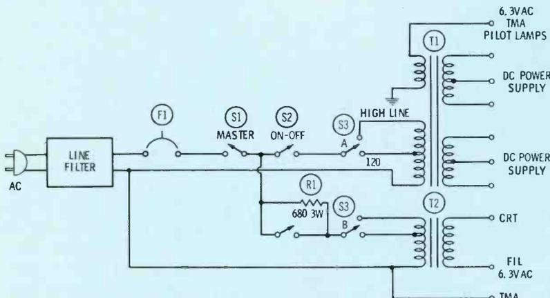
Fig. 11 Schematic of the switching circuitry that permits the CTC40 to take advantage of the "instant-on" characteristics of semiconductors.
