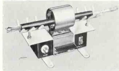
The circular radiant heating elements are energized with a switch and their heat intensity is regulated by a solid-state device. The semi-circular halves of the heat tunnel are closed and locked by depressing a handle. The cylindrical working area inside the heat tunnel is 3" in diameter by 4" long. The heat tunnel shield is gold-fired for maximum heat reflectivity. Height-adjustable, V-shaped, plastic-covered guides center and support the work as it passes through the heat tunnel.
