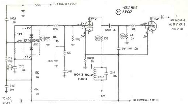
must have a scope. I would suspect that either capacitor C46 or C65 is defective; however, you can prove this only through waveform analysis.
