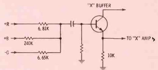
Fig. 9 Matrix circuit for X signal.
