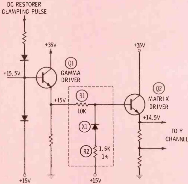
Fig. 6 Gamma correct circuit (blue channel).
