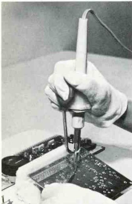
For desoldering, the unit is held as illustrated in the photo; the rubber bulb is depressed with the index finger. As the solder melts, a sudden release of the bulb draws the melted solder into the reservoir. The old solder is ejected by rapidly compressing the rubber bulb. To replace the solder, use the unit as you would a conventional soldering iron.
