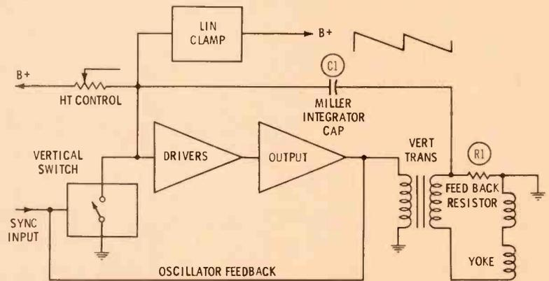
Fig. 4 Illustration of the fundamental sweep system employed in the CTC40.
