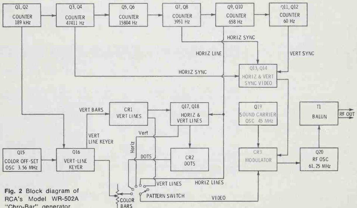
Fig. 2 Block diagram of RCA's Model WR-502A "Chro-Bar" generator.
