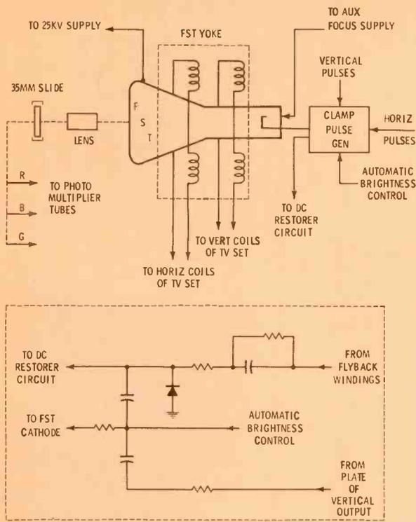
Fig. 3 Circuits associated with the flying-spot scanner.
