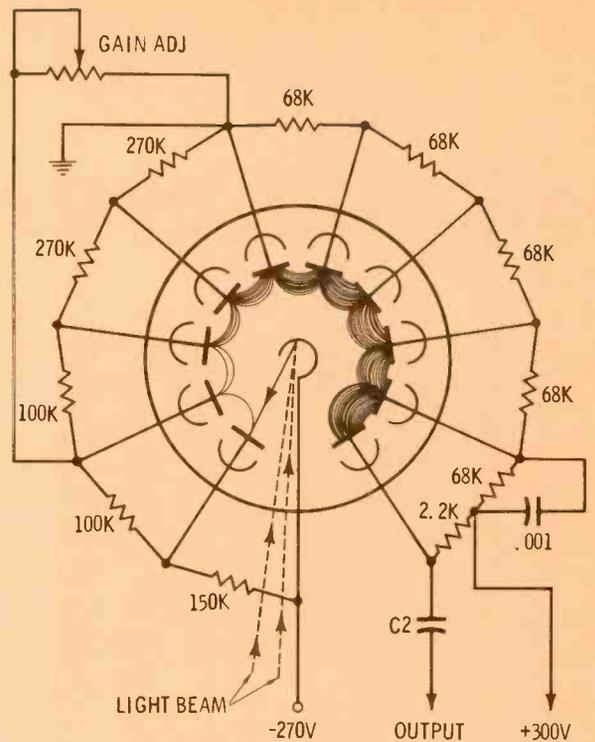
Fig. 4 Diagram of photo-multiplier tube.
