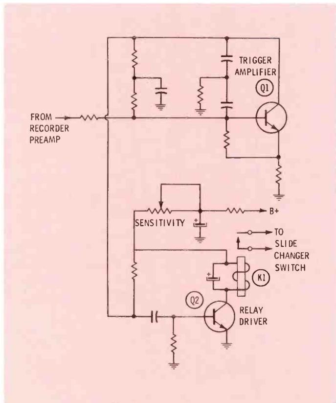
Fig. 12 60-Hz "beep" circuit generates signal for automatically changing slides.
