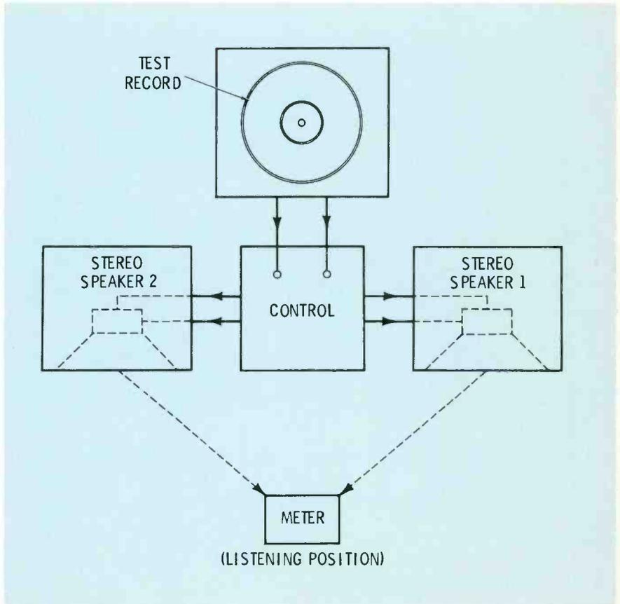
Fig. 8 Test setup for checking the balance of a stereo system.
