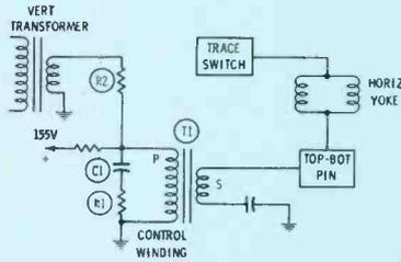
Fig. 10 Side pincushion correction is accomplished by amplitude modulation of the horizontal deflection current.
