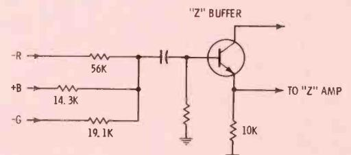
Fig. 10 Matrix circuit for Z signal.
