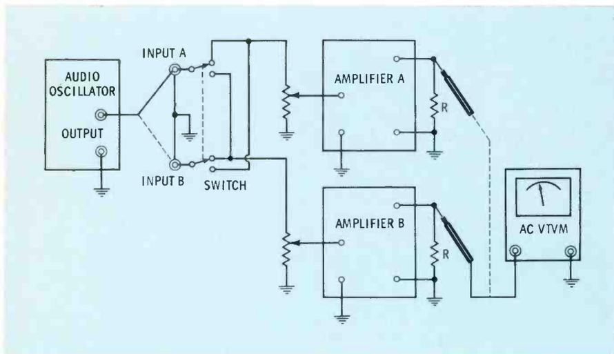
Fig. 9 Checking crosstalk between stereo amplifiers.
