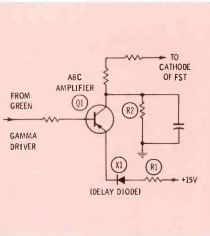
Fig. 11 Automatic brightness control (ABC) circuit.
