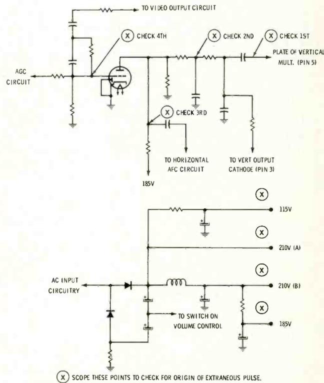
Your description of the problem indicates that an extraneous pulse is causing a change in the operation of the vertical stage. Further waveform analysis should uncover the origin of this pulse. It could be originating in either the sync of the low-voltage power supply circuits. I personally would suspect, and this is an educated guess, the power supply as the source of the extraneous pulse. ▲
