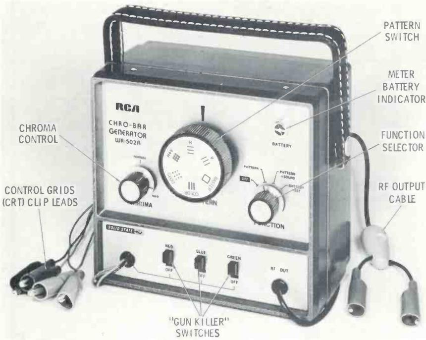
Fig. 1 RCA Model WR-502A color-bar generator.
