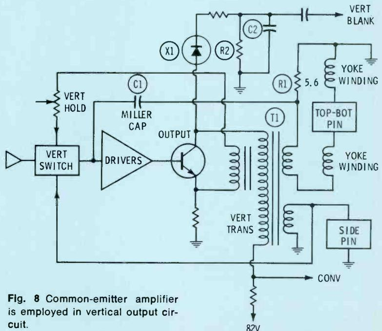
Fig. 8 Common-emitter amplifier is employed in vertical output circuit.
