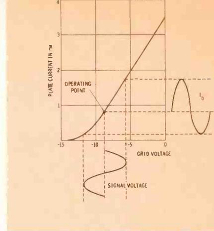
Fig. 13 Compression of the negative half cycle.
