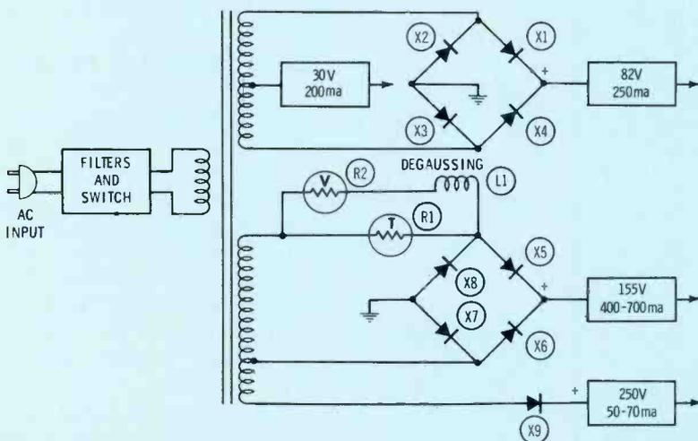
Fig. 12 Three separate rectifier circuits provide the CTC40 with four separate DC sources.
