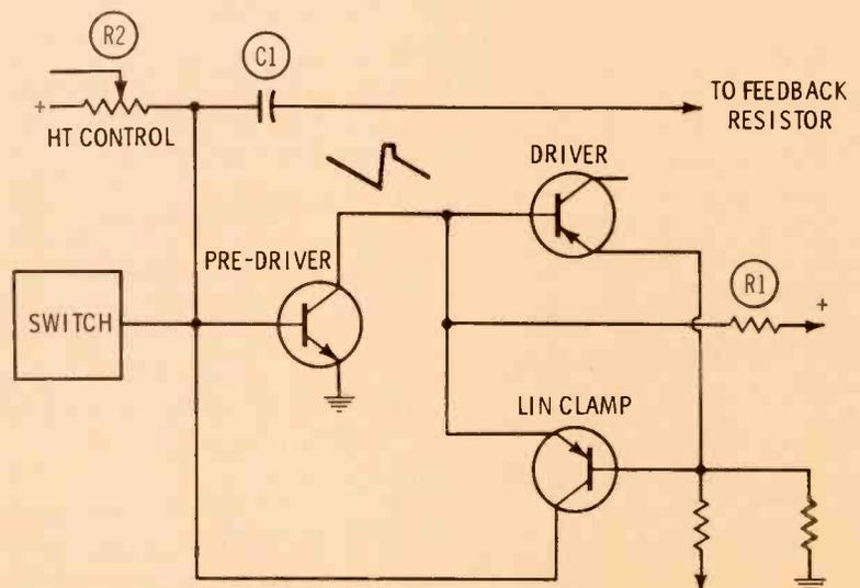
Fig. 6 Schematic showing basic circuitry of linearity clamber stage.
