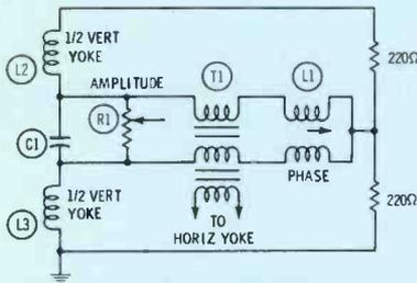
Fig. 9 Top and bottom pincushion correction circuitry.
