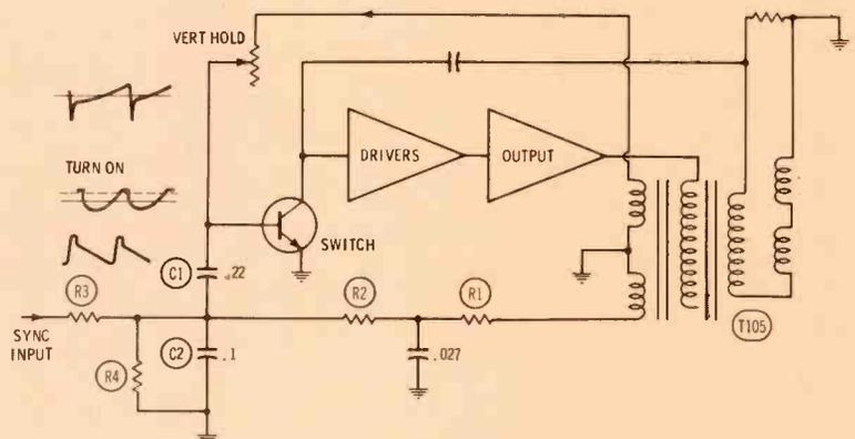
Fig. 5 Partial schematic of the vertical switch and associated circuitry.
