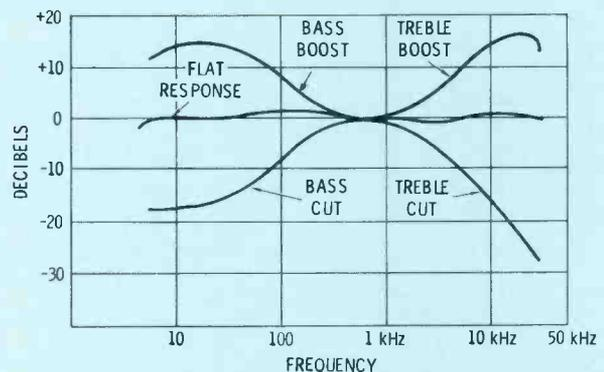
(B) Flat response, with added curves showing the effect of bass and treble controls
