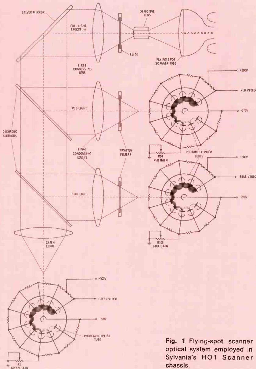
Fig. 1 Flying-spot scanner optical system employed in Sylvania's HO1 Scanner chassis.
