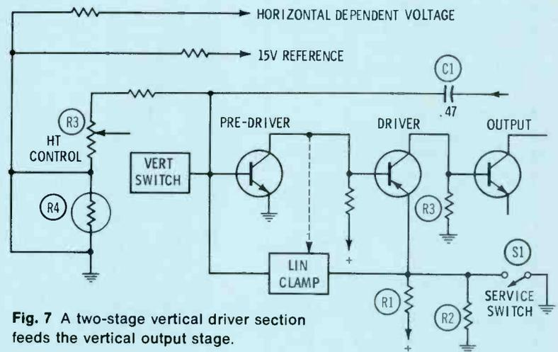
Fig. 7 A two-stage vertical driver section feeds the vertical output stage.
