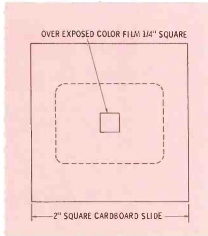
Fig. 14 Illustration of "window" test slide.
