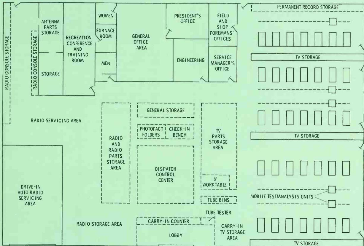
**Simplified floor plan** for Sperry TV. The concrete block building is a "free span" design having no internal supports or columns. This permits maximum use of available floor space and makes it possible to rearrange the layout without expensive and time-consuming removal and reconstruction of permanent interior walls. Outside dimensions of the building are 70' 8" x 120'.
