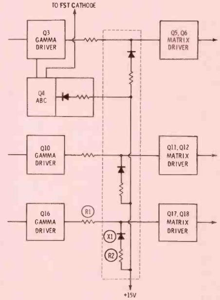
Fig. 7 Block diagram of gamma correction network (all channels).
