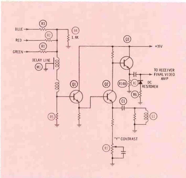
Fig. 8 A matrix circuit consisting of R1, R2, R3, R4 and R5 add red, green and blue signals to produce the Y signal.
