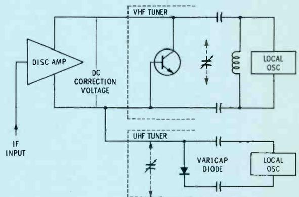
**Fig. 2** Simplified illustrations of the CTC40 AFT system.
