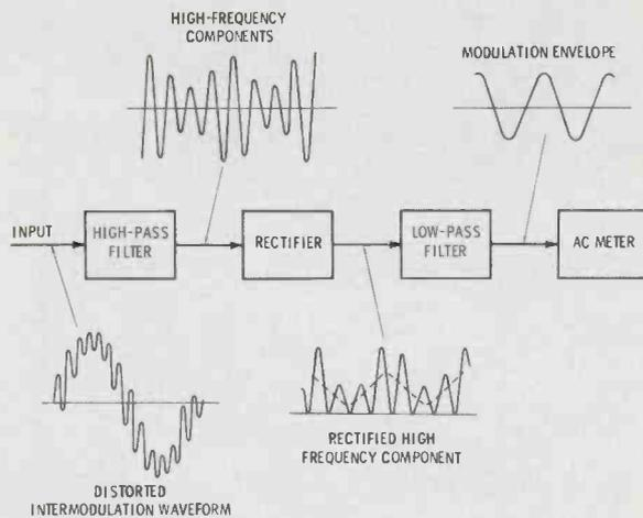
**Fig. 17** Characteristics of the filters in a typical intermodulation distortion analyzer.
