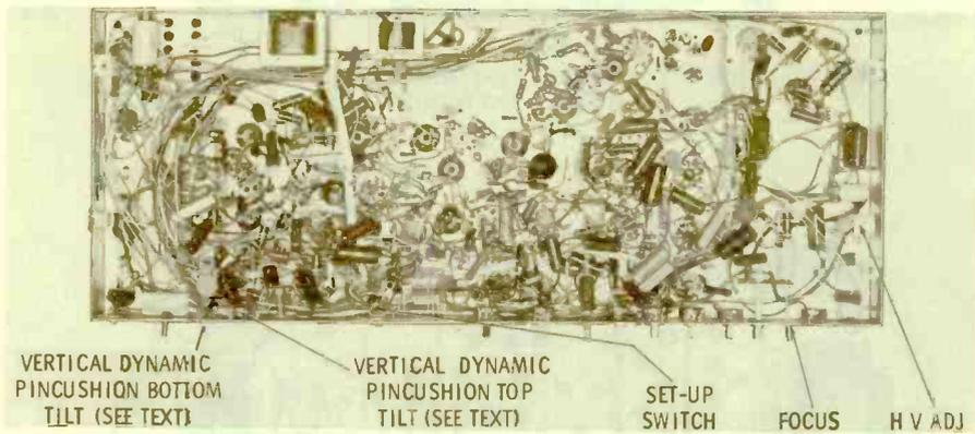
Static convergence is accomplished in the usual manner, except that disc magnets are rotated for center-dot convergence and two pincushion tilt adjustments are provided on the chassis. The "vertical dynamic pincushion bottom tilt" control straightens the horizontal line at the bottom of the screen; the top tilt has the same effect at the top of the screen.
