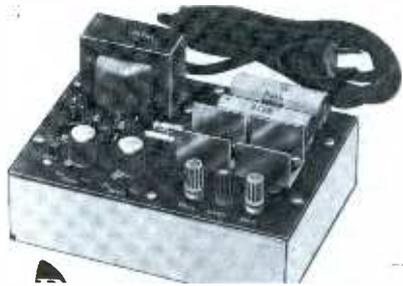
The instrument, intended for use by transistor circuit designers and experimenters, requires a maximum input of 100 watts at 117 volts, 60 cps. The **Buckeye Stamping Co.** Model PS-100 measures 7" x 5" x 4", weighs 2½ lb, and sells for \$49.95.
