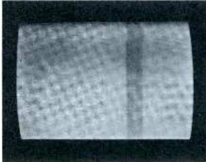
No raster when set is first turned on. Rotation of hold control produces dim raster; two pictures are obtained. Further adjustment of hold control gives sloping bars. Oscillator is running at approximately 1/2 normal frequency; loud whine can be heard. AFC is ineffective.
