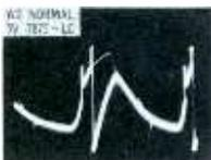
Presetting scope to exactly 7875 cps is valuable aid in troubleshooting oscillator suspected to be at wrong frequency. W5 looks almost normal, but single pulse means oscillator is at 1/2 correct frequency. W2 sync looks normal, but sample pulse occurs only with every other sync pulse (see accompanying normal W2). Waveforms show sync stages are okay and trouble is in either AFC or oscillator circuit.
