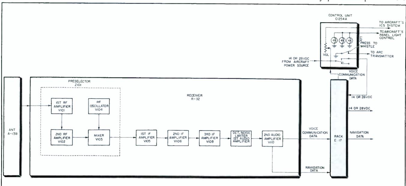
Fig. 1. Block diagram of a continuously tuned VHF-AM superheterodyne aircraft receiver.
