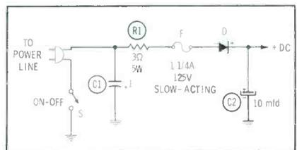
Fig. 3. Peak-limiting resistor in supply filter.
