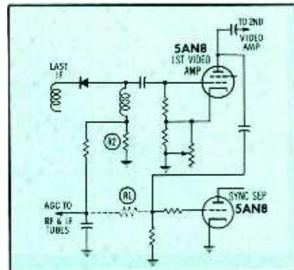
Fig. 4. Adding resistor in circuit helps prevent video overloading from strong signals.
