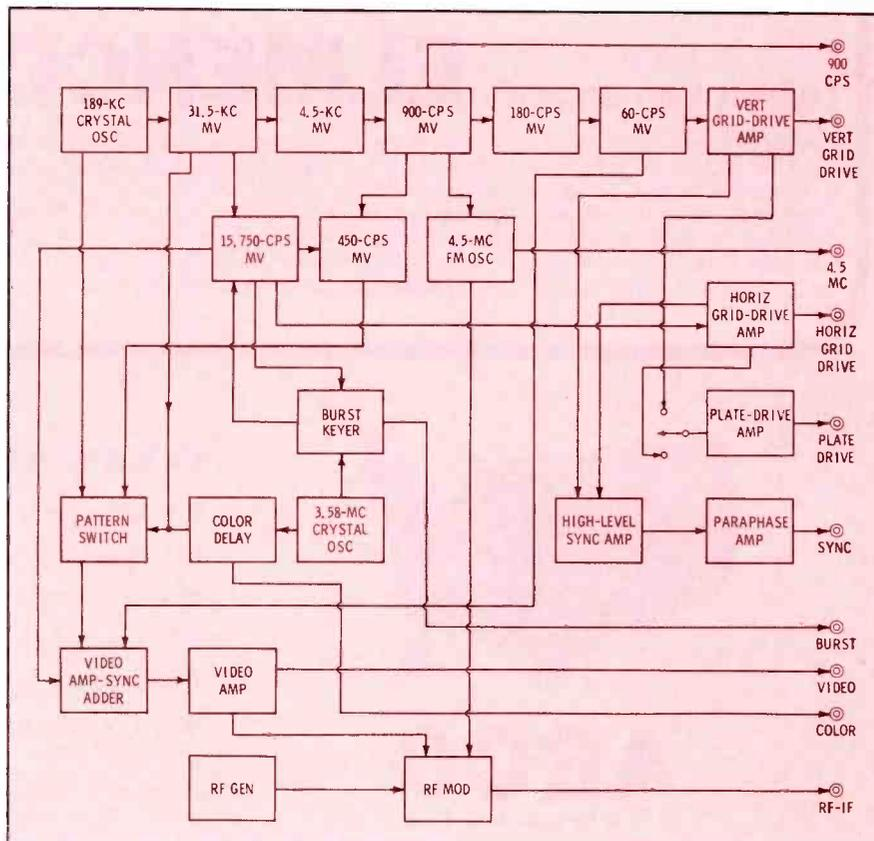
Fig. 2. Simplified functional diagram shows how signals are generated in B & K 1074.
