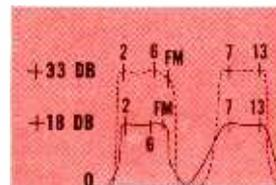
ACTUAL MEASURED CURVES PROVE A FLAT 18 OR 33 DB GAIN . . . HIGH BAND, LOW BAND, FM, TOD.
