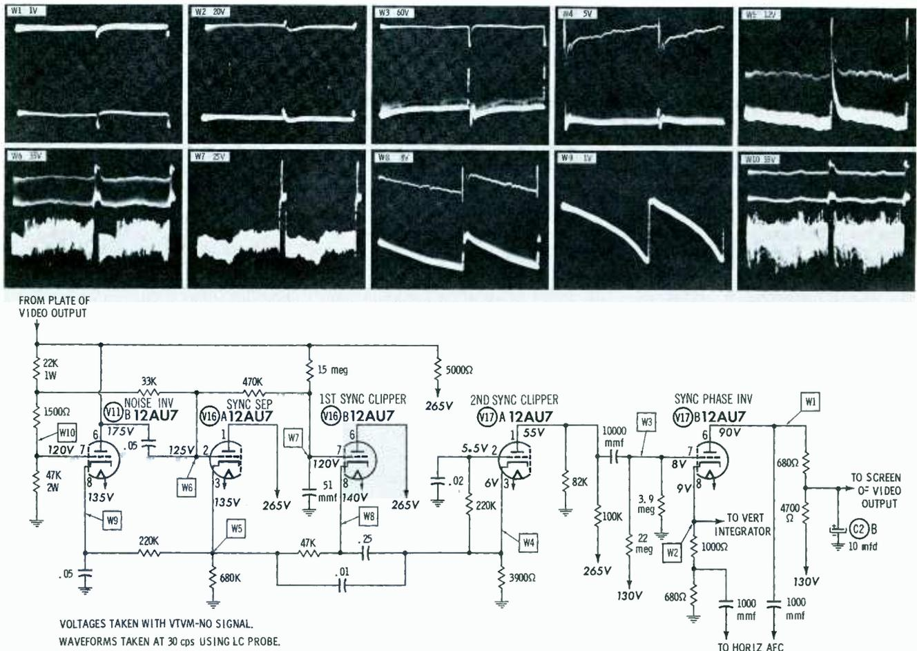
Fig. 1. Five-stage sync circuit in DuMont Chassis RA-170 poses unusually tough problem in trouble isolation.
