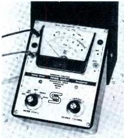
Fig. 3. This compact power supply provides DC voltages for variety of transistor devices.
