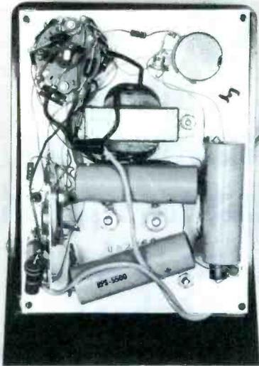
Fig. 5. Internal view Seco RPS-5 power unit.
