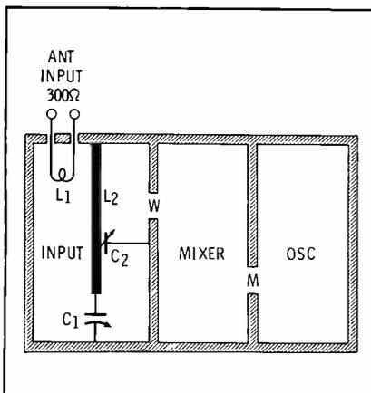
Fig. 4. Case configuration of typical tuner.
