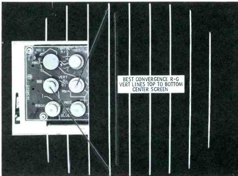
Use R-G vert lines top (Master Tilt) and R-G vert lines bottom (Master Amp) to converge the vertical red and green lines top to bottom center screen.
