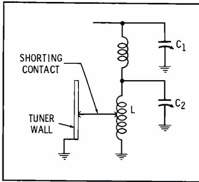
Fig. 3. Schematic of inductance-ring type.
