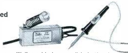
Temperature control of this new Weller soldering pencil is in the tip. Interchangeable tips give a choice of 500°F, 600°F, or 700°F controlled temperatures. Operates on 24 volts. Small, lightweight, highly efficient. Complete with 3/16" 700°F tip and 60 watt, 120 volt, 50/60 cycle power unit with stand for soldering pencil attached. Model W-TCP—\$26.00 list.
