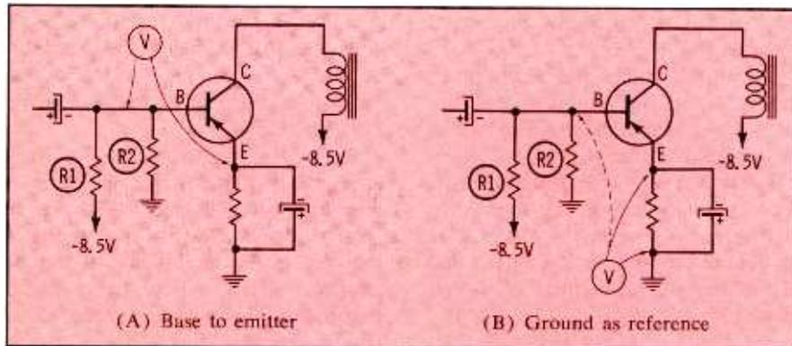
Fig. 1. Methods of measuring transistor bias.
