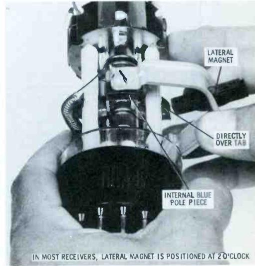
Poor convergence may result from improperly positioned elements; convergence yoke directly over pole pieces  $3\frac{7}{8}$ " from CRT base, purity ring  $\frac{5}{8}$ " rearward, and the lateral magnet over internal pole piece.
