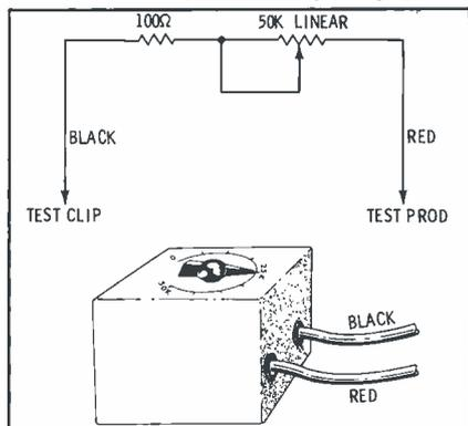
Fig. 3. "Bias-changer" will trace distortion.
