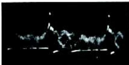
Fig. 3. Overdriving of video amplifier results in compressing white portion of video signal.
