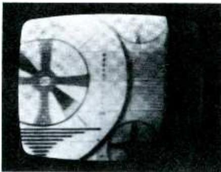
Bars may be sloping in either direction, depending on setting of horizontal hold control; at one setting, stable picture can be obtained, but phasing bar still appears in right side of picture. Adjusting L1 or L2 has little effect on symptom; defect on screen remains.
