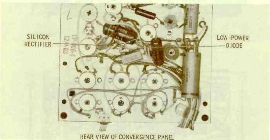
Convergence controls are located on a hand-wired assembly behind a removable speaker panel on the front of the receiver. The two latches that hold the panel may be reached from underneath.
