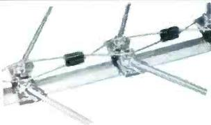
One-piece cross-over drive line assembly has no joints between adjacent driven elements. Eliminates loose connections, shorts, broken drive line sections. Polystyrene snap-lock spacers, with center 'air insulator' space.
