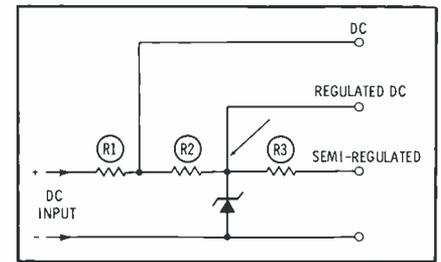
Fig. 3. Zener diode simple voltage regulator.
