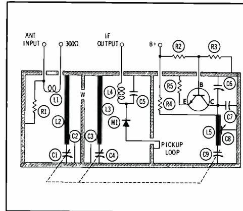
Fig. 5. Schematic of a typical UHF tuner. mixer, and an internally mounted transistor oscillator, the schematic will resemble that shown in Fig. 5. Other types of tuners are essentially similar—enough so that a single explanation should serve for most basic circuit functions.
