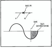
Fig. 2. SCR gate junction is control element.
