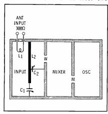
Fig. 4. Case configuration of typical tuner.
