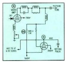
Fig. 1. Voltage drop across video-amplifier load resistor controls AGC tube conduction.
