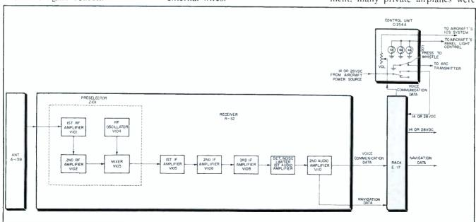
Fig. 1. Block diagram of a continuously tuned VHF-AM superheterodyne aircraft receiver.
