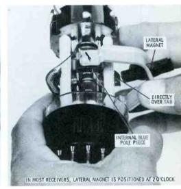
Poor convergence may result from improperly positioned elements; convergence yoke directly over pole pieces 3%" from CRT base, purity ring  $\frac{5}{8}$ " rearward, and the lateral magnet over internal pole piece.
