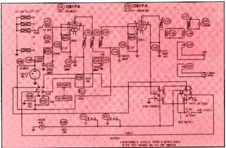
Fig. 3. Schematic of VHF transmitter. Separate modulator and power supply are required.
