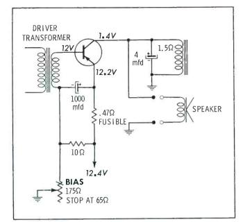
Installation of this radio requires the use of a 10-ohm rear-seat speaker to properly match the output impedance of the audio power transistor. Using a speaker with lower impedance would cause excessive current to be drawn by the output stage, thus burning out the bias control and/or the output transistor. The .47-ohm fusible resistor in the emitter circuit may also open.
