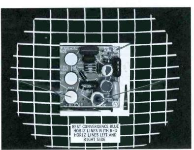
Use the blue horiz lines right (B-1) and blue horiz lines left (B-2) to converge blue horiz lines with red and green at the left and right center area.
