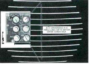
Use R-G horiz lines top (Diff Tilt) and R-G horiz lines bottom (Diff Amp) to converge red and green horiz lines top and bottom at the center of screen.
