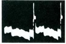
Fig. 5. W7 taken at V16B grid (18V p-p) consisted mostly of the vertical sync pulses.
