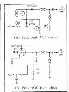
Fig. 10. Circuits in which AGC voltage is determined by peak level of video IF signal.
