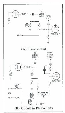
Fig. 8. Circuits producing supplemental AGC. grid of the sync separator resulted in excessive contrast along with disabling of the contrast control.
