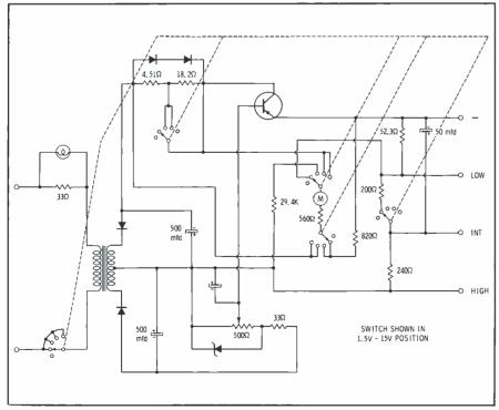
Fig. 4. Circuit diagram of the Seco Model RPS-5 shows how outputs are obtained and metered.
