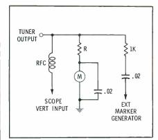
Fig. 6. Setup for sweep alignment of tuner.
