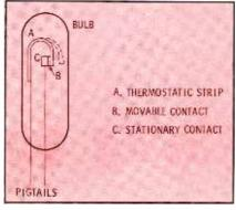
Fig. 2. A typical thermally-activated breaker.
