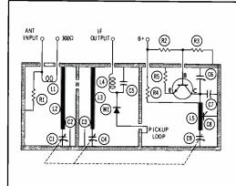
Fig. 5. Schematic of a typical UHF tuner. mixer, and an internally mounted transistor oscillator, the schematic will resemble that shown in Fig. 5. Other types of tuners are essentially similar—enough so that a single explanation should serve for most basic circuit functions.
