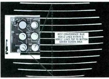
Use Blue horiz lines top (Blue Tilt) and Blue horiz lines bottom (Blue Amp) to converge blue horiz line with red and green lines at the center of the screen.
