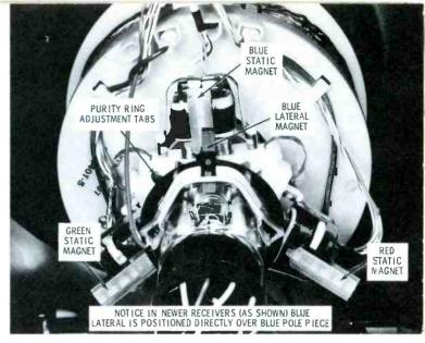
Black and white setup procedures, CRT degaussing, and purity checks should be performed previous to convergence. Use the red, green, and blue magnets and the lateral magnet for center dot convergence.
