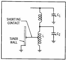
Fig. 3. Schematic of inductance-ring type. equivalent is shown in Fig. 1B. Both the inductor rod and the capacitor plates are silver plated to minimize losses by "skin effect."
