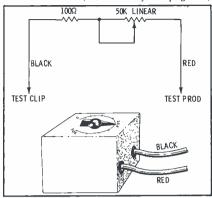
Fig. 3. "Bias-changer" will trace distortion.
