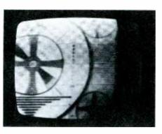
Bars may be sloping in either direction, depending on setting of horizontal hold control; at one setting, stable picture can be obtained, but phasing bar still appears in right side of picture. Adjusting L1 or L2 has little effect on symptom; defect on screen remains.
