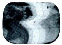
Fig. 9. Negative picture, poor sync resulting from gassy tubes in IF strip of TV receiver.
