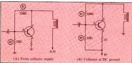
Fig. 2. Here is how bias is derived for base.
