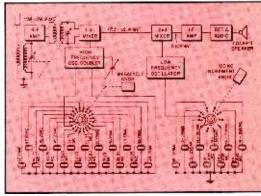
Fig. 2. Block diagram of a crystal-tuned VHF receiver in which frequency synthesis is used.
