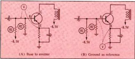
Fig. 1. Methods of measuring transistor bias.
