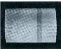
No raster when set is first turned on. Rotation of hold control produces dim raster; two pictures are obtained. Further adjustment of hold control gives sloping bars. Oscillator is running at approximately ½ normal frequency; loud whine can be heard. AFC is ineffective.
