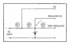
Fig. 3. Zener diode simple voltage regulator.
