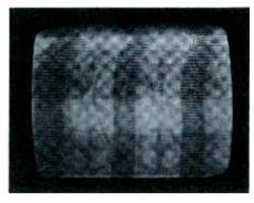
Three images—resembling Christmas-tree effect—can be seen, indicating extreme shift in oscillator frequency. AFC control straightens picture, but instability is still apparent. Drift over extended period requires continued readjustment of AFC.
