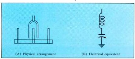
Fig. 1. Physical and electrical arrangement of a typical series-tuned UHF tank circuit.
