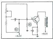
Fig. 4. Tester can substitute variable bias.
