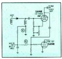
Fig. 4. Adding resistor in circuit helps prevent video overloading from strong signals.
