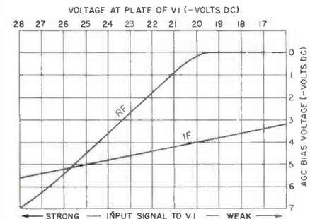
Fig. 3. Graph of the RF and IF Bias Voltages When an AGC Delay Circuit Is Employed.
