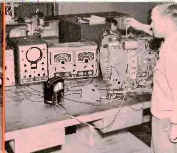
Actual alignment is performed using typical service type equipment to provide step-by-step instructions for alignment procedure.
