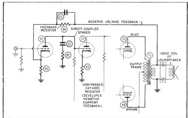
can give rise to many peculiar and disturbing forms of distortion. Loudspeakers have been blamed for a rattling or buzzing sound when the amplifier was actually at fault.
