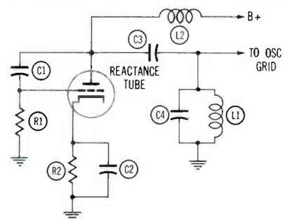
Fig. 3. Basic Circuit of a Reactance Tube.
