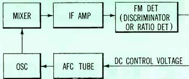
Fig. 1. Block Diagram of the Feedback Path for AFC.
