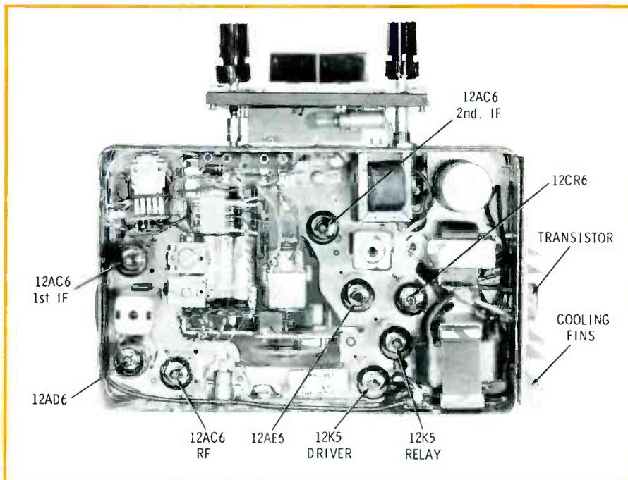
Fig. 4. Photograph Showing Placement of Tubes and Output Transistor in the Motorola Auto Radio. (Courtesy of Motorola, Inc.)
