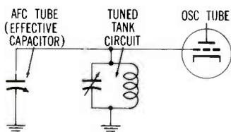
Fig. 2. Equivalent Circuit of an AFC Tube and a Tuned Tank Circuit.
