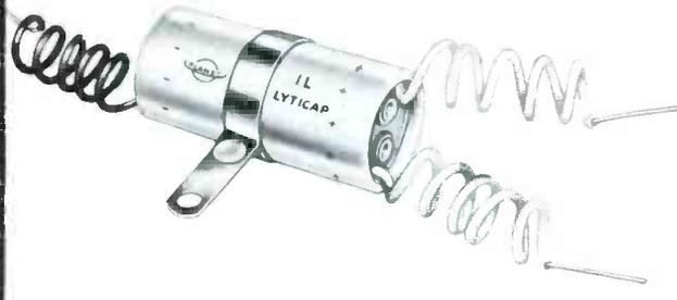
**NEW DUAL SECTION ELECTROLYTIC CAPACITORS HERMETICALLY SEALED IN ALUMINUM TUBES WITH COMPLETELY FLEXIBLE INSULATED LEADS.** By riveting the leads directly to the condenser end disc, Planet has eliminated the use of rigid terminal risers ordinarily used on this type construction. This allows Planet Type IL capacitors to fit into a smaller space and eliminates the possibility of lead breakage.
