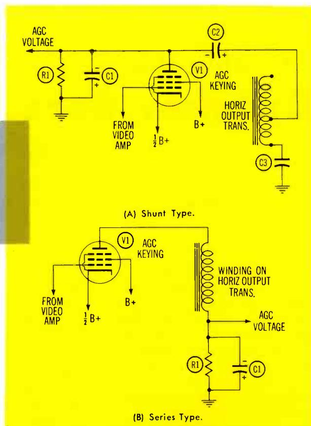
Fig. 1. Simplified Schematic Diagrams of Keyed AGC Systems.
