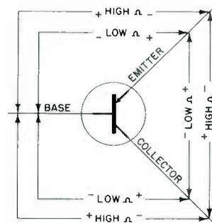
Fig. 5. Ohmmeter Connections for Checking the Power Transistor.
