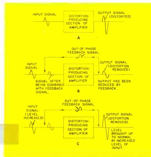
Fig. 1. The Effect of Negative Feedback on a Distorted Signal.
