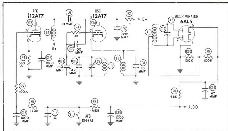
Fig. 5. AFC and Oscillator Circuits of the Harman-Kardon Model D200 Tuner.
