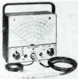
Just announced by Radio Corporation of America is the WV-98A Senior Voltmyst. This new meter measures DC voltages to 1,500 volts, AC voltages (rms and peak to peak) to 4,200 volts, and resistance to 1,000 megohms.
