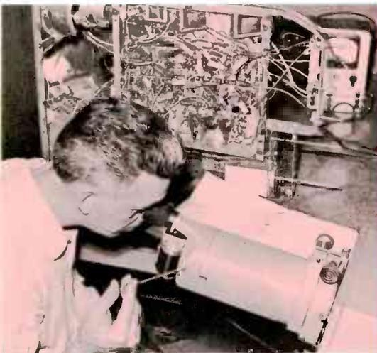
Oscilloscope camera records waveforms at selected reference points in a normally operating television receiver.
