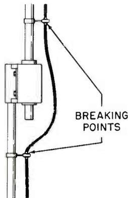
Fig. 2. Possible Breaking Points Near a Rotator.
