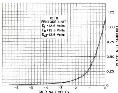
Fig. 3.  $E_{c1}$  Curve for a 12F8.
