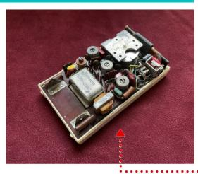
The TR-1 used many new miniature components ranging from Vokar 262kHz IF transformers, R/C tuning capacitor and a Jensen 3" speaker.
