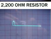
E-C GOOD SILICON TRANSISTOR SLIGHT ZENERING LEADS REVERSED
