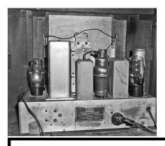
Once it was cleaned and assembled it does work, disengaging the clutch virtually "floats" the tuning dial. The Planetary Drive service notes state the disengaged position gives a 96 to 1 tuning ratio while the engaged is 16 to 1. All fine and good but pulling the knob to the disengaged position requires some effort and easily results in a disassembled knob and shaft in hand. Oh well, some things you just have to live with. *Fred Prohl, May 2018*
