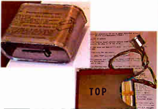
Above: Radiosonde Batteries. Evolved from acid fill in WWII through Korea to water fill in later years.
