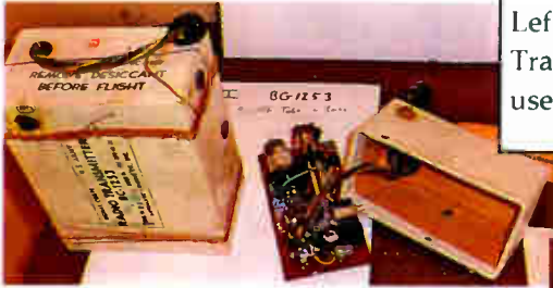
Right: A post war version of the radio transmitter, model AMT-2. The ACORN tube is replaced with a sub-miniature tube.
