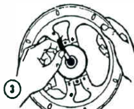
3 Clean pole piece of dirt and filings. Put scratch tape with sticky side out on shim stock, and push into gap. Hold shim steady and move speaker in rotary motion until all dirt and filings are removed. If air pressure or hand pump is available, it would help speed up operation, as it would blow out the dirt and most of the filings.
