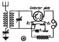
Receiver using the new Sodion tube.
