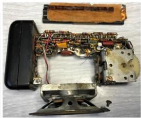
been the very first pocket-size, "highperformance" super-het transistor radio in the world. However, I imagine prohibitive costs killed it. For those who read the detailed engineering paper contained in PDF linked below, it appears that RCA designed this prototype to be a top-notch performer--unlike the TR-1 which was intended to meet a "price-point"...
