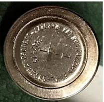
One of the audio transistors had been replaced at a later date with a (1954 date code) 2N35.
