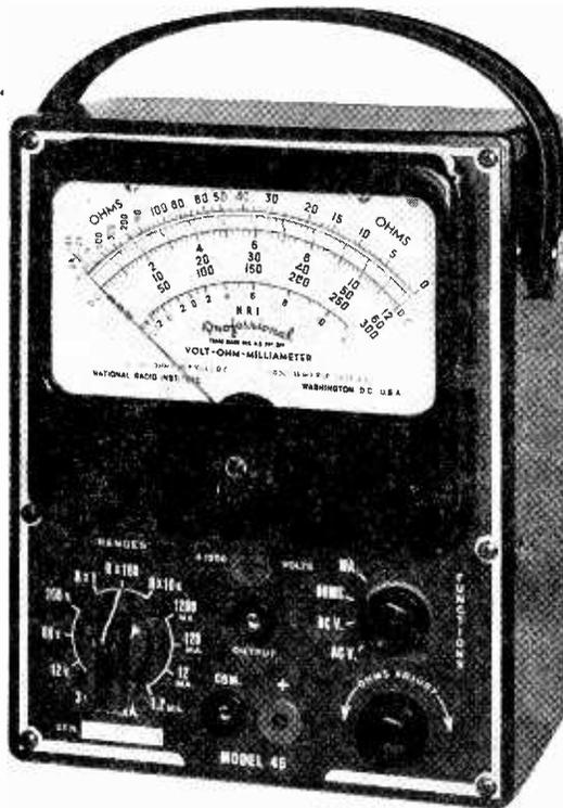
**5. Milliampere**s—Four ranges, up to 1200 ma. (1.2 amperes), measure plate and screen current in any receiver tube. 1200 ma. range, handy for measuring total current from television low-voltage supply.
