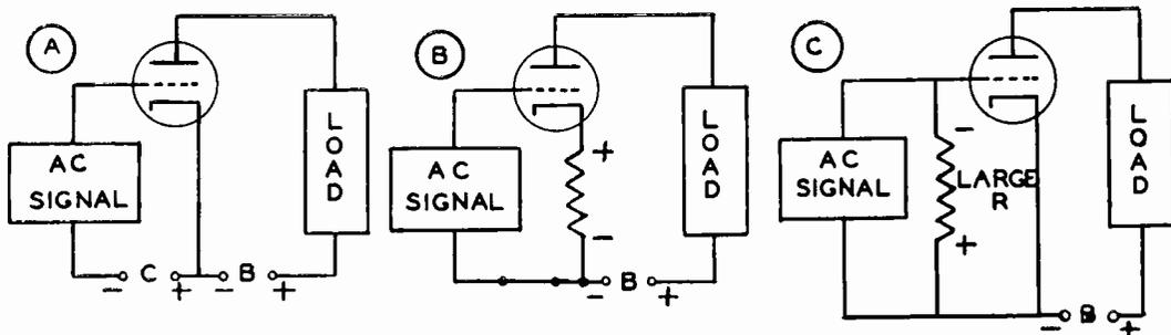
Fig. 2. The three bias methods most frequently used. Explanations are given in the text.
