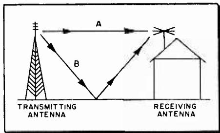
Fig. 2. The phase difference between the direct signal A, and the ground reflected signal B, produces a cancellation effect which varies with the height of the antenna.
