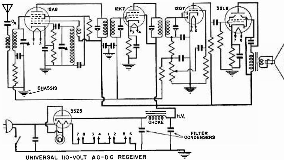
FIG. 4. Schematic of a typical AC-DC receiver.
