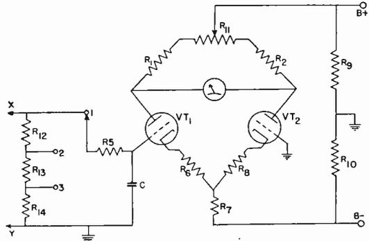
FIG. 2A. Basic, simplified circuit used in most bridge-type vacuum tube voltmeters, such as the NRI Model 11 VTVM.
