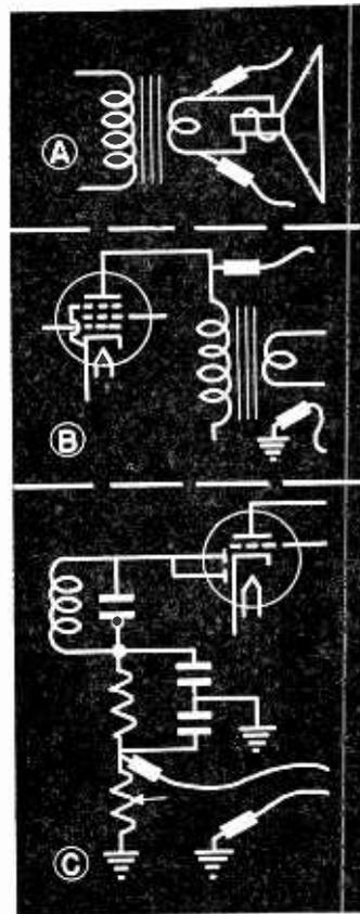
FIG. 5. Three ways of connecting a vacuum tube voltmeter for use as an output indicator in alignment: A, across the speaker voice coil; B, from the plate of the output tube to B—; C, across the diode load. Methods A and B use the instrument as an audio voltmeter. In method C, measure the avc voltage by connecting the instrument as a dc voltmeter, with the function switch set at —DC.
