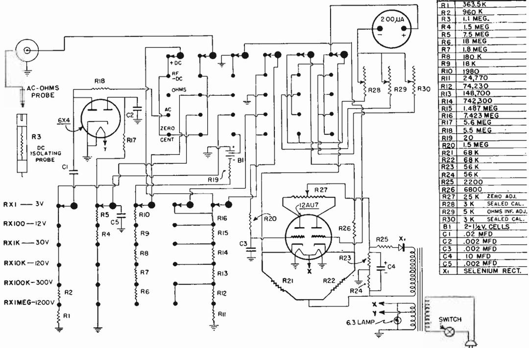
Fig. 2B. Actual schematic diagram of Model 11 NRI Professional Vacuum Tube Voltmeter.
