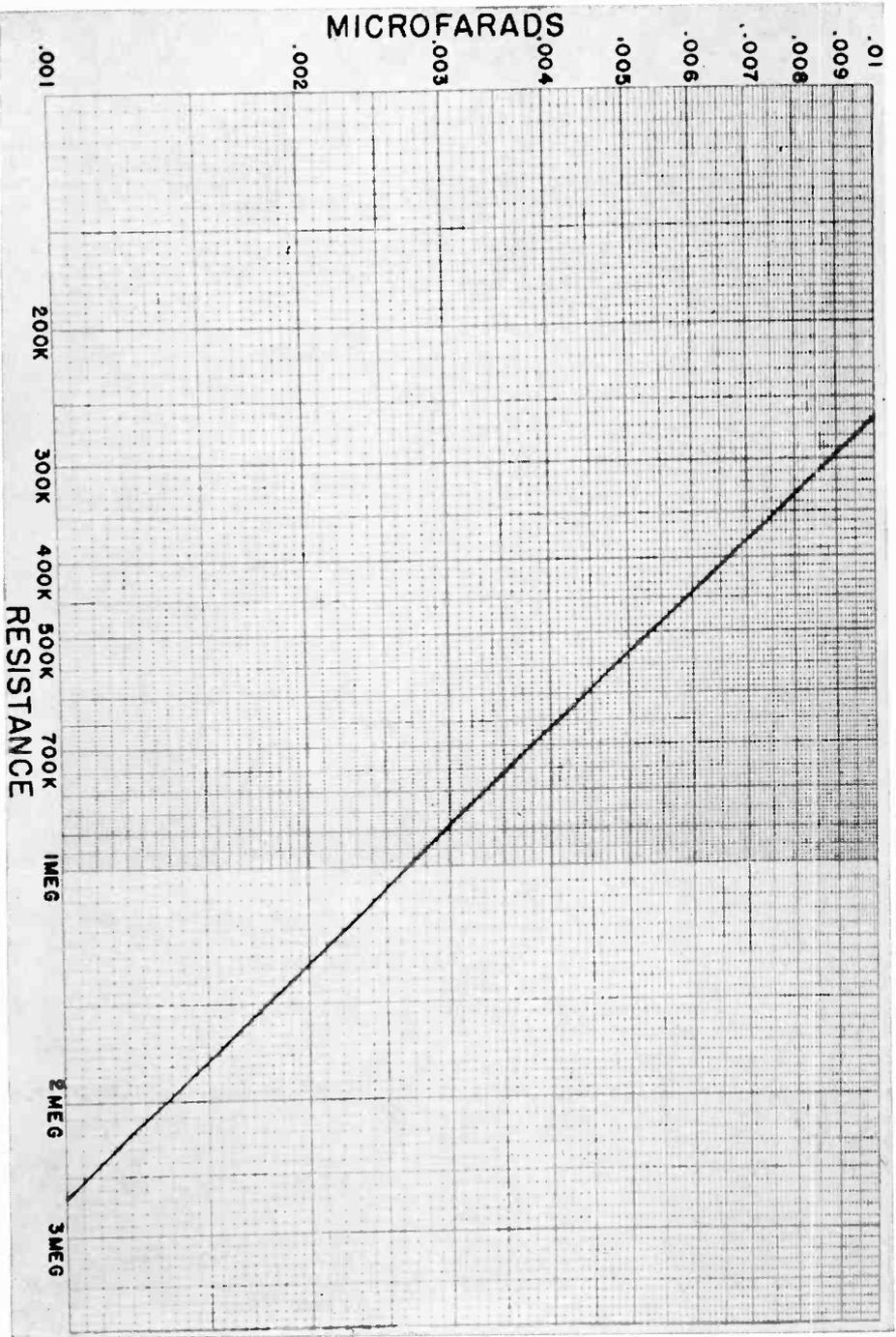
FIG. 6. This graph is used in obtaining approximate capacitance values with a VTVM.
