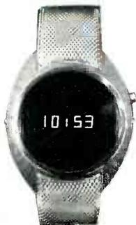
Push one button and the bright-red light-emitting-diode display against a dark background shows hours and minutes. The two dots between hours and minutes pulse every second.
