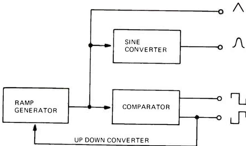
FIGURE 1. BLOCK DIAGRAM OF BASIC FUNCTION GENERATOR.
