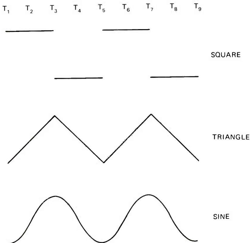
FIGURE 4. PULSE RELATIONSHIPS OF FUNCTION GENERATOR WAVEFORMS.
