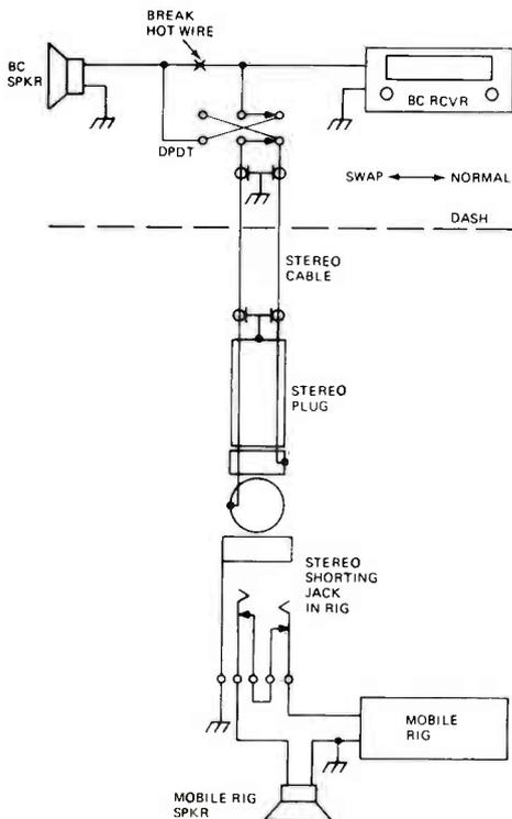
My GTX-2 did not have a separate phones or external speaker jack, but there was plenty of room on the rear apron to add one. Rather than put in the usual shorting type two-conductor jack, I installed the shorting stereo jack shown. If your rig already has a jack you can do the same thing quite simply since both types are the same size.
