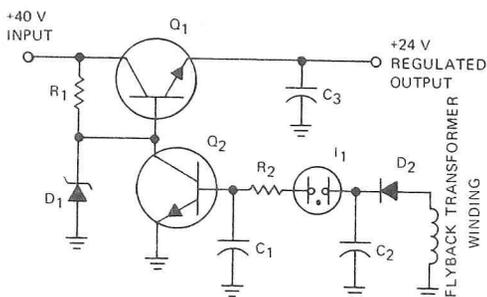
Fig. 2. The +24V supply, with automatic shut-down circuit.
