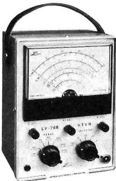
Performs all measurements with a single probe. Input Impedance of 11 megohms reduce loading effects. The AC range is usable to 4MHz. Large meter face for easy reading.
