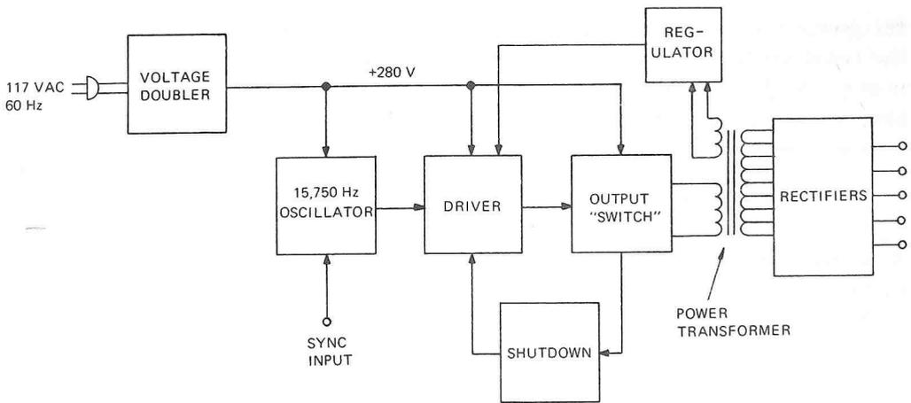
Fig. 3. Block diagram of power supply used in 1972 "QUASAR" by Motorola.
