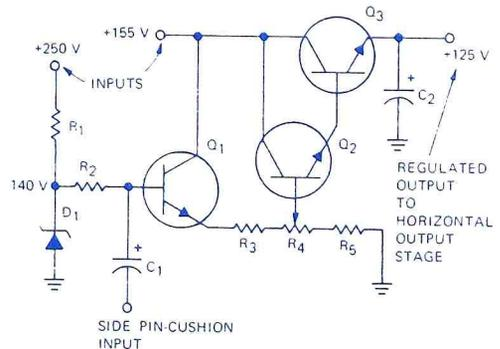
Fig. 1. Simplified diagram of +125V power supply used in Zenith solid-state color TV.
