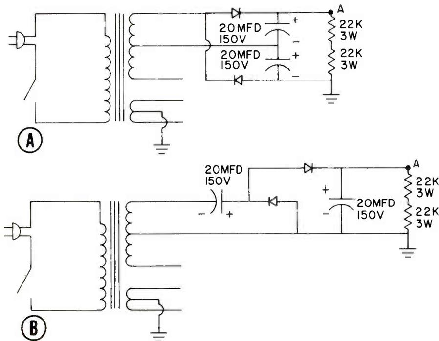
**Fig. 7. (A) Full-wave voltage doubler. (B) Half-wave voltage doubler.**
