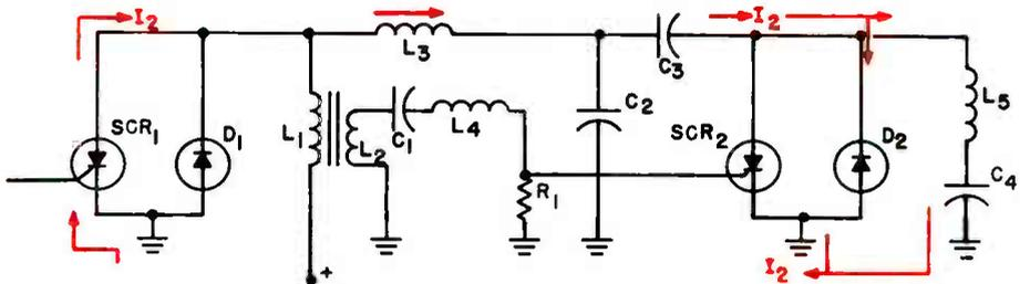
Fig. 8. Current flow during the interval  $T_4$  to  $T_5$  when  $SCR_1$  and  $D_2$  are conducting.
