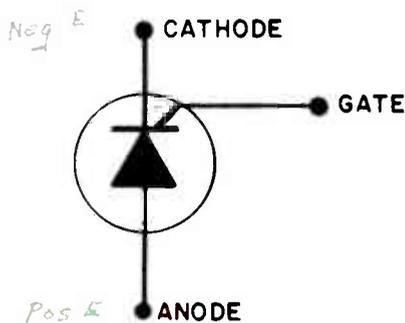
**Fig. 2. Schematic symbol of silicon controlled rectifier.**
