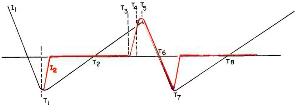
Fig. 4. The horizontal trace and retrace cycle.
