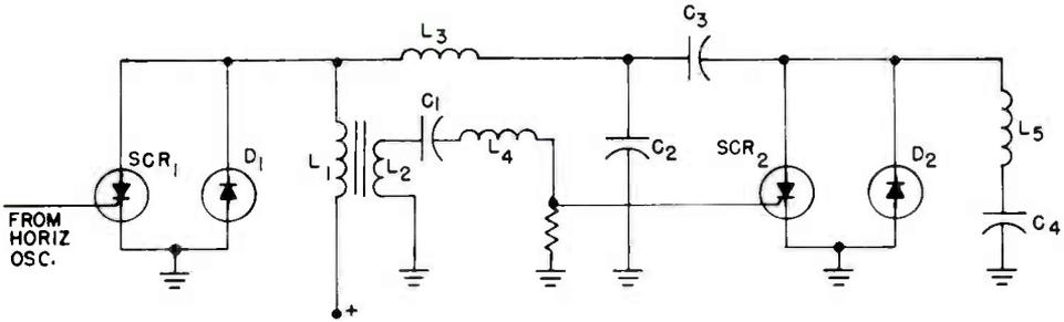
Fig. 3. Simplified schematic of horizontal sweep.
