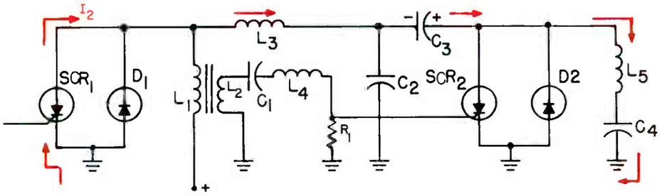
Fig. 9. Current flow during the interval  $T_5$  to  $T_6$ . Now only SCR<sub>1</sub> is conducting
