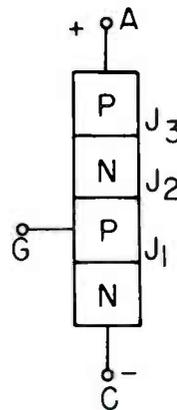
**Fig. 1. The SCR has four semiconductor regions and three junctions.**
