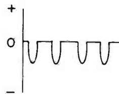
**Fig. 4. Full-wave capacitor charging current.**
