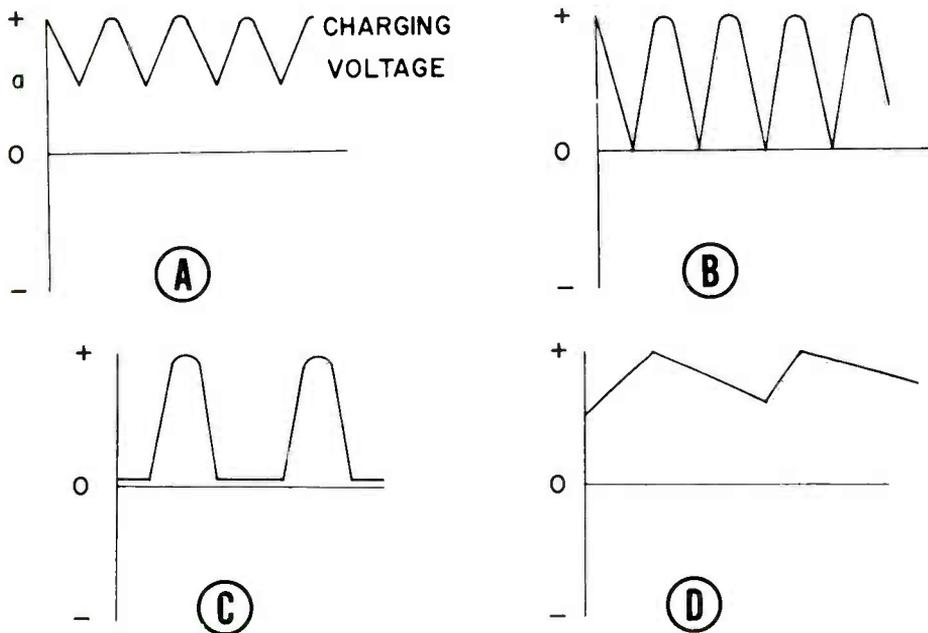
**Fig. 2. Power supply waveforms. (A) Full-wave ripple with capacitor and load. (B) Full-wave ripple without capacitor and load. (C) Half-wave ripple without capacitor and load. (D) Half-wave ripple with capacitor and load.**
