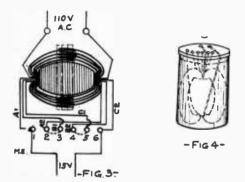
and another of wire until you get three separate layers of No. 16 wire of 50 turns each. Over this wrap several layers of cloth. These layers form the secondaries of which there are three separate coils.
