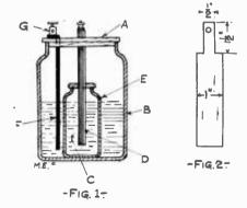
sulphuric acid. This style of interrupter has given the writer excellent results. Using 220 volts A. C., he was able to draw a spark an inch long from a coil whose secondary was composed of three quarters of a pound of No. 32 S.C.C. wire.
