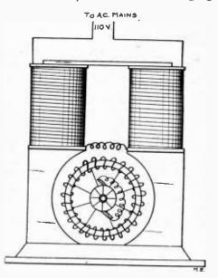
the position of the brushes, for in this way the speed of the motor and direction of rotation is controlled. At low speed this motor is very powerful, but as the speed increases the power decreases.
