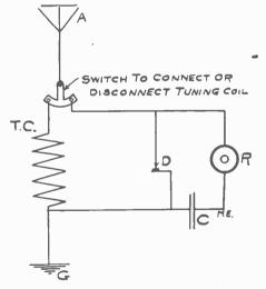
small case which contains the detector, and a condenser consisting of sheets; a tinfoil or copperfoil separated by some collodion, or better yet, "Healskin," and a switch. The cane does duty as both aerial and ground.
