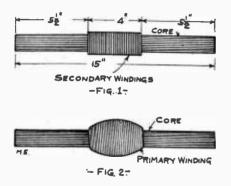
one layer of 50 turns of No. 16 D. C. C. wire over this. See Fig. 1. Then wrap a layer of cloth, which need not be shellacked because the whole transformer will be placed in oil, around this, then another of wire and cloth.
