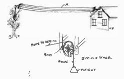
and put from one rafter to the other and then I took a bicycle rim with the ball bearings in it and put it on this rod and turned the nuts, so that the wheel could not move side-ways. The groove in the bicycle wheel is excellent to run the rope in and the rope will not wear out so quickly as with a smaller pulley.
