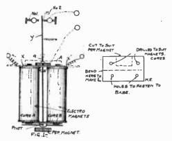
The instrument is now mounted on a base. This is done by fixing an angleshaped piece of brass at A. See Fig. 2. The contact posts, and springs are placed as in Fig. 1. Contact No. 2 is tipped with platinum.
