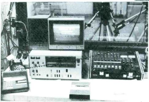
This locks the different sync from satellite, recorders, studio cameras, character generator, etc. all together on out going so there is no picture roll, etc. when changing. Randy Swingle said that this device was necessary because the cable system put their channel 51 on channel 4 which happens to be their main cable system control channel. Therefore, channel 51 has to maintain the exact standards of a full service station.
