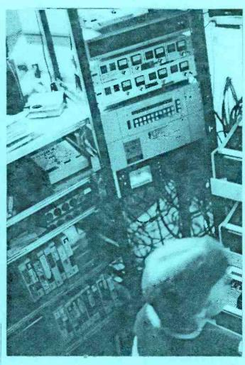
Upper left photo shows the rear view of equipment shown in the rack in right top photo, top equipment right, with all the dials, are two satellite receivers. Switcher personnel are in full time attendance from 6:30 am to 12:00 pm and switch program sources and stick in local commercials at pre designated spots, by using the 3 - ¾ inch tape decks shown far right in top right and bottom photo. All local production is on ¾ inch including commercials.
