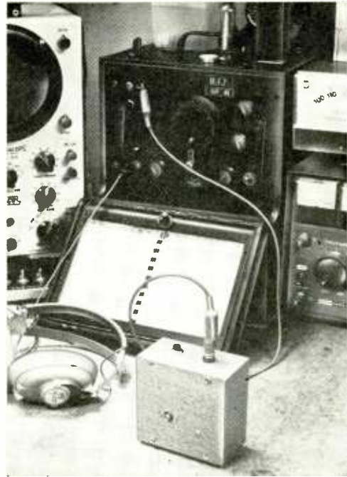
Where accurate frequency check points are a must, as when checking a BC-221 at 100-kc. points, the super calibrator speeds and eases the operation.
