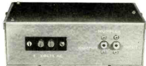
Fig. 2. In the self-contained unit, all connections are made on the rear panel. The name "Multiplex" refers to a function that no longer applies.
