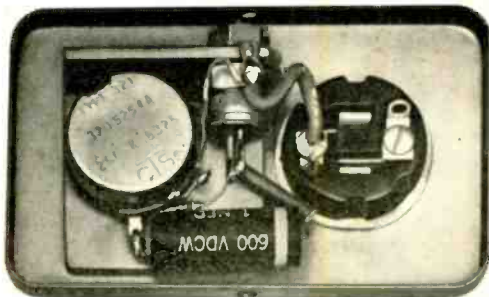
The heat sink on the inside of the case and the dial plate on the outside are held in place by a rivet (hidden by the capacitor) and the potentiometer nut.
