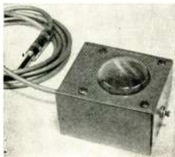
Low-impedance pickup, made from small 45-ohm speaker, uses plastic "cap" for mechanical coupling. The switch mounts on top of case.
