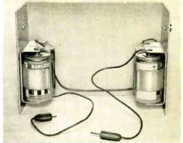
These two photos show how the power supply or shoulder pack is mated. In the photo above, the D cells—mounted in battery clips—are bolted to the two end plates of the shoulder pack wraparound. The batteries are wired in series and, for convenience, the positive and negative leads end in color-coded insulated tip plugs. The power supply sub-chassis and capacitor C2 must be positioned so that the batteries will slip into the small space available.
