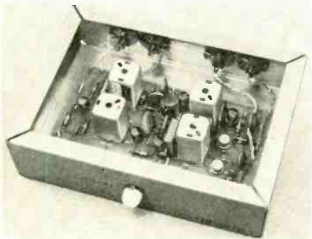
Fig. 8. Twisted leads are used as self-shielded conductors. The lead acting as a shield is connected only to the ground foil on the board. A bare wire connects the ground side of the jacks to a single ground point on the circuit board.
