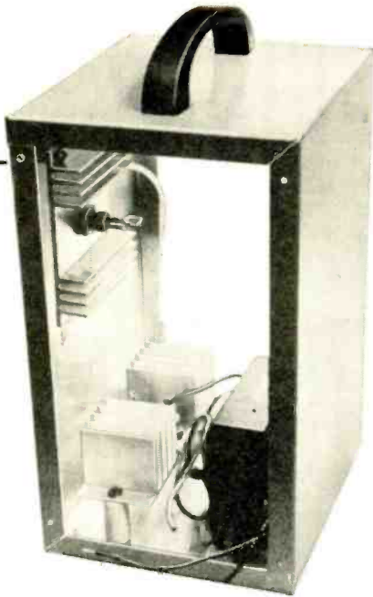
Transformer is bolted to bottom of box. Rectifier heat sink is at left and heat sink for SCR1 is attached to the side.
