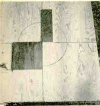
Centers for port holes are marked out using two pattern boards. Dimensions of the boards are given in the Bill of Materials. How they are used is described below.
