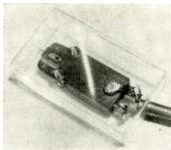
High-impedance pickup at right consists of phono cartridge mounted in plastic case. Above, unit is shown detecting vibration in fan base.
